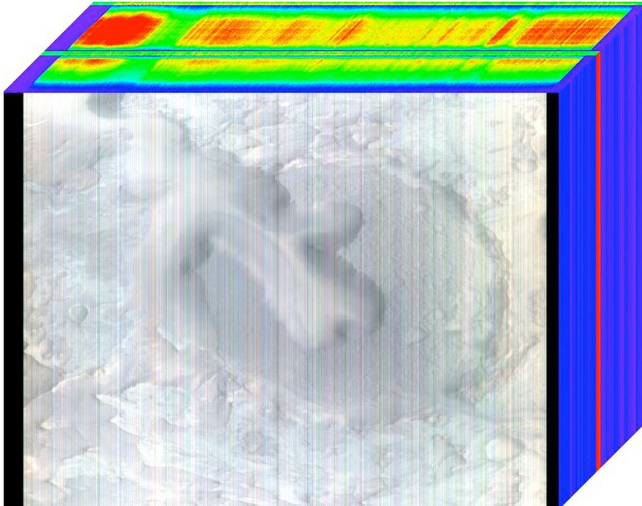
A multiband image of raw data formatted from the telemetry stream; assembled from multiple frames
