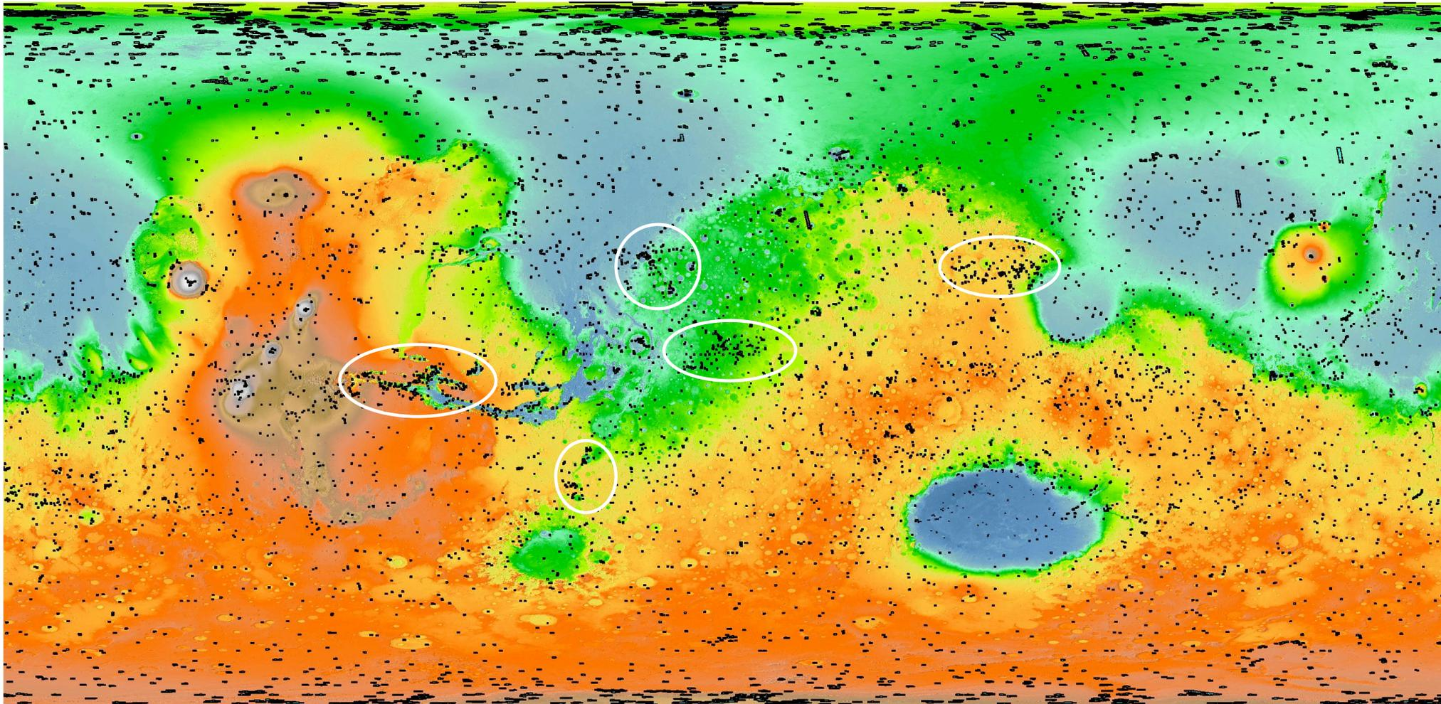
9,514 targeted observations were taken during MRO's PSP. 6,674 were at full resolution (18 m/pixel) and 2,840 were at half resolution (36 m/pixel). The highest concentrations are at phyllosilicate, sulfate, and chloride deposits discovered by OMEGA and THEMIS.
