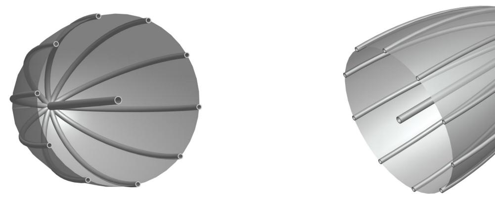
**THE INFLATABLE APPROACH: The entire envelope will be fabricated on** Earth as a single piece and flexible fiber tube joints to allow packing. Upon landing on the Mars' surface the envelope would be pressurized and epoxy resins rapidly pumped into the tubes to solidify and thus forming a rigid structure and then the vacuum pump takes over.
