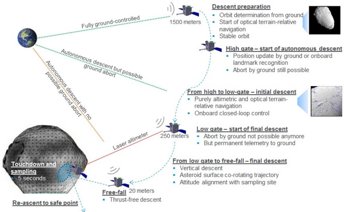
Figure 5.6: MarcoPolo-R asteroid descent and sampling sequence (altitudes and exact procedures vary depending on the design option)
