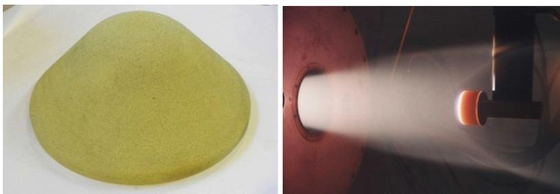
Figure 5.25: Heat shield material prototype (left) and sample plasma tests in DLR (right)
