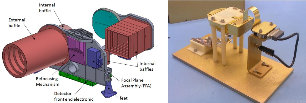
**Figure 4.1:** CAD view of the proposed MaNAC design (left). Test setup of the detector used for SimbioSys on BepiColombo, which is the current baseline detector for MaNAC.
