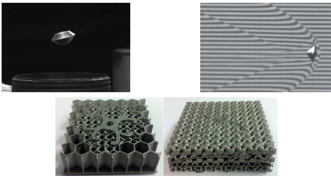
Figure 5.26: ERC stability tests in the subsonic regime at DLR (top-left) and the super/transonic regime at ISL (top-right); Titanium foam crushable material by Magna Parva (bottom left and right).
