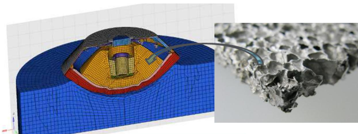
**Figure 5.8:** Re-entry capsule numerical impact analysis (left), sample of impact absorbing material (right).
