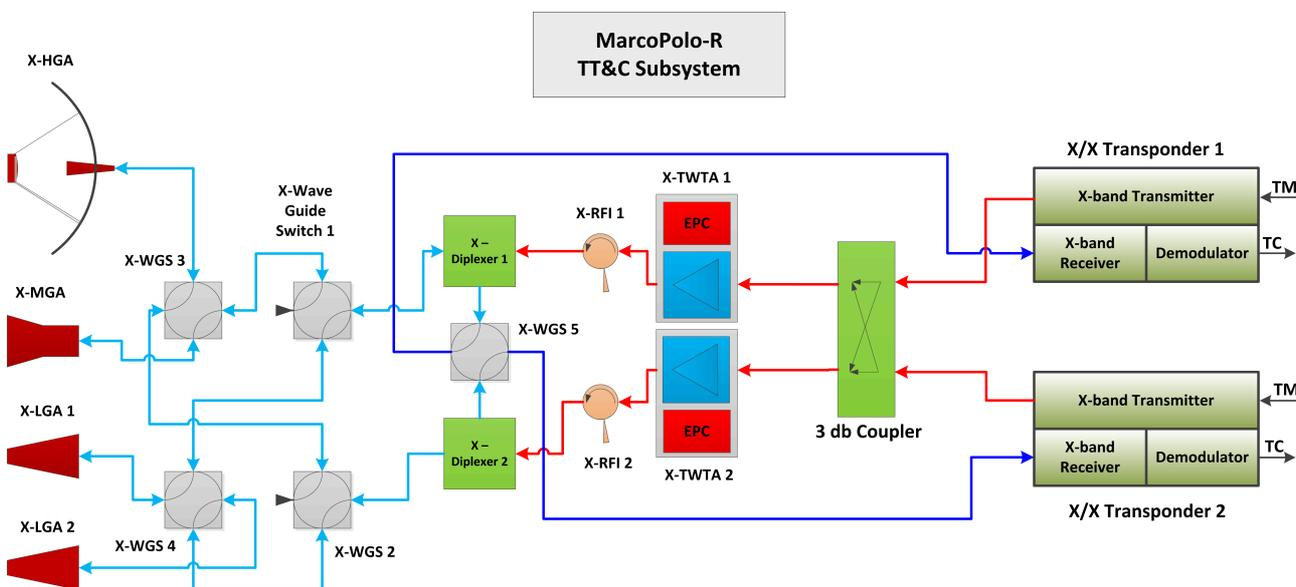
Figure 4.9: Design of the TT&C subsystem (X/X band link) onboard MarcoPolo-R which can be used for RSE in its basic configuration.
