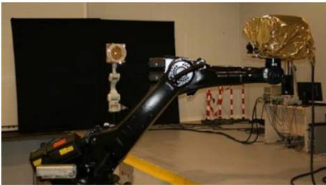
**Figure 5.19:** GNC Test Bench by GMV.
