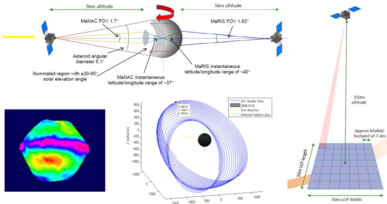
Figure 5.4: Observation strategy during the GCP (top-left), LCP (right), RSP (bottom-centre). Simulation of 2008 EV5 as seen by MaNAC during GCP (bottom-left).
