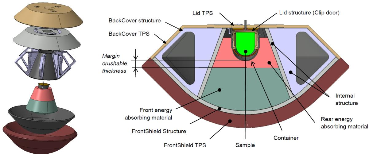
Figure 5.14: Option A - design of the ERC.
