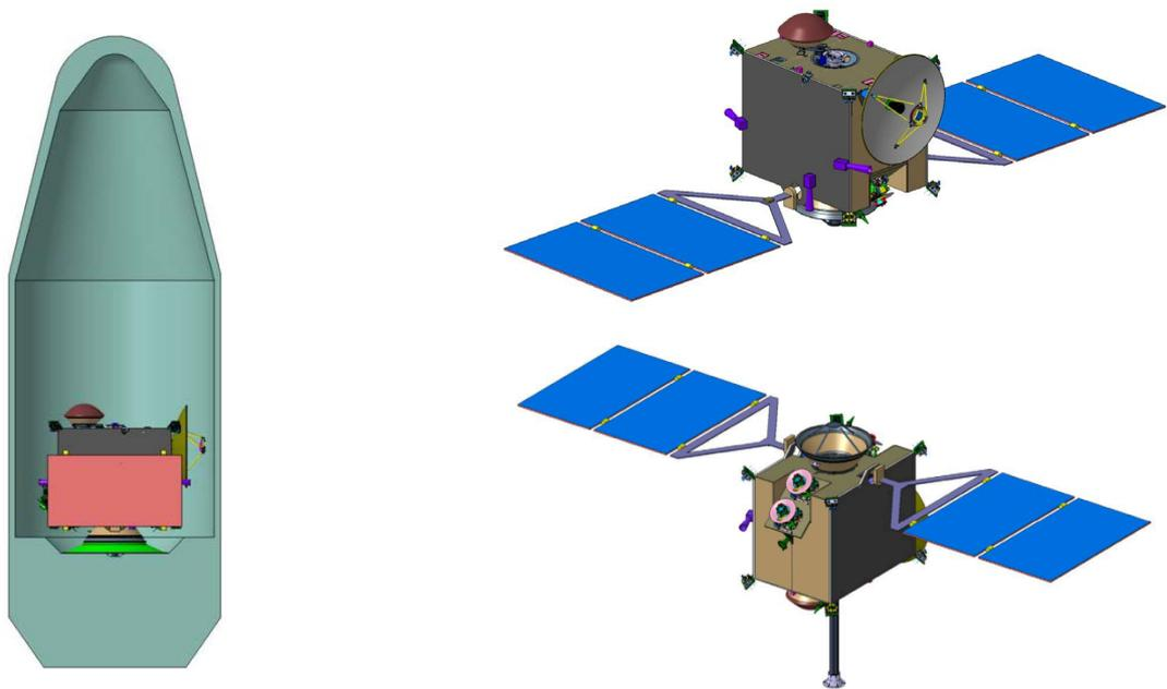
Figure 5.10: Option A – Spacecraft in launcher fairing (left), during cruise (top-right), in touchdown configuration (bottom-right)
