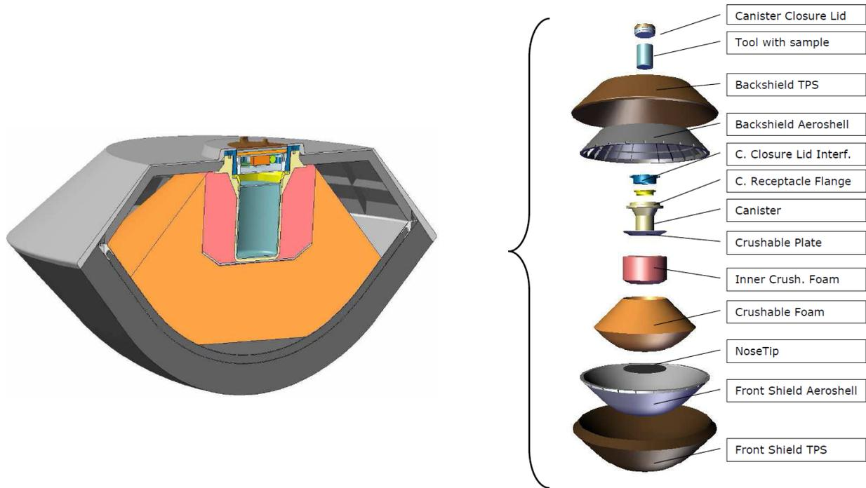
Figure 5.18: Option B - ERC Design (left) and sample container accommodation (right).
