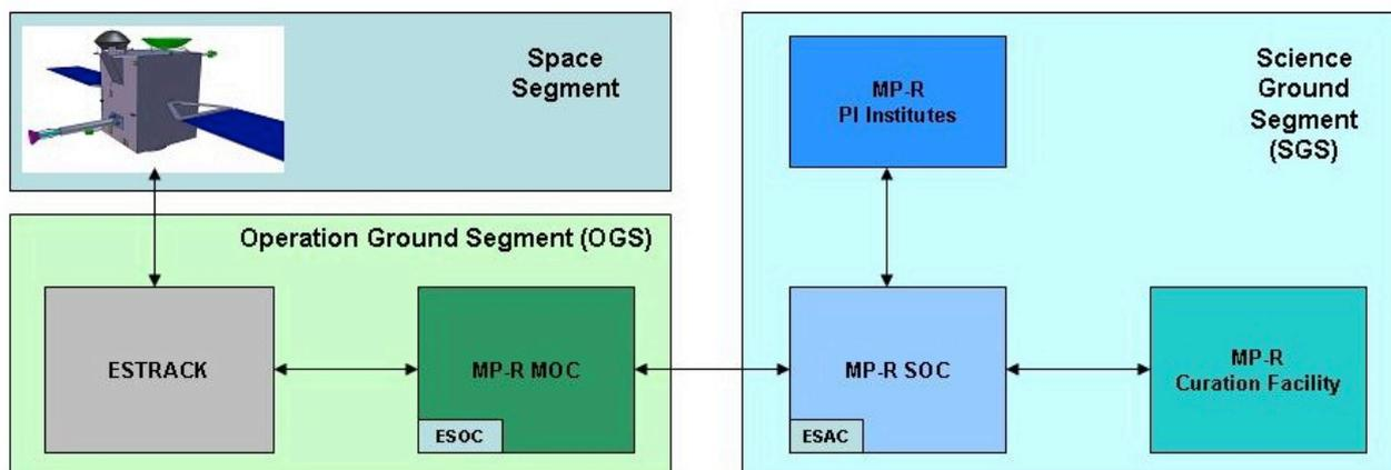
**Figure 6.1:** MP-R ground segment architecture, showing the SOC interface with the MOC for uplink and downlink support to the MP-R spacecraft, and the SOC interface with the PI Institutes and Curation Facility.
