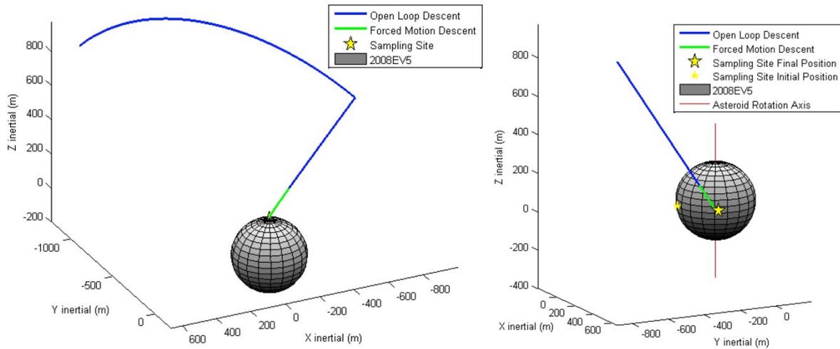
Figure 5.12: Option A GNC approach Examples (left: polar sampling, right: equatorial sampling)
