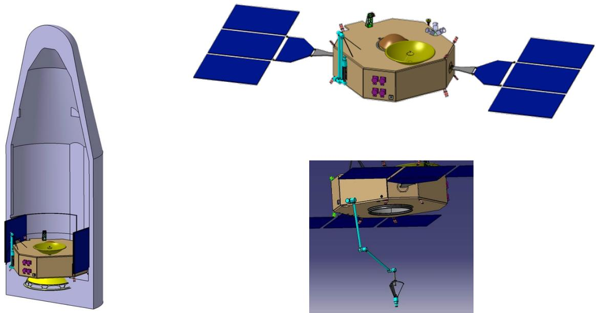
Figure 5.15: Option B - Spacecraft in launcher fairing (left), during cruise (top right), in touchdown configuration (bottom right).
