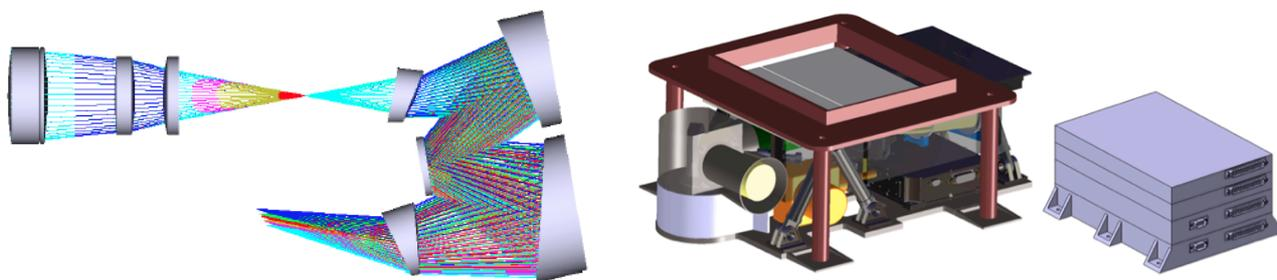
Figure 4.5: Optical head (left) and mechanical design (right) of MaRIS.
