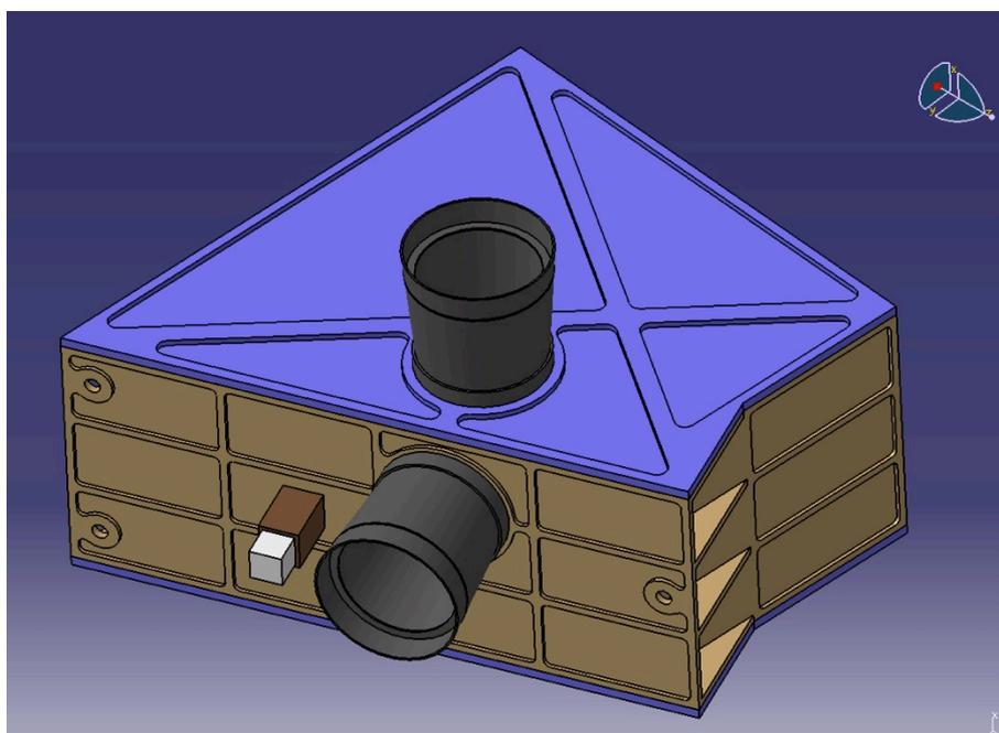
**Figure 4.8:** External view of the THERMAP instrument, showing the main box and the two external baffles toward the asteroid and deep space (for calibration purposes).
