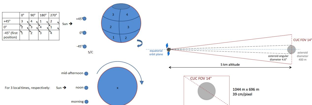
Figure 4.4: Viewing geometry of the CUC when used as wide-angle camera.
