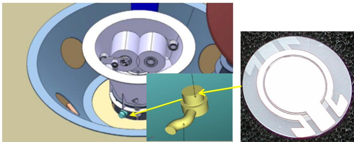
**Figure 4.10:** Left: Location of the VISTA2 sensor mounting (insert) on the brush-wheel sampling tool viewed from below. Right: Photo of the GaPO<sub>4</sub> crystal located on top of the sensor mounting (IMM-CNR).
