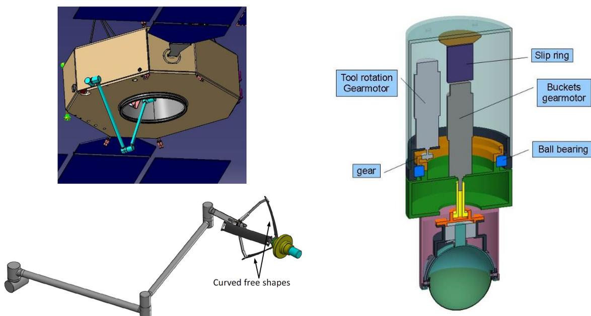
**Figure 5.17:** Option B – SATCS: transfer of the sample container (upper left), touch and go arm (bottom-left), sampling tool (right)
