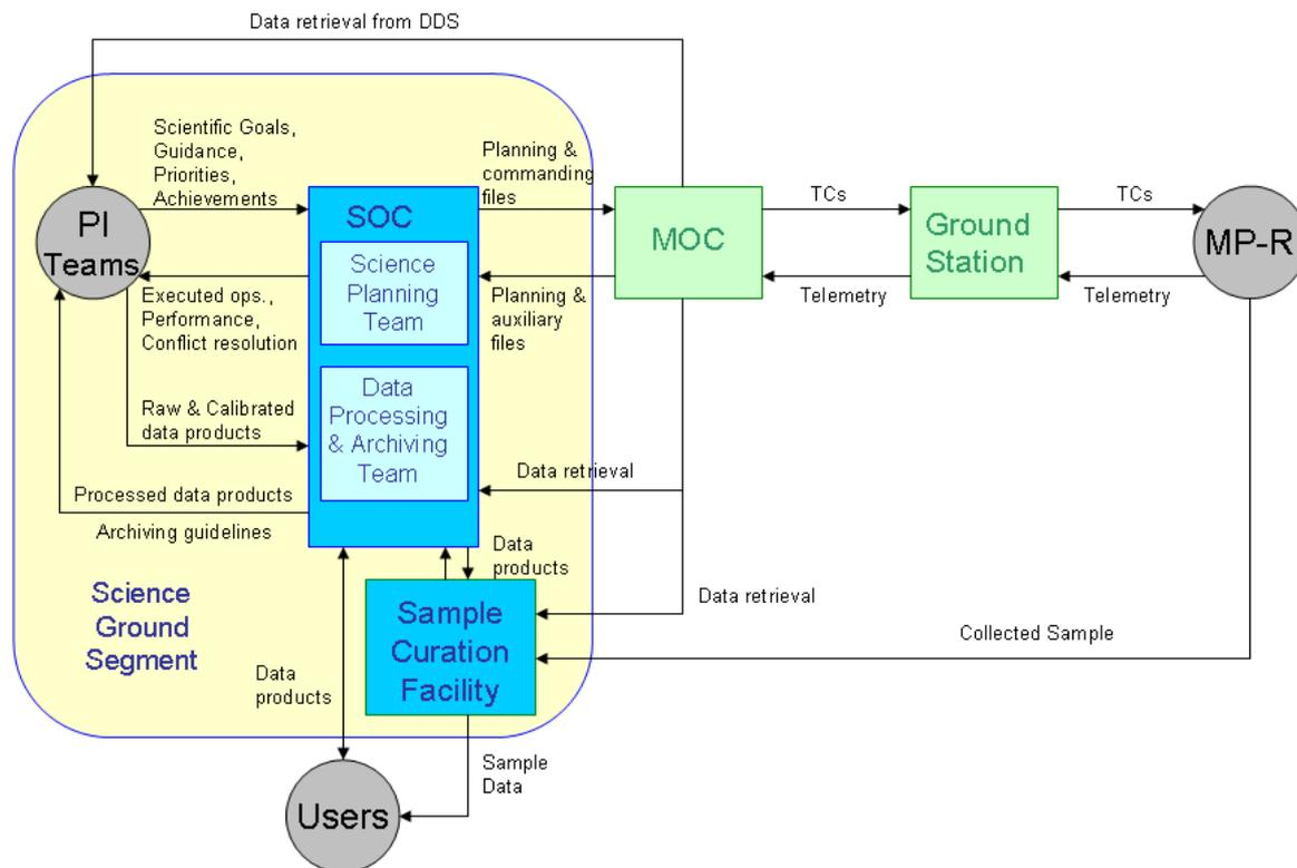
**Figure 6.4:** Data flow to and from the MP-R Science Ground Segment (SGS). Science Operations are developed and implemented within the SGS that encompasses ESA functionalities (SOC, for both uplink and downlink including Science Planning and Data Handling and Archiving Teams) and non-ESA science operations activities (PI teams and Sample Curation Facility Team).
