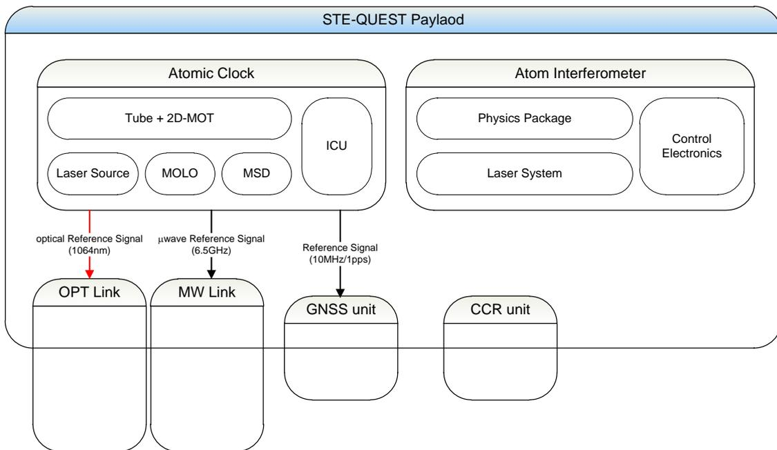
**Figure 3: Block Diagram of the STE-QUEST Payload**
