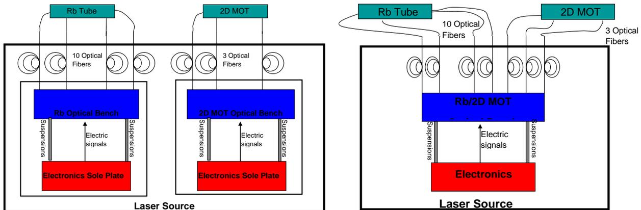
**Figure 7: Preliminary Design of STE-QUEST Atomic Clock Laser Source: baseline design based on Pharo heritage (left) and alternative design based on telecom fibre lasers (right)**
