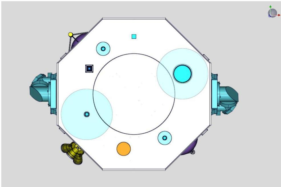
**Figure 23: Placement of the two LCT heads on the CDF model of STE-QUEST. Placement on two different, opposite panels ensures the common view capabilities.**
