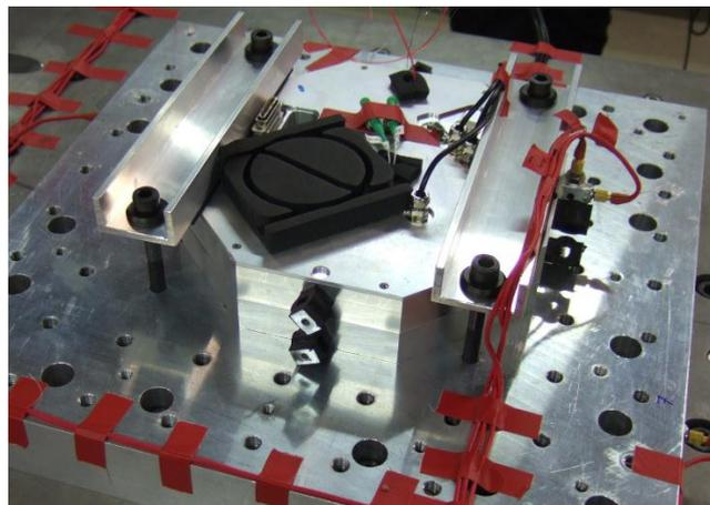
**Figure 12: Menlo Systems femtosecond frequency comb for TEXUS experiment**
