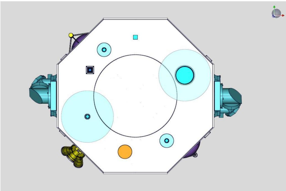
**Figure 21: Antennae placement from the CDF study (light green shades denote minimum obstruction-free zones) .**
