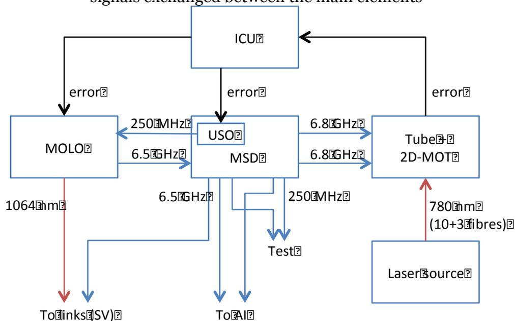
Figure 4: Clock Subsystem Block Diagram
