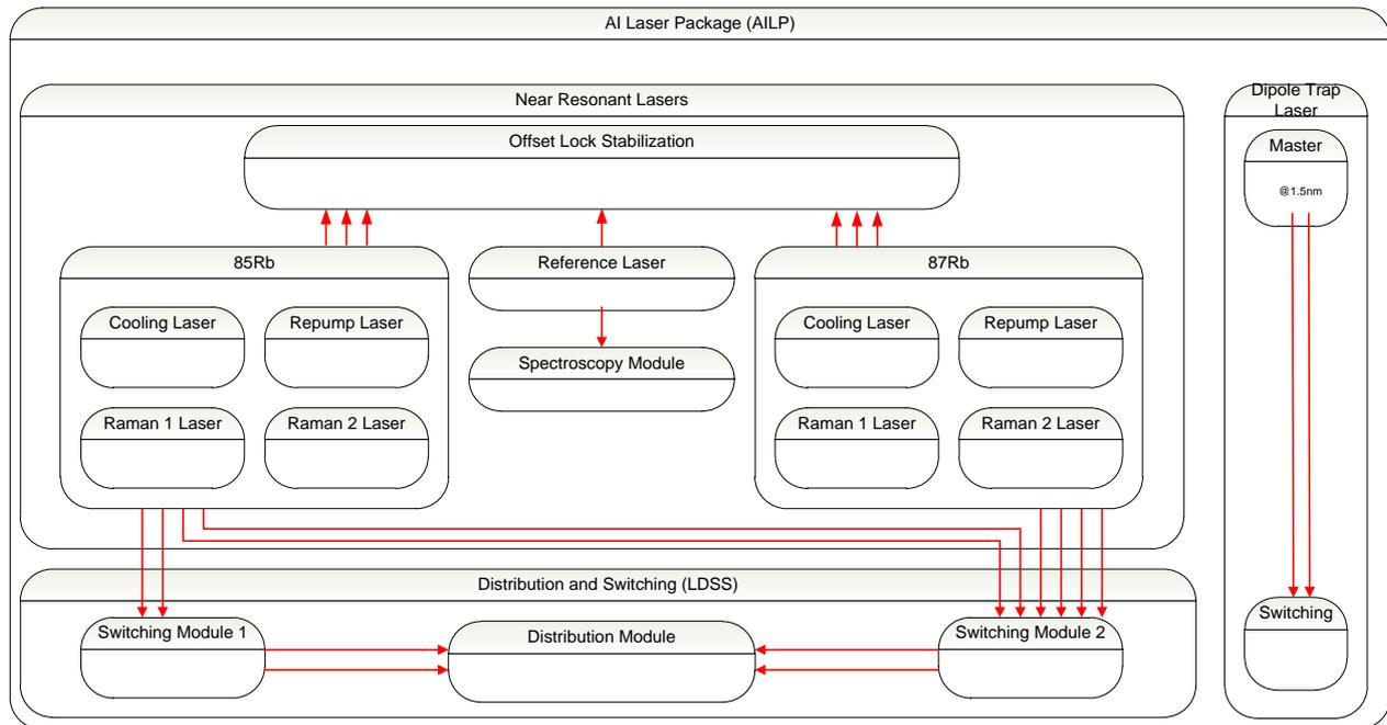
**Figure 18: Example Block Diagram of AI Laser Package (redundant lasers are no shown)**
