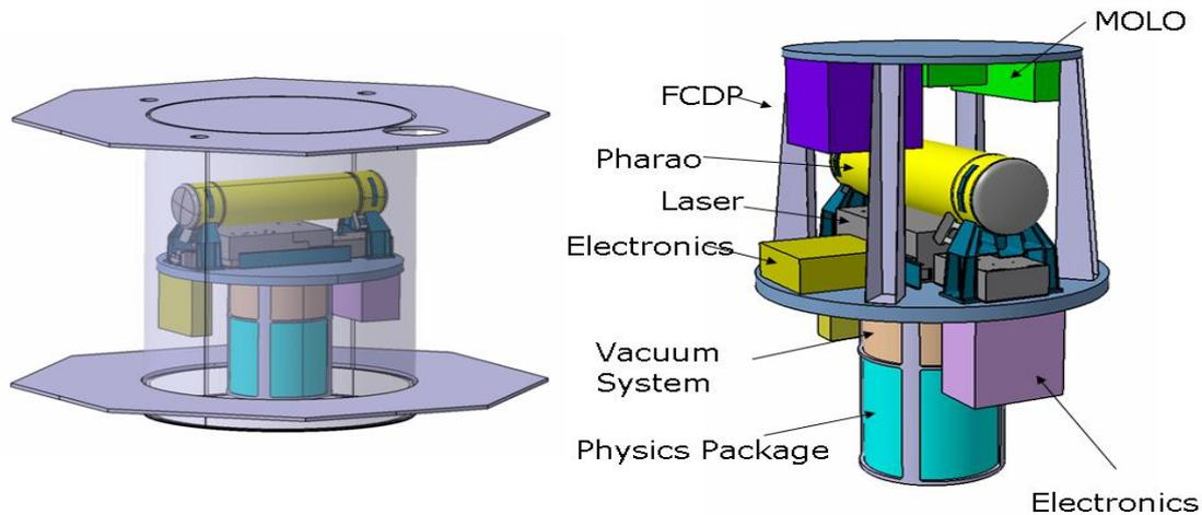
**Figure 2: STE-QUEST model payload accommodation (as defined during the CDF study). Left the payload compartment with the clock subsystems in the top part and the atom interferometer systems in the lower part. Right the accommodation of the compartment in the main spacecraft structure.**
