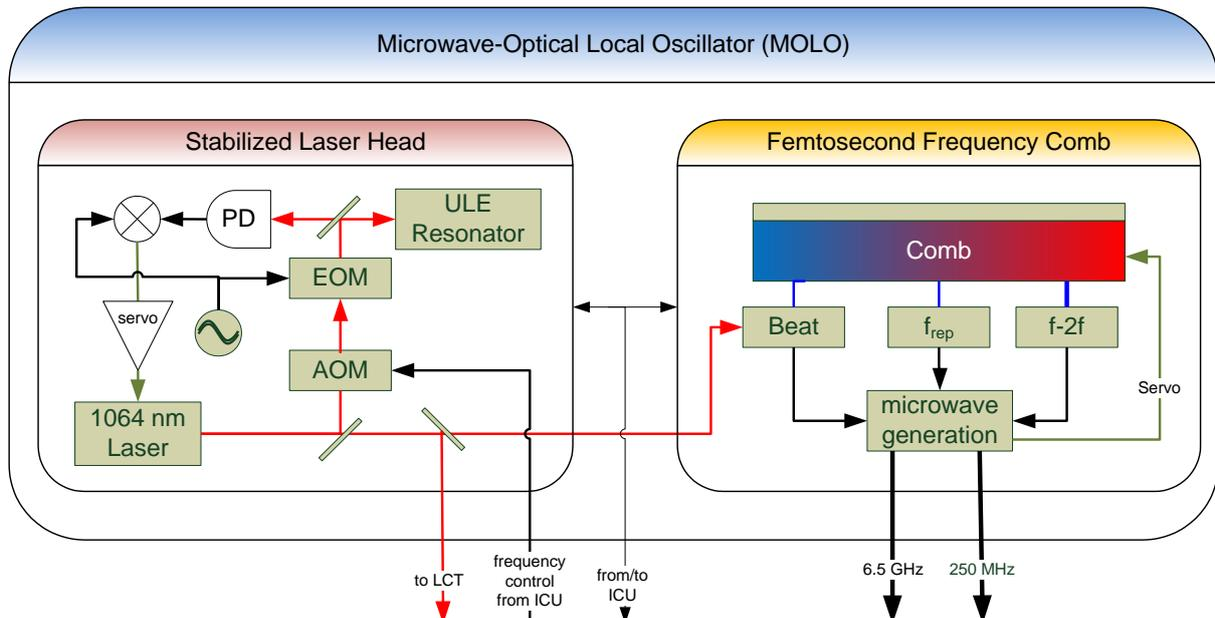
**Figure 8: Block Diagram of MOLO**
