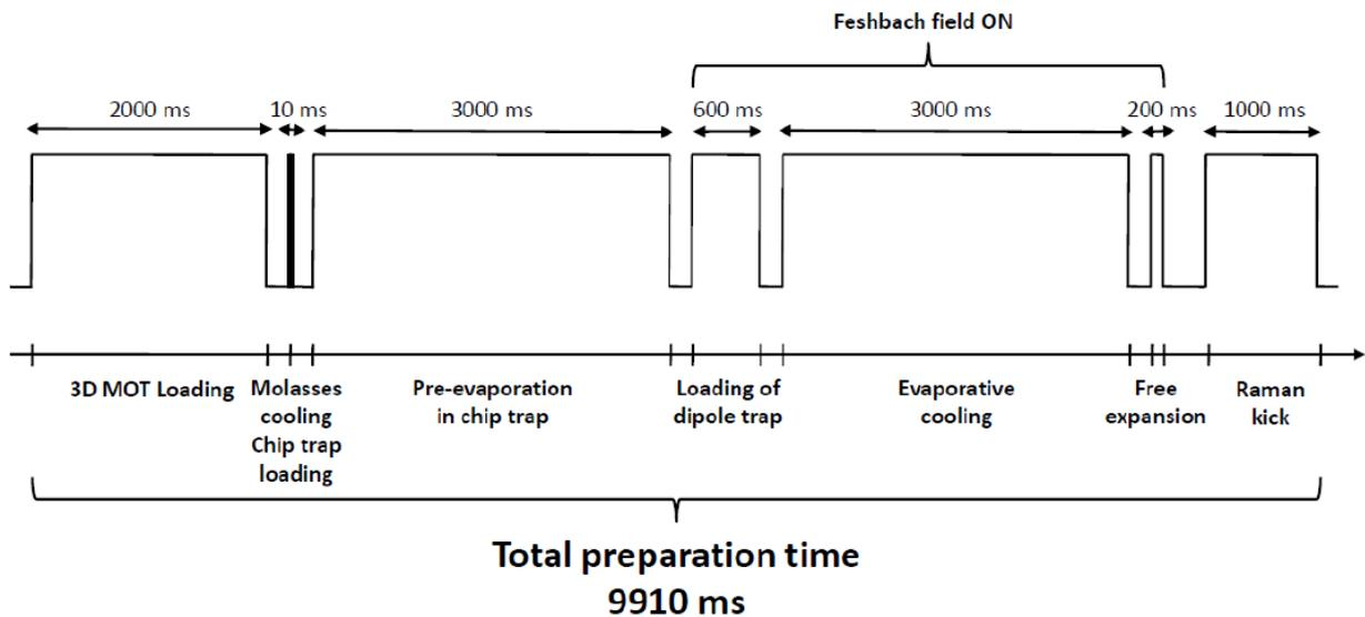
**Figure 15: Time sequence for trapping and cooling the atom clouds. The 10 seconds expansion time and the detection sequence is not shown.**
