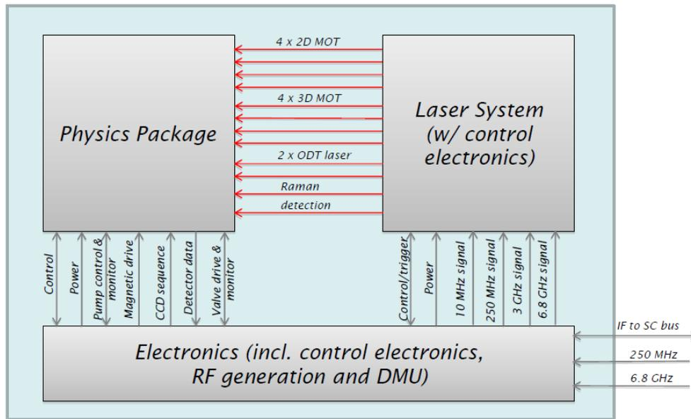
**Figure 14: Atom Interferometer Top-Level Block Diagram**
