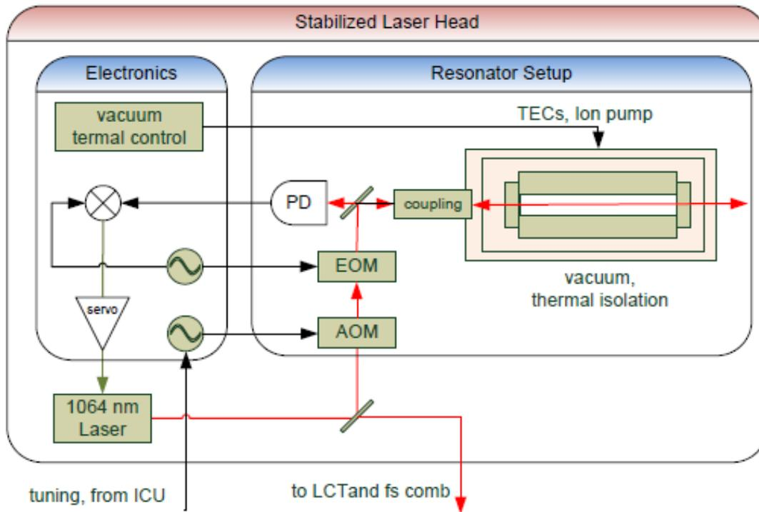
**Figure 9: Block Diagram of MOLO Stabilised Laser Head**
