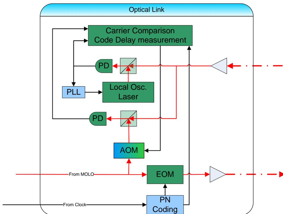
**Figure 22: Example Layout for the optical link (space segment)**
