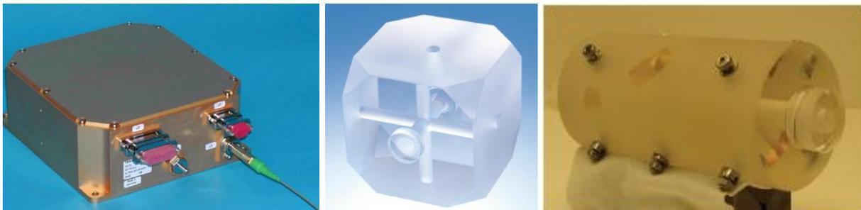
**Figure 10: Elements of MOLO Stabilised Laser Head: Tesat Laser Head at 1064nm (left), NPL squeezed-cube optical cavity (centre), PTB multi-point supported cylindrical cavity (right)**
