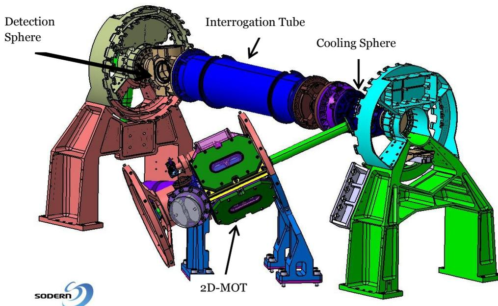
**Figure 5: Current baseline design of Pharao NG (Rubidium Tube) shown without mu-metal shields.**
