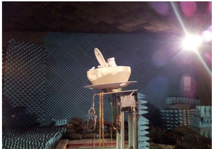
Figure 4-6: ACES MWL ground terminal under test in compensated compact range facility. The STE-QUEST ground terminals will be based on the ACES technology.
