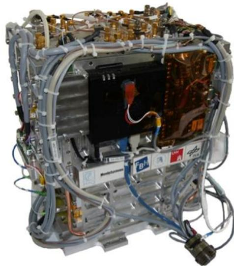
**Figure 4-9:** Er:fibre based comb delivered for the TEXUS sounding rocket test (Menlo Systems).
