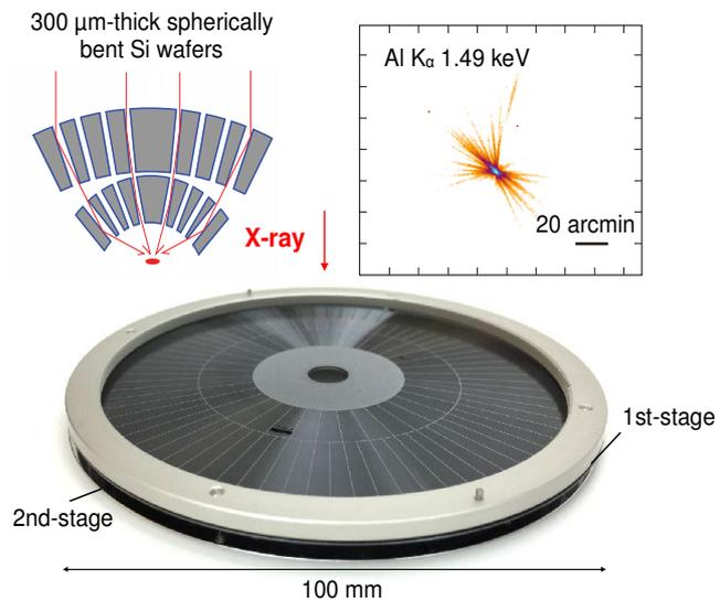
**Figure 1: Ultra-light-weight X-ray telescope.**
