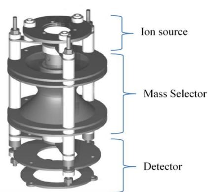
Figure 2: Volatiles Analyser miniature mass spectrometer
