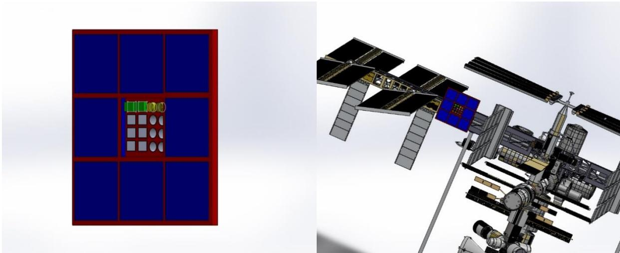
**The first image shows a simple 3D model of the plate, as well as a good camera-angle to monitor experiments. The second image shows an example of the placement of the plate on a space station (not to scale).**
