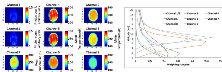
**Figure 1. (Left) Example Earth scan data from a sequence of observations made on July 13, 2010 at 14:10 UTC. (Right) Approximate weighting functions for the Diviner channels when viewing Earth. Channel 1, 2: albedo, channel 3: 7.8 μm, 4: 8.25 μm, 5: 8.55 μm, 6: 13-23 μm, 7: 25-41 μm, 8: 50-100 μm, 9: 100-400 μm.**
