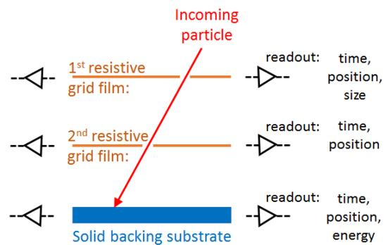
Fig. 2: Schematic of real time sensor design with data readouts
