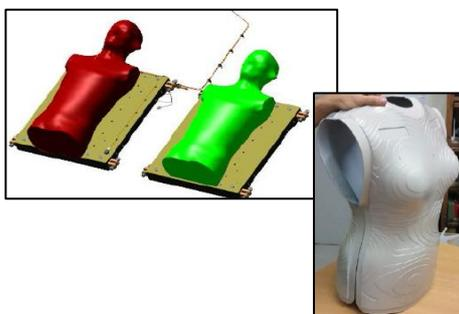
Figure 1 – The MARE Experiment Matroshka Torsos and AstroRad Vest
