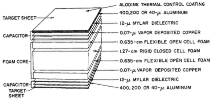
*Concept of the PEGASUS I and II meteoroid large area dust detector. The outer aluminium layer of the capacitor determines the mass threshold for penetrating particles.*
