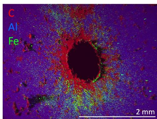
Fig. 1: Residue around penetration hole made by 1mm steel particle impacting Al-coated Kapton foil
