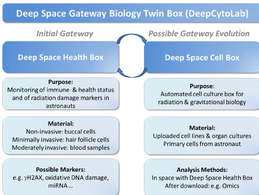
**Figure 1** In the initial phase of the Deep Space Gateway, the “Deep Space Health Box” can be used for monitoring of immune and health status and of space radiation damage in astronauts. After upgrade of the station, the cell culture box called “Deep Space Cell Box” can be added for biological experiments on the station.
