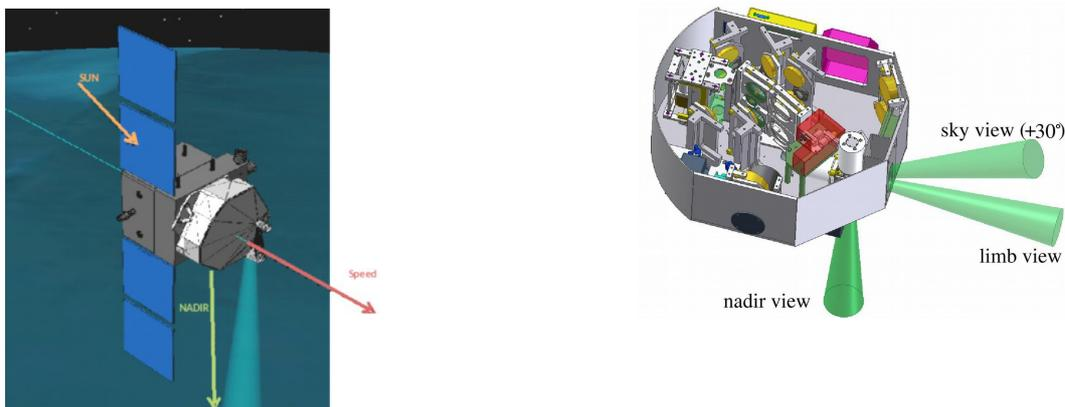
Figs 1 and 2: Schematic representation of the proposed remote sensor (credits: Luca Palchetti, IFAC, Italy).
