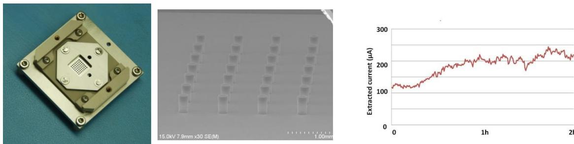
**Figure 3:** Left panel: picture of the extraction device developed for the first set of tests. Panel in the middle: networks of CNT on their substrate. Right panel: example of electron currents extracted using this device during 2 hours. A typical current of  $200 \mu\text{A}/\text{cm}^2$  is produced by this device.
