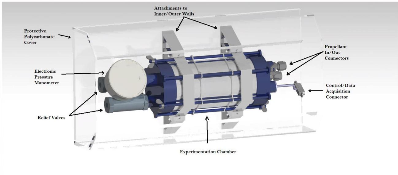
**Figure 1. Schema of GAUSS-PRO chamber at Inner configuration. It would include two relief valves for a double failure tolerant approach, an electronic pressure manometer, strain gauge sensors at the walls, tri-axial accelerometers, and Pt 1000 temperature sensor at the skin and within the chamber at different radius. It would be connected to DSG station telemetry and remotely controlled.**
