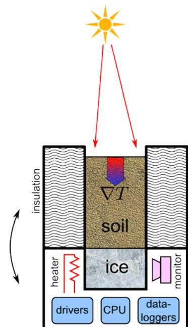
conditions on the surface of Moon. The heat propagating through the soil's layer gradually heats up the frozen volatile and forces it to sublime. The vapour molecules then diffuse through the porous layer (presumably via free molecular flow) and escape into vacuum. The escape rate can be monitored by different means: either optically, with transparent container for volatiles, or by acoustic probing of the ice bulk.
