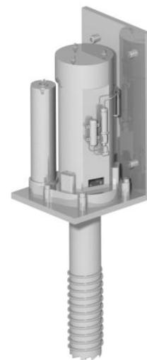
**Figure 1: Left: Render image of LUVMI on the lunar surface. Right: CAD Model of the Volatiles Sampler/Volatiles Analyser instrument package**
