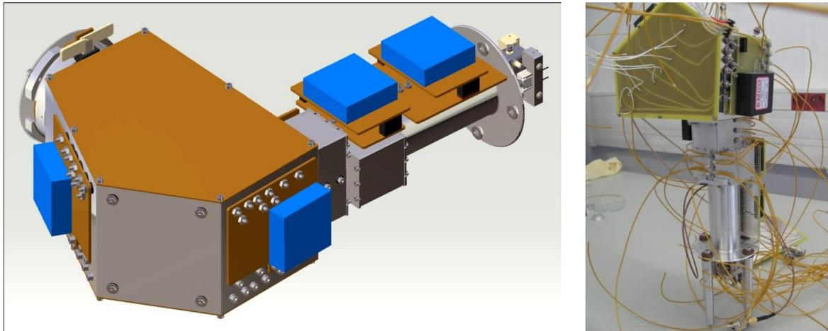
**Figure 2:** Mechanical drawing of NIMEIS and picture of the prototype with a laboratory ionization source.
