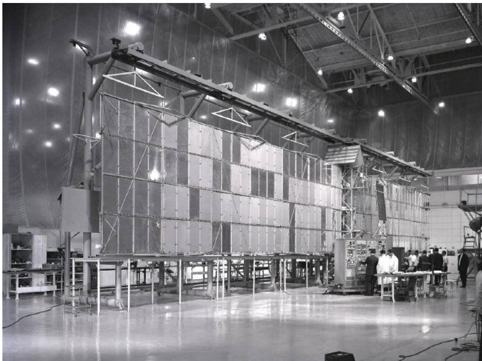
*PEGASUS spacecraft with deployed meteoroid sensor panels. The panels carried 208 segments with a size of 50 cm x 100 cm giving a total sensitive area of 194 m<sup>2</sup> (front and back side).*
