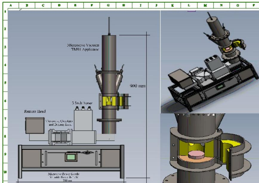
Fig. 1: A concept drawing of a bespoke microwave sintering equipment with a vacuum capability
