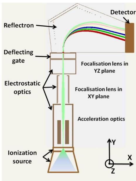
**Figure 1:** Schematic view of NIMEIS. Colors are for energy difference of 1 eV.
