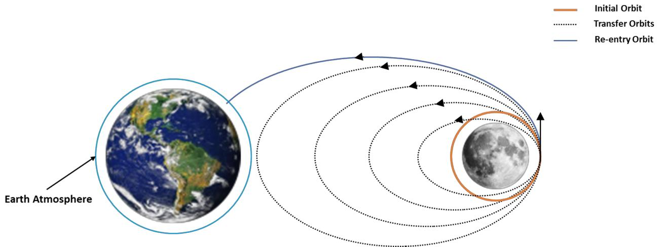
**Figure 1: Passive Waste Disposal Demonstration Mission Concept**
