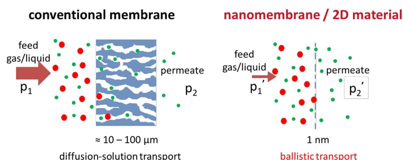
**Fig. 1:** Permeation through conventional membranes and nanomembranes. The ballistic transport needs smaller pressure differences than a diffusion-solution transport:  $(p_1' - p_2') < (p_1 - p_2)$ .
