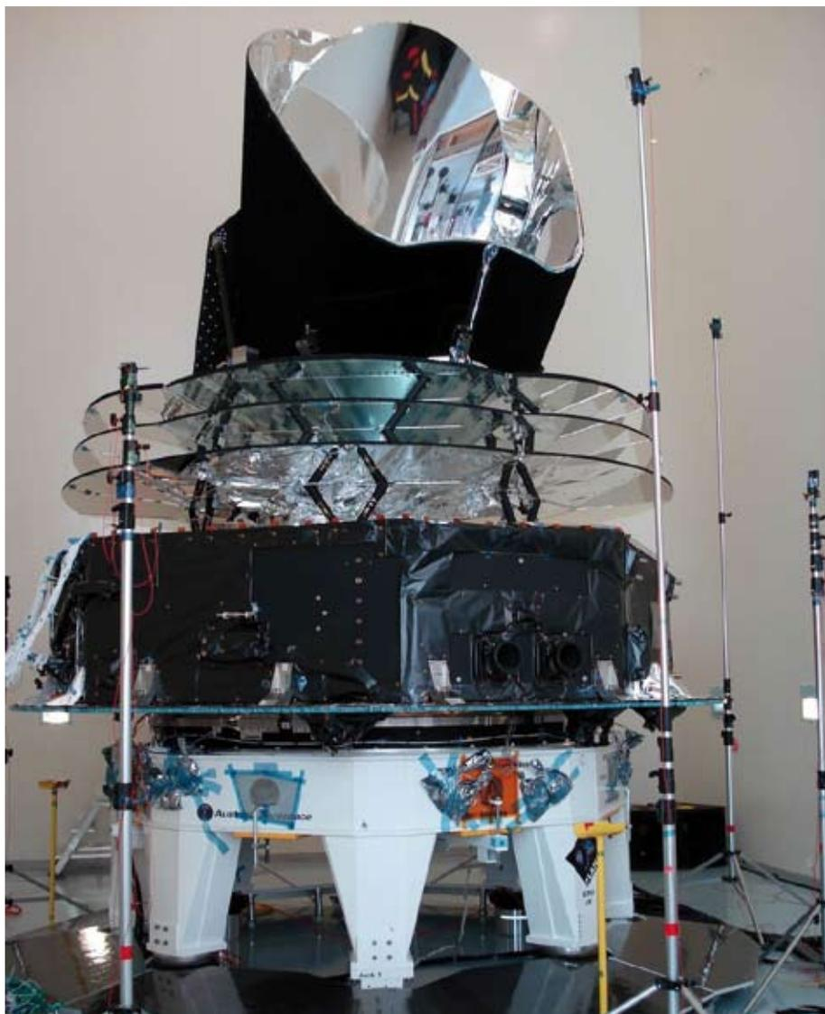
**Figure 4.3.2. The fully-assembled Planck satellite being readied for acoustic tests.**
