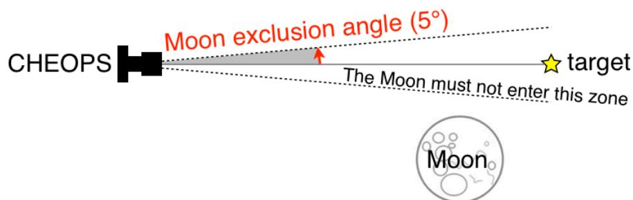
Figure 22 | Illustration of the pointing constraint introduced by SciReq 3.4.
