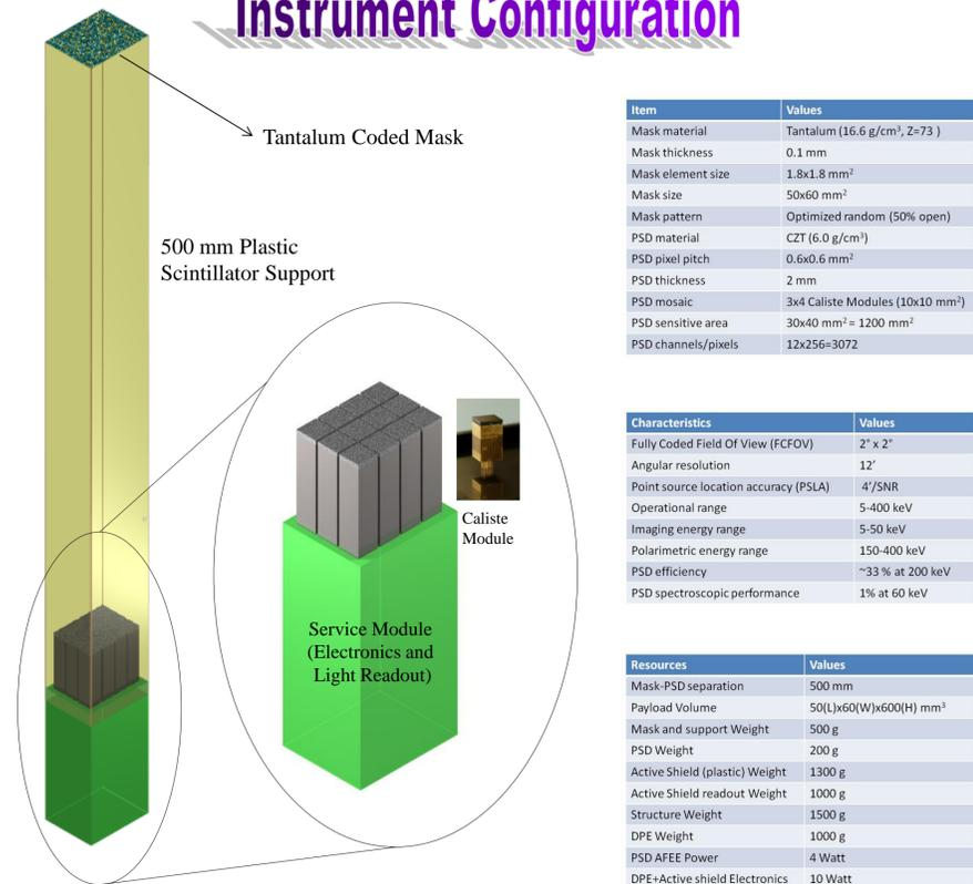
Fig. 2 – Solar polarimeter design
