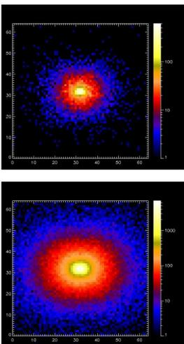
Fig. 4- Simulated double event distributions obtained for a 200 keV (top) and a 400 keV (bottom) 100% polarized monochromatic beam irradiating a matrix central pixel.  $Q_{100}$  of the instrument in the range is calculated from these distribution maps.
