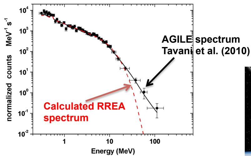
→ PANGU will measure the >10 MeV spectrum with higher resolution imaging (better rejection of earth limb background).
