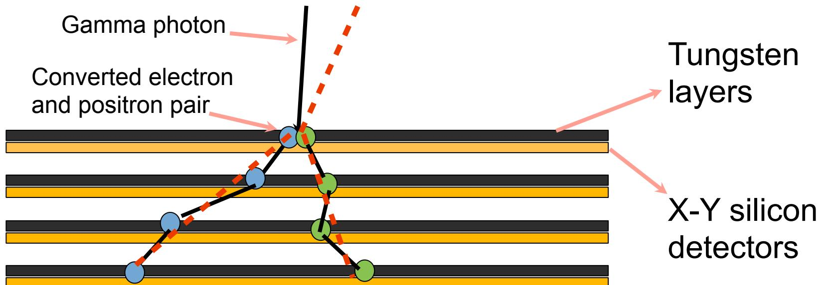
Converted electron/positron pair carries information about the direction, energy and polarization of the **gamma** photon
