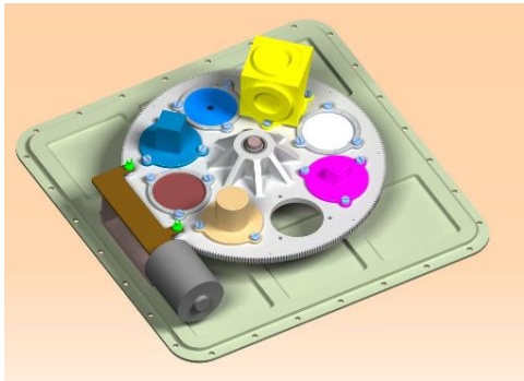
Figure 4-16 Filter wheel with the DU lid and position sensors.
