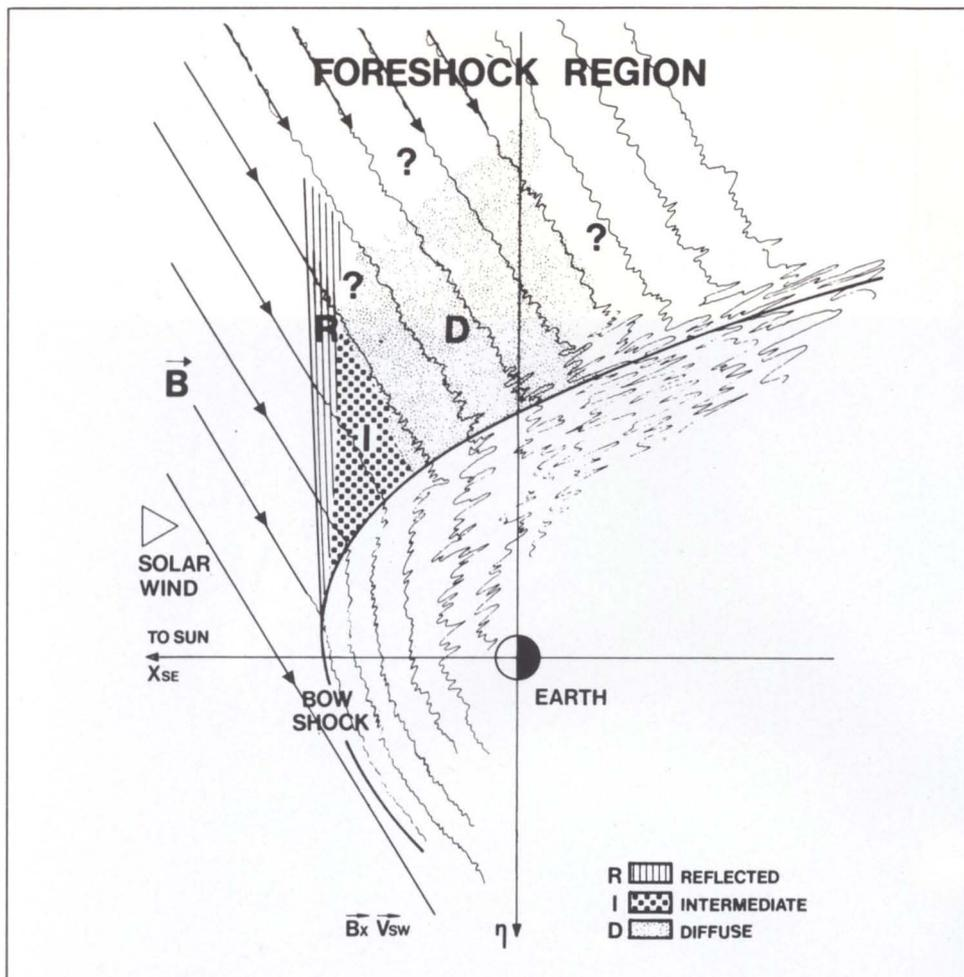
Illustrating where ions are sent from the Earth's bowshock region back towards the sun and along the magnetic field lines. R (reflected), I (intermediate) and D (diffuse) represent characteristics of the ions found in different regions
