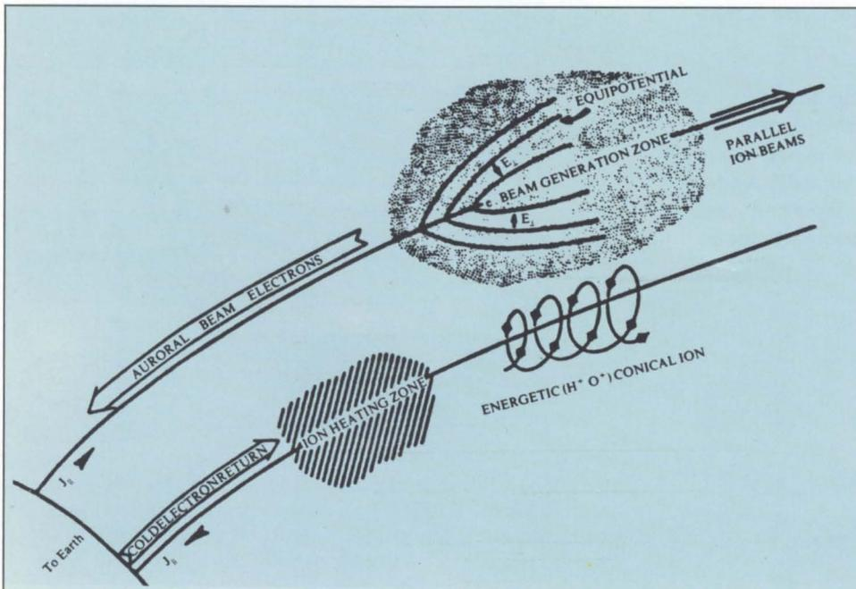
*Schematic of suggested electrodynamic structure of near-Earth magnetosphere at auroral latitudes. An electric double layer accelerates downward (towards Earth) electron and upward ion beams and a consequent  $j_{\parallel}$ . The return current is assumed to be carried by upwardly drifting cold electrons whose bulk energy feeds ion-cyclotron instabilities, which in turn accelerate  $H^+$  and  $O^+$  in the direction transverse to  $B$  (from Ashour-Abdalla & Okuda, 1982)*
