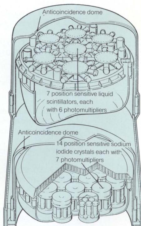
*Schematic of the Imaging Compton Telescope (Comptel) designed to study the sky in the light of low-energy gamma rays from NASA's Gamma-Ray Observatory (GRO). The Comptel Collaboration comprises MPE Garching, ROL Leiden, the University of New Hampshire, and the Astrophysics Division, Space Science Dept. ESA.*
