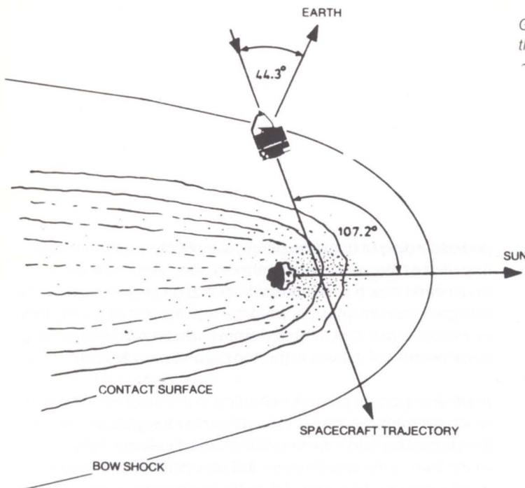
Geometry at Halley encounter. The spacecraft will be aimed to pass the nucleus on the sunward side. A bow shock is expected at  $\sim 10^5$  km, a contact surface at  $\sim 10^3$  km from the nucleus
