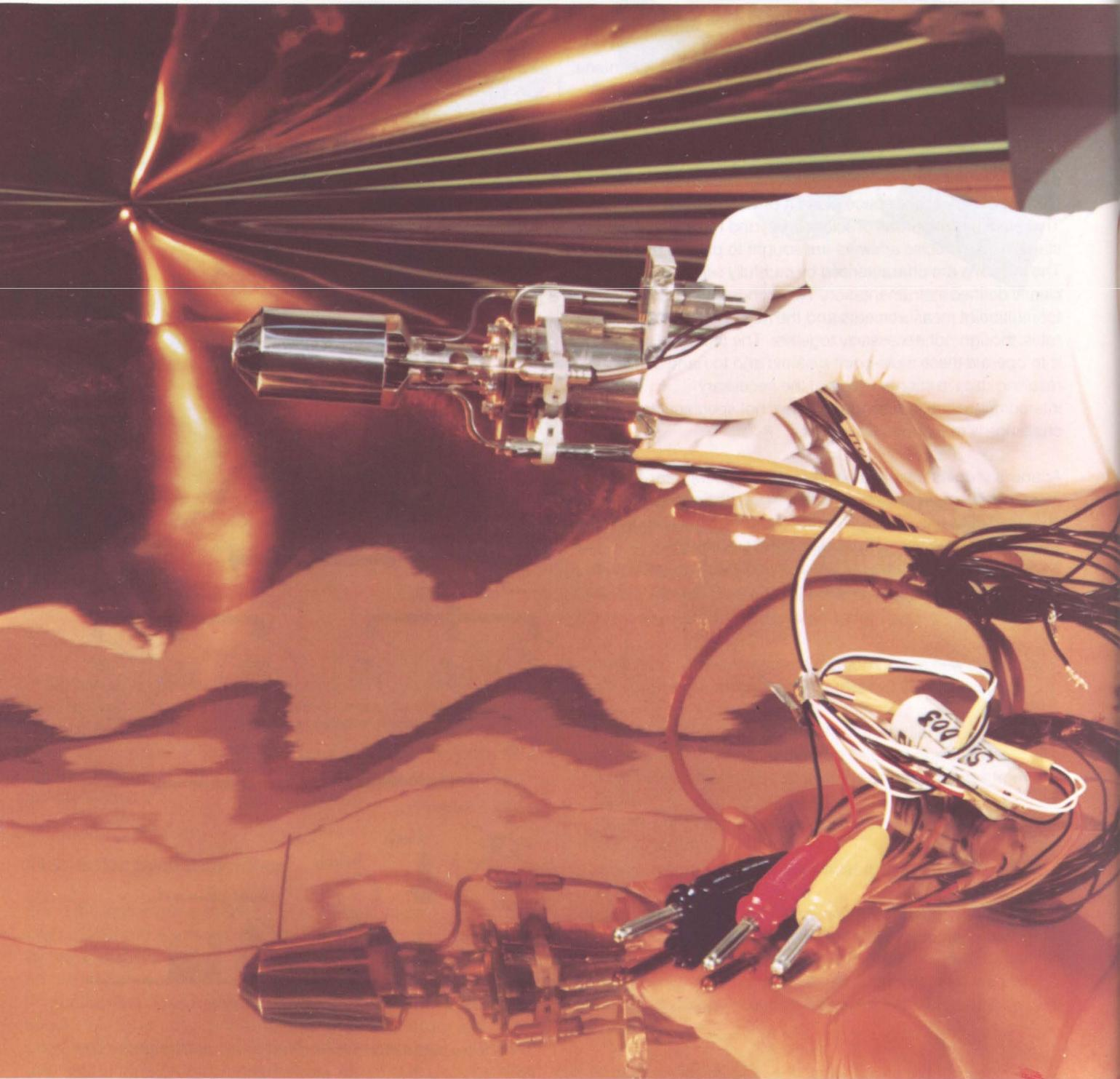
*The 2-N thruster for use on board ISPM spacecraft. (Photo ERNO, Bremen).*
