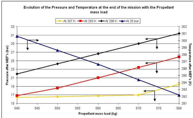
Fig. 4. Final Pressure at the end of mission and the temperature in the ullage vs propellant load.
