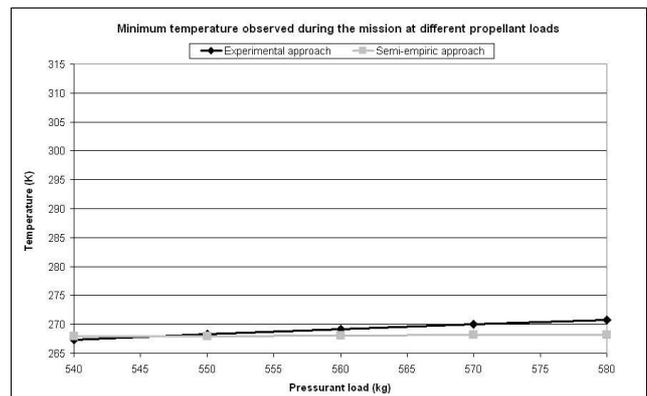
Fig. 6. Minimum expected temperature in the Pressurant tank vs. propellant load.
