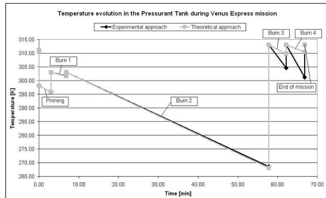
Fig. 3. Evolution of the temperature in the pressurant tank with time.
