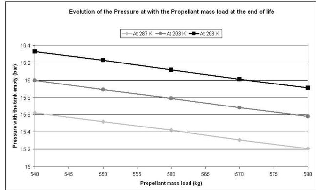
Fig. 5. Final Pressure when the tanks are empty vs propellant load.
