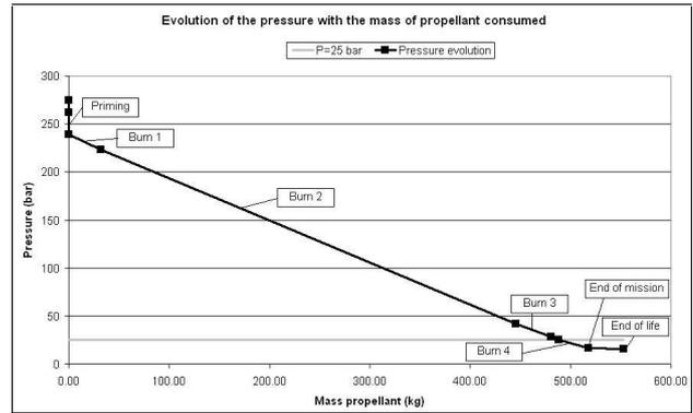
Fig. 2. Evolution of the pressure in the pressurant tank with the propellant consumption.
