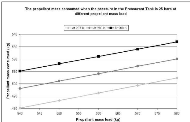
Fig. 7. Propellant mass consumed when the pressure is 25 bars vs. propellant load.
