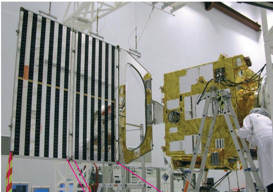
Fig. 9a. The solar array during integration and deployment testing at Intespace.
