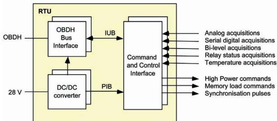
Fig. 14. The Venus Express RTU. IUB: Internal User Bus. PIB: Power Interchange Bus.
