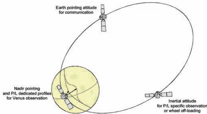
Fig. 4. The manoeuvrability of Venus Express required for Venus nadir observations, Earth pointing attitudes and inertial attitudes for specific payload (P/L) observations.
