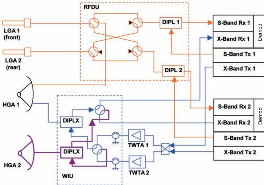
Fig. 10. RF communications block diagram. Purple denotes the hardware added to the Mars Express design: HGA2, diplexer and waveguide.
