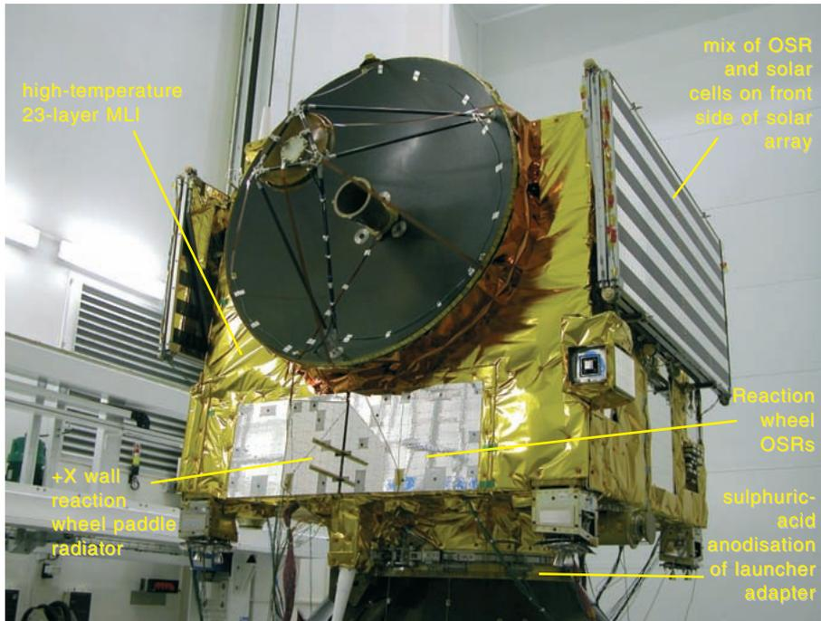
Fig. 2. Venus Express during integration at Intespace (Toulouse, F), showing the thermal control of the +X wall and the solar array. The MultiLayer Insulation (MLI) and Optical Solar Reflectors (OSRs) are clearly visible.
