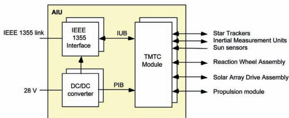
Fig. 15. The Venus Express AIU. IUB: Internal User Bus. PIB: Power Interchange Bus. TC: telecommand. TM: telemetry.
