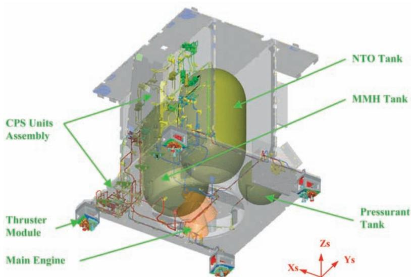
Fig. 7. Layout of the propulsion system.
