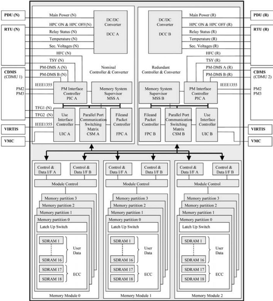
Fig. 16. The architecture of the Solid-State Mass Memory. HFC: High-Frequency Clock. TSY: Timer Synchronisation.
