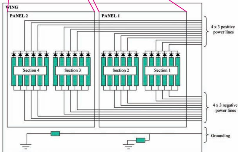
Fig. 9b. Solar wing block diagram.
