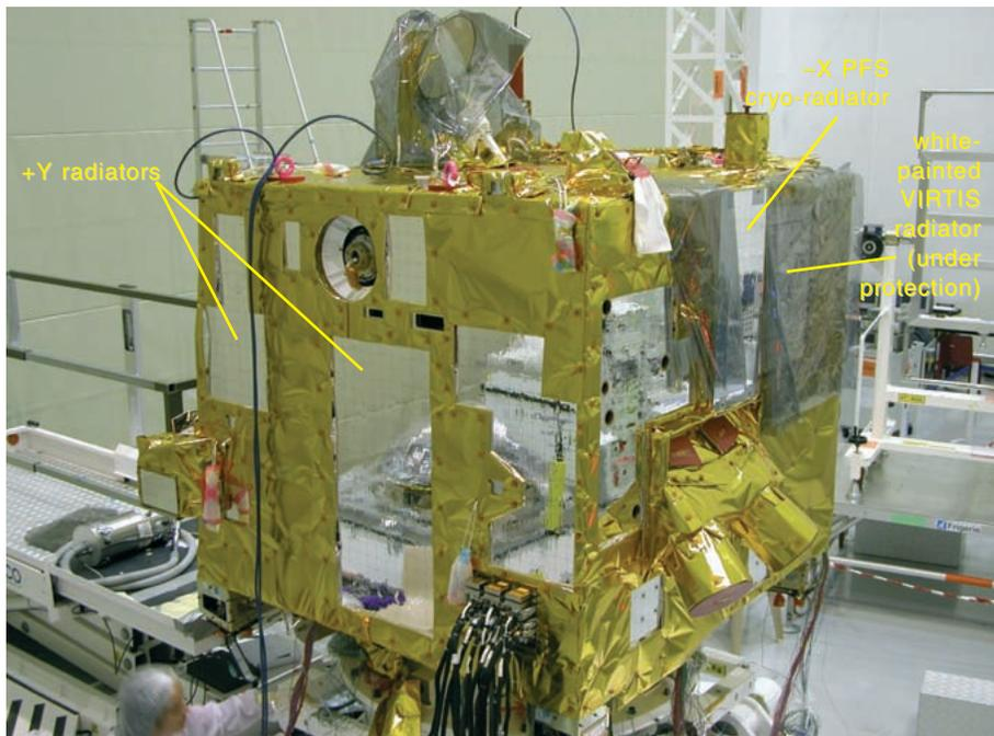
Fig. 3. Venus Express during integration at Intespace (Toulouse, F), showing the thermal control of the +Y and -X walls.
