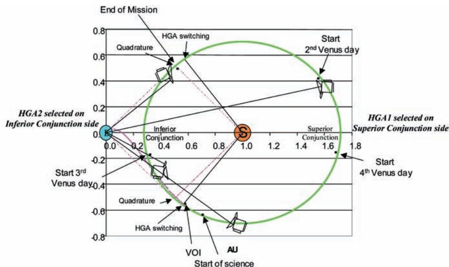
Fig. 11. HGA selection combined with an optimised attitude guidance law, shown in a fixed Earth (E)-Sun (S) reference frame.
