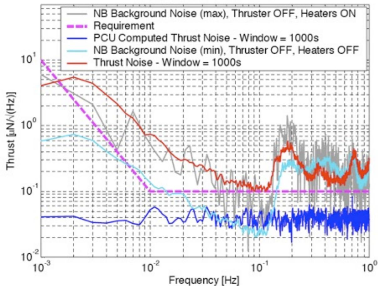
Thrust Noise @ 25  $\mu$ N - PSD
