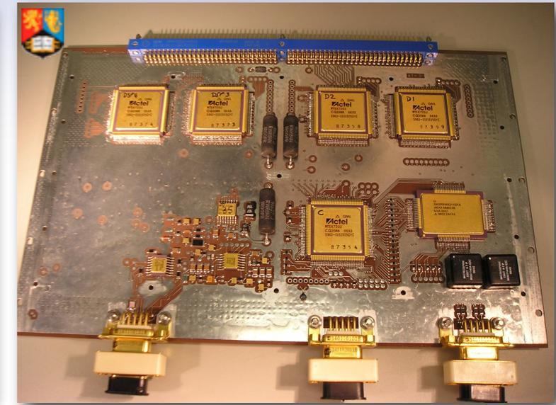
Phasemeter analogue and digital proto-flight boards
