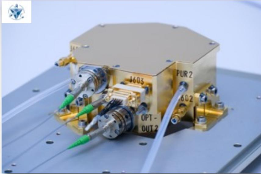
Laser Modulator flight unit
