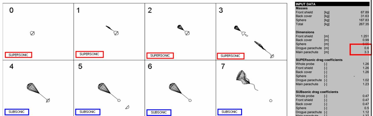
CONCLUSION of the above: It is possible to change back to EDLS option 2. The ballistic coefficients differ sufficiently and the drogue parachute that shall be jettisoned with the mortar is small. Mortar dimensions fit in this case the current configuration design.
