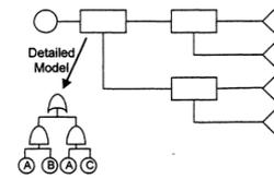
Figure 2: Multilayered Event Sequence Diagram / Fault Tree model.
