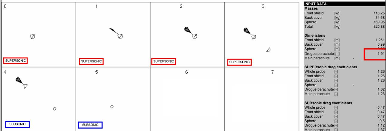
Conclusion: 1.9 m (projected diameter) Conical Ribbon parachute
