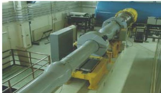
(Free piston shock tunnel HEG, Picture: Courtesy DLR)
