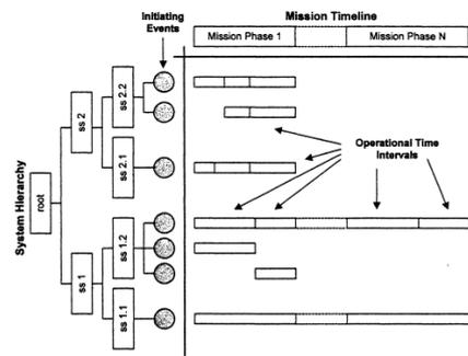
Figure 1: High-Level Model Structure based on System Hierarchy and Mission Timeline.
