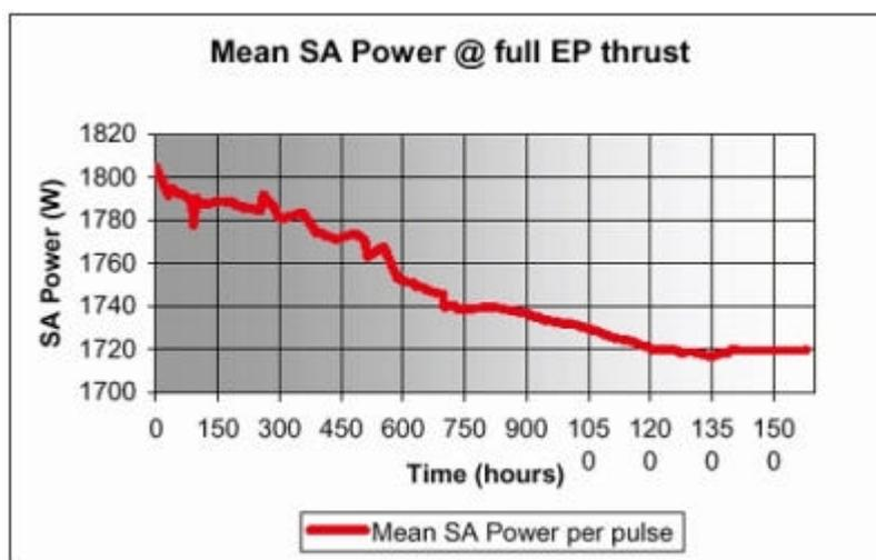
The graph shows the measured power produced by the solar arrays when the electric propulsion is operating at full power starting from the beginning of the mission.
