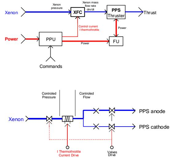
Figure 5. Xenon flow regulation loop and Xenon flow Controller functional diagram.
