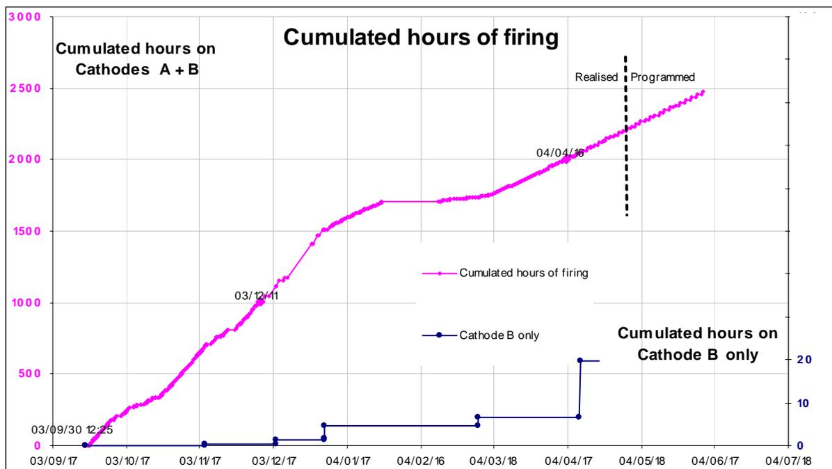
Figure 9. Total thrusting time of the Smart-1 EPS. Since the 30<sup>th</sup> of September, the EPS was used quasi-continuously. Thousand hours occurs on 11<sup>th</sup> of December and two thousand of hours occur the 16<sup>th</sup> of April. The longest continuous firing occurs between December 23<sup>rd</sup> and January 2<sup>nd</sup> 2004, for 240 hours (10 days).
