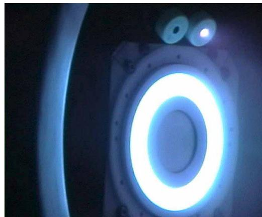
Figure 4. Thruster PPS®1350-G FM during acceptance tests firing sequence.
