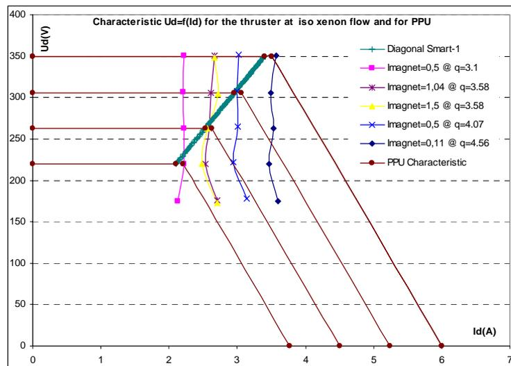
Figure 6. The diagonal with the 117 steps of the variable power feature of Smart-1 given by the Nominal Power Set parameter. The EPS Power at thruster level is of course  $U_d \cdot I_d$ . Thruster characteristics at iso-mass flow and only 4 of the 117 characteristics provided by the PPU/TSU are shown.
