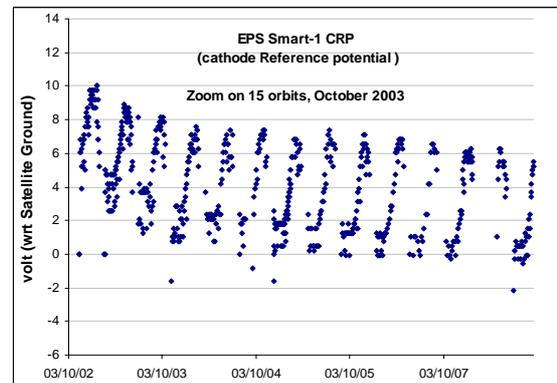
Figure 13. Zoom on 15 orbits, Cathode potential with respect to the electrical ground of the satellite.
