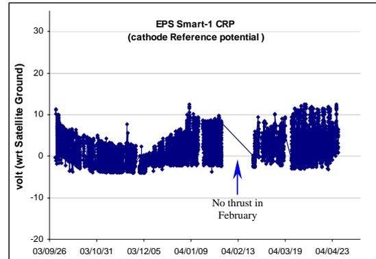
Figure 11. Long term (7 months) Cathode potential with respect to the electrical ground of the satellite.
