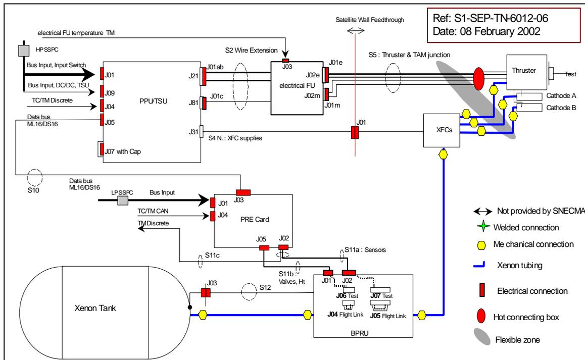
Figure 1. EPS functional diagram: the xenon system feeds the thruster cathodes and anode.
