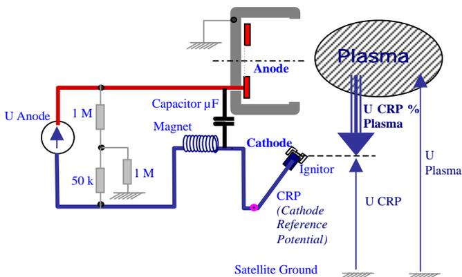
Figure 12. Sketch of the simplified electrical circuit of the EPS Smart-1. The Cathode potential with respect to the electrical ground of the satellite is called CRP.
