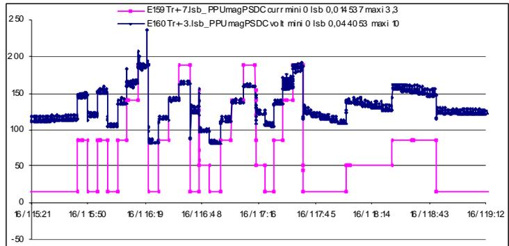
Figure 15. Magnet current during a characterisation test sequence of the EPS Smart-1 in flight.
