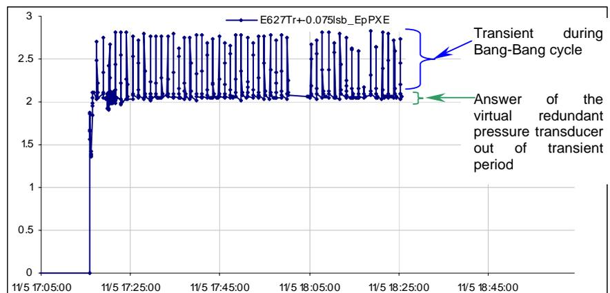
Figure 18. Virtual redundant pressure transducer telemetry: the values given by the computations are fully in line with the real transducer telemetry (out of the transient periods).
