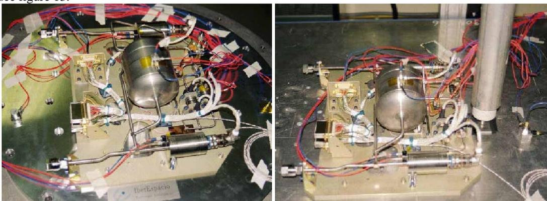
Figure 13. BPRU during the vibration sinus, random and shock tests of the acceptance tests sequence performed by INTA /Iberespacio
