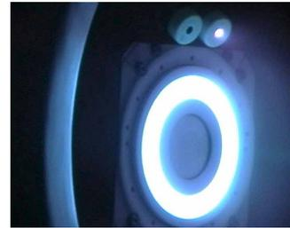
Figure 4. Thruster PPS®1350-G FM during acceptance tests Firing sequence.
