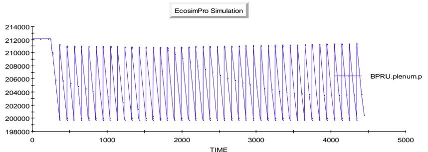
Figure 16. EcosimPro simulation of the pressure steps with the inputs coming from the flight data: Behaviours are very similar with fig. 15, as expected.
