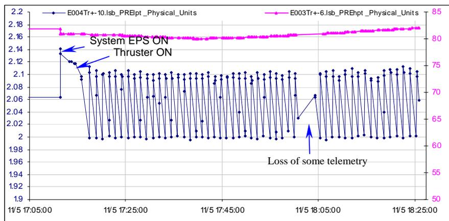
Figure 15. Behaviour of the pressure regulation, in flight, May 2004, duration 80 minutes: Pressure steps between 1.995 bar and 2.11 bar (ie  $\pm 0.058$  bar) occurs at each Bang-Bang cycle. The High pressure around 82 bar shows slow variations.
