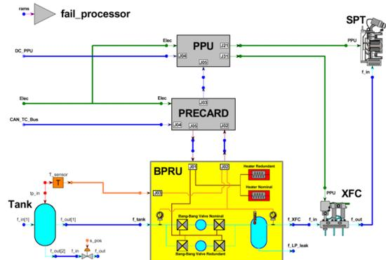
Figure 12. EPOS an EPS simulation software which includes the functional modelisation of the BPRU, on EcosimPro
