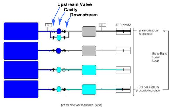
Figure 8. BPRU sketch of the robust concept
