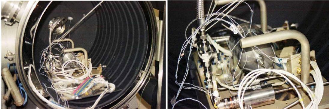
Figure 14. BPRU during the thermal vacuum acceptance tests with xenon, INTA facility
