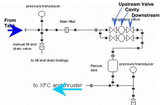
Figure 7. BPRU system functional flow diagram
