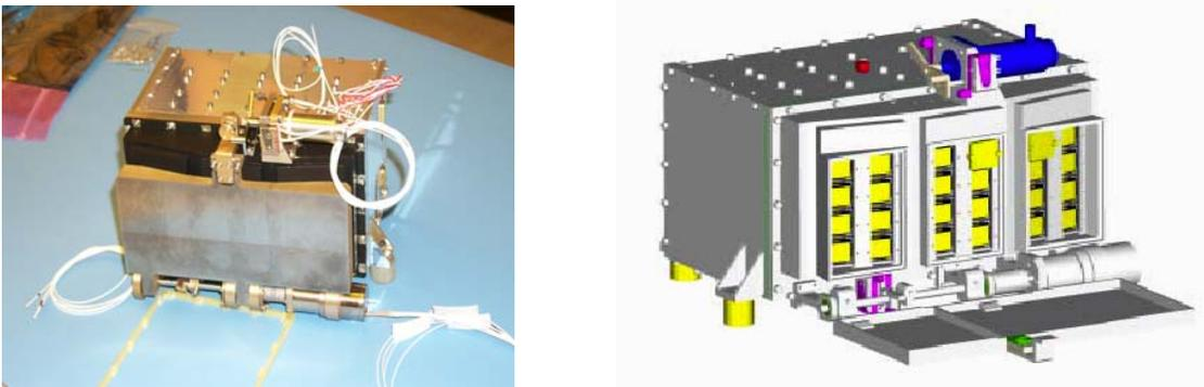
Fig.2: D-CIXS flight unit (left) vs mid-term design (right). D-CIXS was built in Rutherford Appleton Labs, with support from UK, ESA, Finland, France, Spain, Sweden, Japan, India, US. It has a 12 x 32 deg Field of View, for Global mapping of the lunar surface (elemental composition) via X-ray fluorescence. It uses a parallel X-ray Solar Monitor, built in Finland, to monitor Solar X-ray flares and coronal monitoring (calibration).
