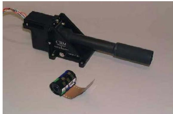
It provides high-resolution multi-colour imaging with up to 40 m pixel at 400 km perilune, and complements SIR and D-CIXS and Apollo/Clementine. It supports the laser-link experiment, OBAN On Board Autonomous Navigation Experiment, RSIS Radio Science Libration Experiment.
