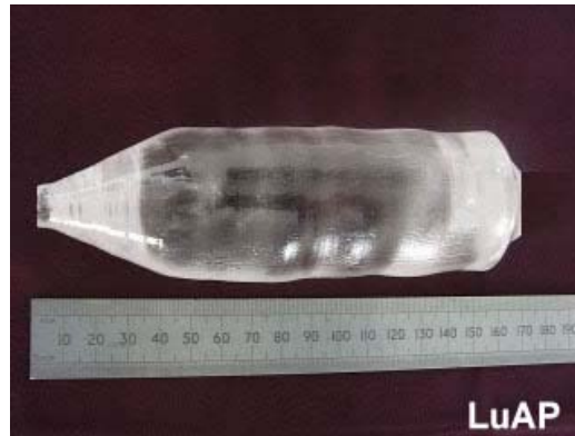
Fig. 4.4 Photograph showing the largest LuAP crystal reported to date
