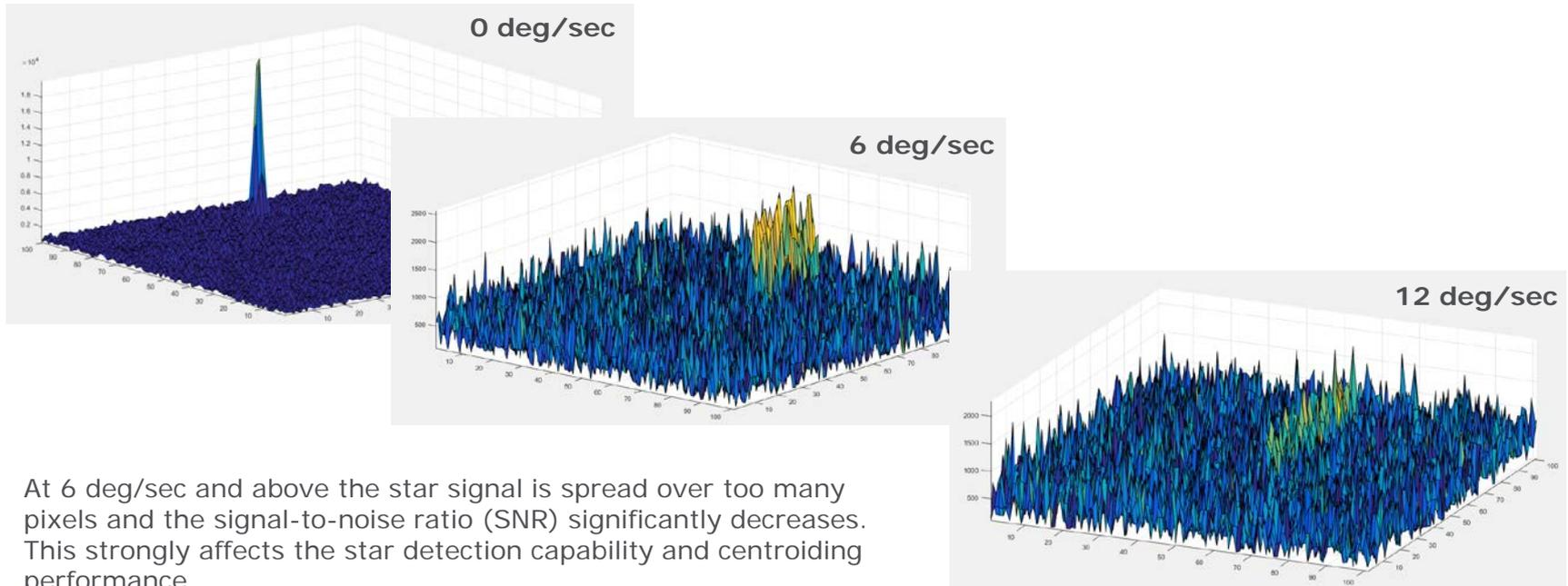
At 6 deg/sec and above the star signal is spread over too many pixels and the signal-to-noise ratio (SNR) significantly decreases. This strongly affects the star detection capability and centroiding performance.
