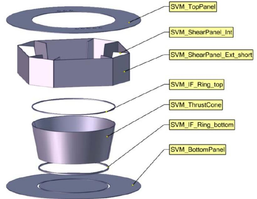
Stiffer and heavier configuration → better suitable for bending issues on CMB
