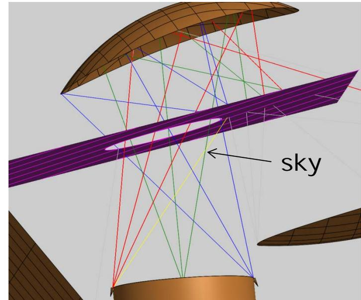
A first assessment of the feasibility and reliability of the baffle modelled as aperture on screen has been carried out. The screen model shows as the feeds radiate through the screen.
