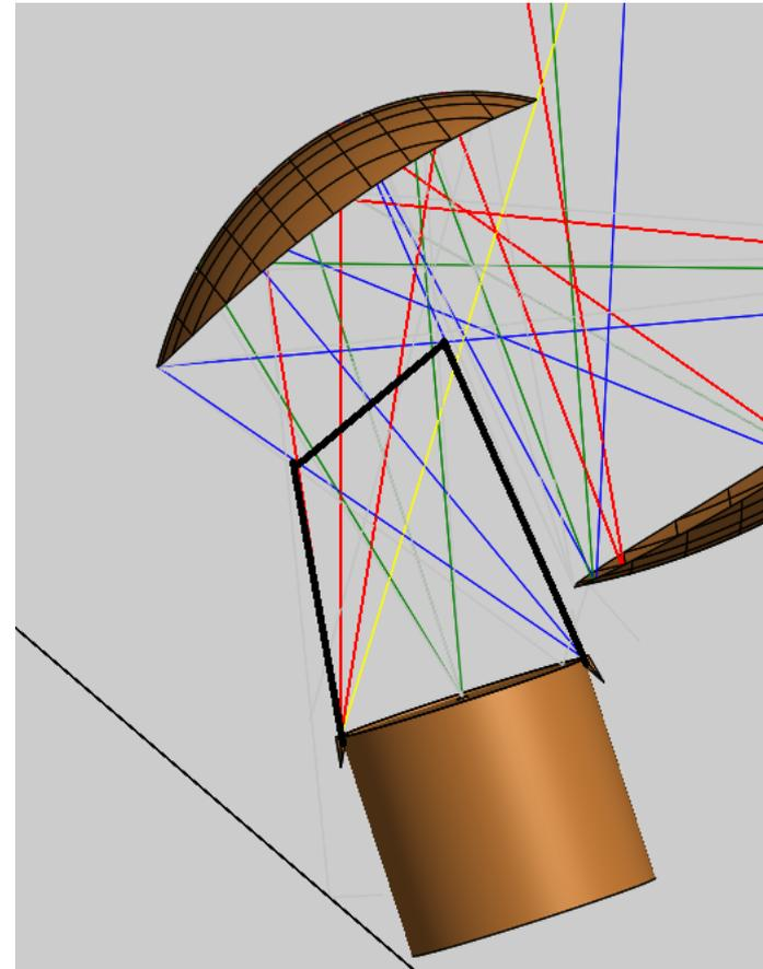
Making use of ray tracing a baffle has been designed.
