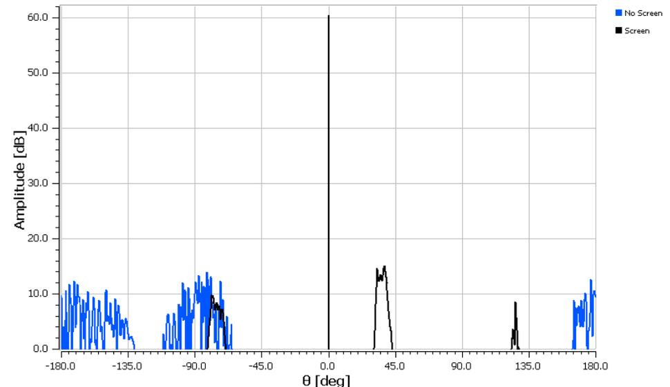
Assessment via PO/GTD analysis of the reflection of the **outer surface of the baffle via a PEC model.**
