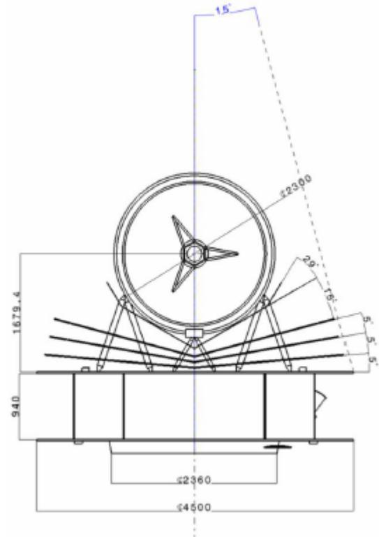
Core+ → Cryogenic structure concept on Gregorian configuration
