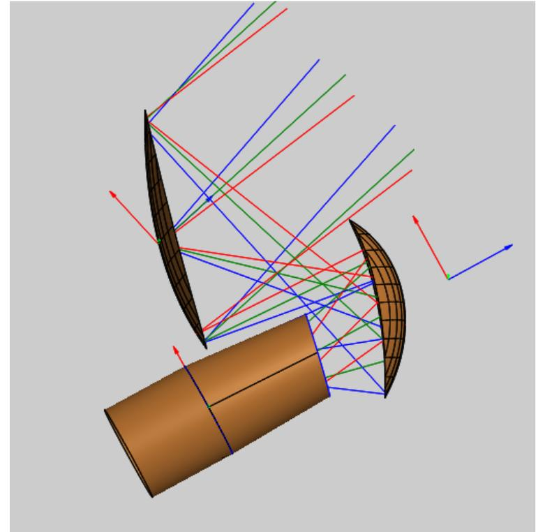
Ideally the entire baffle should be modelled as an absorbing surface on the inside and reflective/diffusive surface on the outside.
