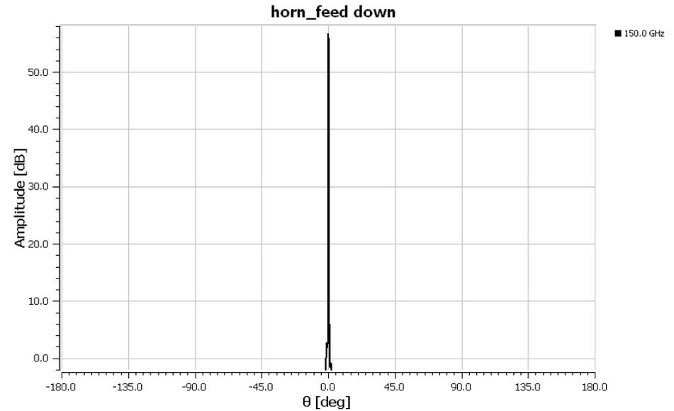
1. The optics as designed in first approximation shows focused central beam without main distortion.
