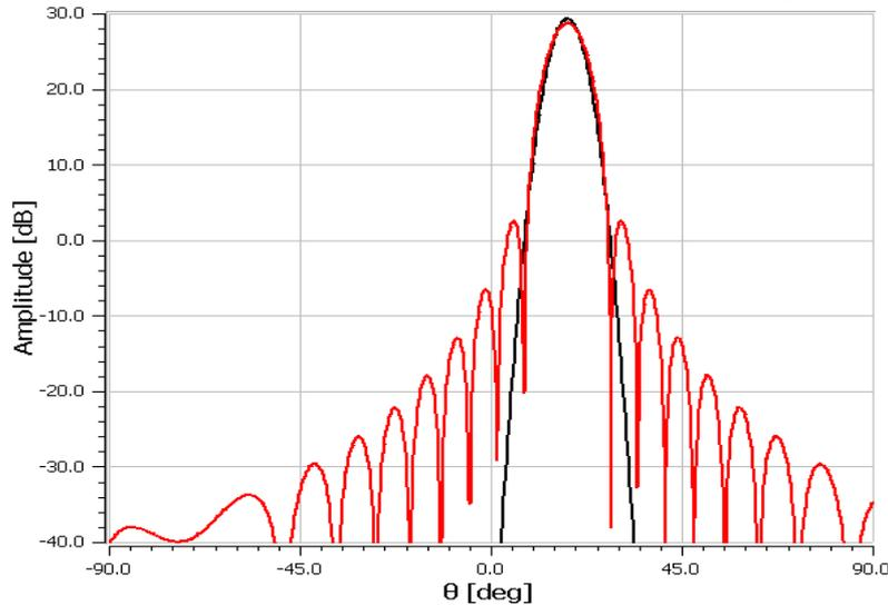
Patterns tapered -23db at 9 deg – Feed down
