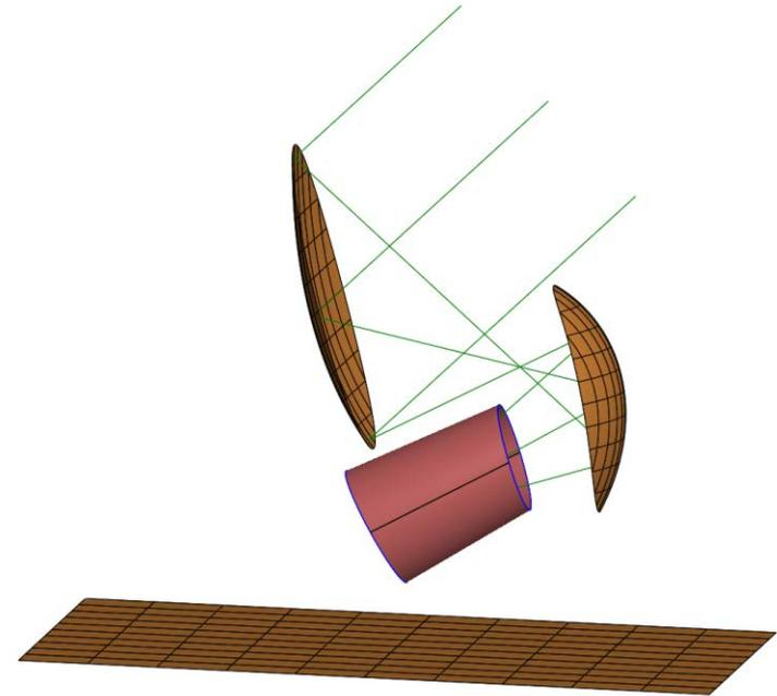
A gaussian feed is placed in the centre of the FPU:
