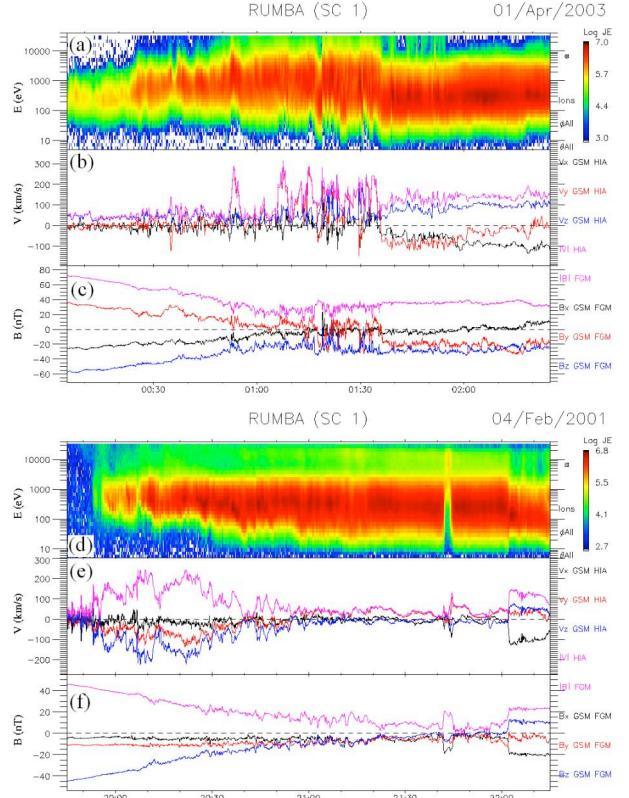
Fig. 4: Cluster time-series of two selected outbound traversals of the high-altitude cusp region on April 1<sup>st</sup>, 2003 for southward IMF (upper part) and on February 4<sup>th</sup>, 2001 for northward IMF (lower part). The three panels show: the ion energy-time spectrogram, the ion velocity components, where all ions are assumed to be protons, and the magnetic field components. Magnetopause crossings are located at 01:40 and 22:02 UT respectively for the two events.
