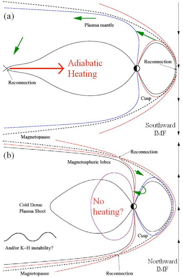
Fig. 6: Schematic of solar wind plasma circulation and magnetic topology of the magnetosphere in the context of magnetic reconnection for (a) southward and (b) northward IMF directions.
