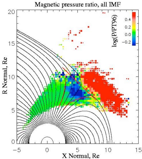
Fig. 3: Spatial distribution of the ratio of the measured magnetic pressure ( $B_2/2\mu_0$ ) to that calculated from the T96 model. The color palette illustrates the amplitude of the magnetic pressure ratio with blue indicating a small measured magnetic pressure. In this figure all IMF conditions are taken into account. The three red lines surrounding the magnetic field cavity correspond to approximate boundaries of the high-altitude cusp. Other details are given in the caption for Figure 2.
