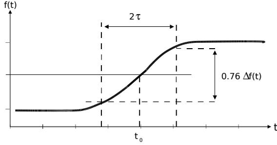
Figure 2. Idealized magnetic field (or density) profile across a discontinuity, and one possible definition of crossing time,  $t_0$ , and crossing duration,  $2\tau$ . With a known velocity,  $V_d$ , of the discontinuity, the thickness,  $d_d$  is given by  $2\tau * V_{MP}$ . After Paschmann et al. (2005)
