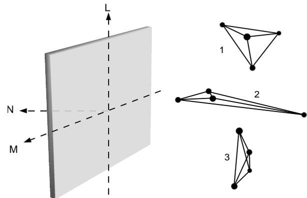
Figure 3. Illustration of different Cluster spacecraft tetrahedron shapes relative to a discontinuity. The various configurations give various success rates; The regular tetrahedron shape in configuration 1 is the best compromise to infer orientation and motion. In the elongated configuration in 2 and the nearly planar configuration in 3, the orientation, respectively the velocity is very sensitive to timing accuracy.
