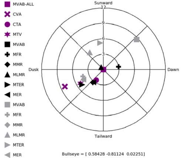
Figure 6. Polar plots of normal orientations obtained from various methods during a magnetopause crossing on 5 July, 2001. Each symbol represents one method to determine the orientation of a discontinuity (see text for abbreviations). The center of the plot (the “bullseye” normal) is here the  $\mathbf{n}_{COM}$  normal based on MVAB results from each spacecraft.
