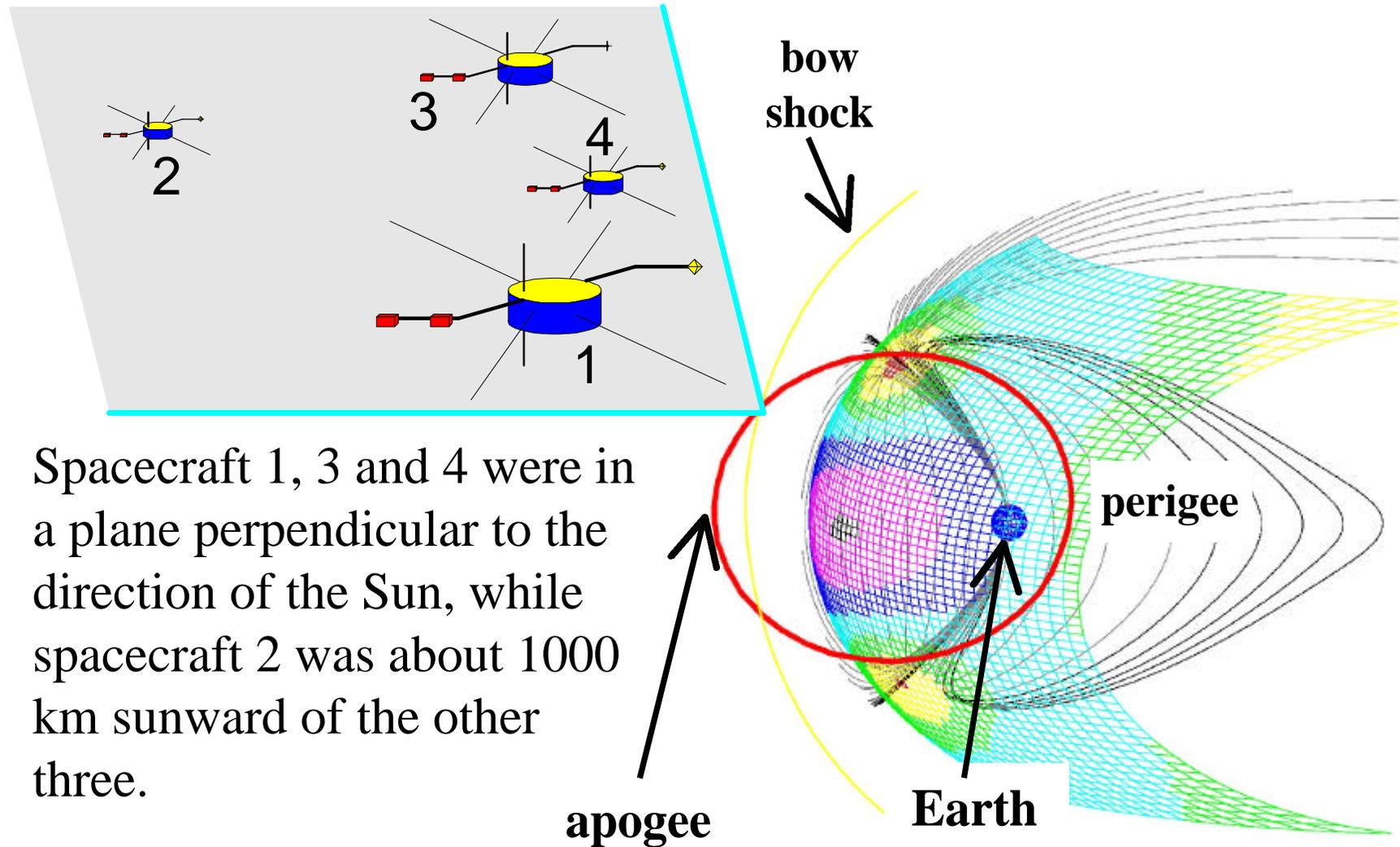
Spacecraft 1, 3 and 4 were in a plane perpendicular to the direction of the Sun, while spacecraft 2 was about 1000 km sunward of the other three.
