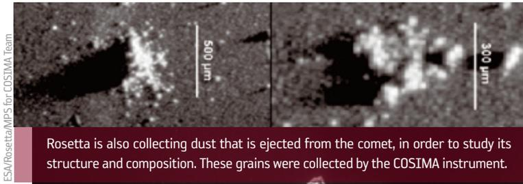
Rosetta is also collecting dust that is ejected from the comet, in order to study its structure and composition. These grains were collected by the COSIMA instrument.
