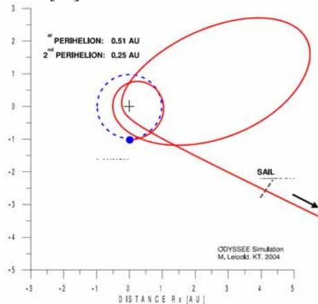
Figure 11: Double photonic assist for the solar sail based IHP transfer [21]
