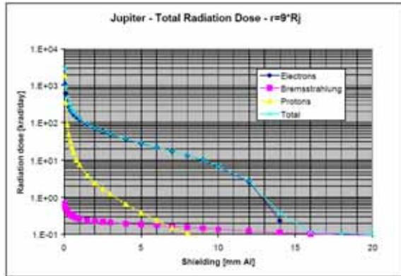
Figure 10: Ionizing dose as a function of shielding thickness for  $9R_J$  equatorial distance from Jupiter
