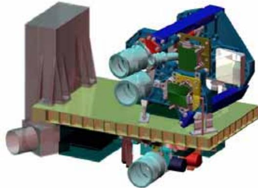
Figure 14: Potential design of a bread board for a reduced HIPS with laser altimeter, cameras, UV and IR mapping spectrometer [26]
