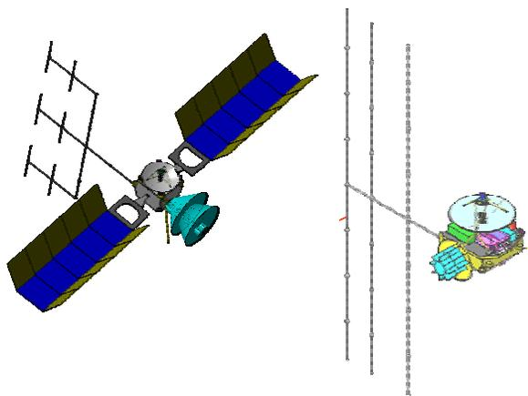
Figure 9: The Jupiter Europa Orbiter (JEO) based on solar power (left) or alternative RPS power (right) with a further developed antenna design for the ground penetrating radar
