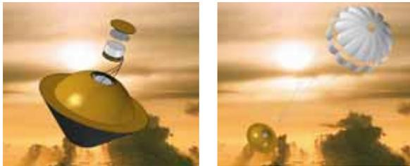
Figure 2: Pilot chute deployment and probe descending on the main parachute [5]
