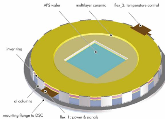
**Figure 5.1.2** – Schematic diagram of the NFI Focal Plane detector (NFI1 – STJ / NF2 - TES).
