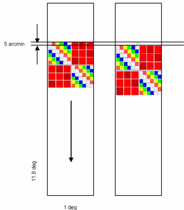
Figure 2 WFI FPA layout and scanning concept
