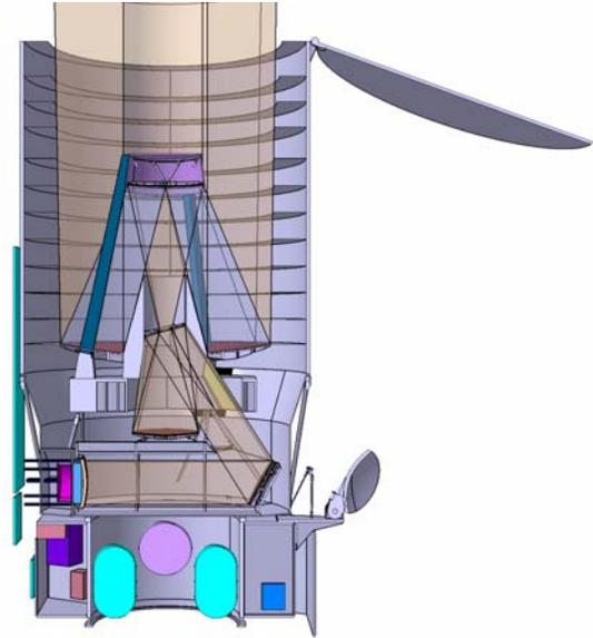
Figure 6 WFI spacecraft configuration
