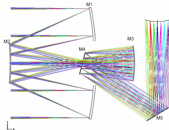
Figure 3 Telescope optical design for WFI
