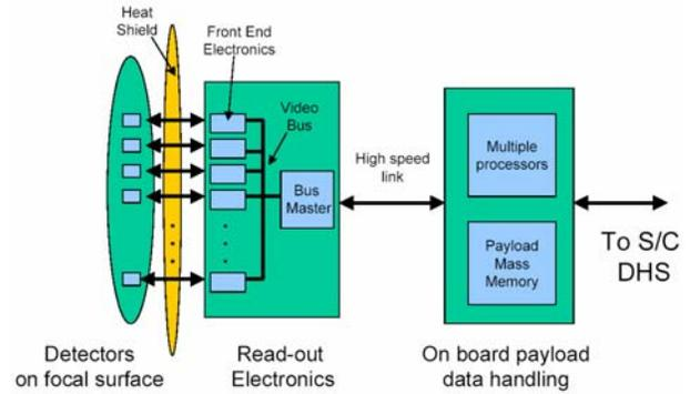
Figure 4 Block-diagram of the WFI camera
