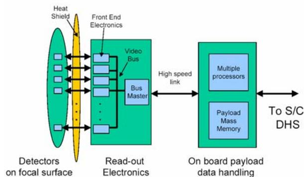
Figure 4 Block-diagram of the WFI camera
