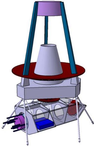
Figure 5 The WFI telescope and instrument
