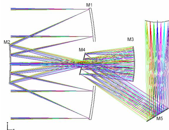
Figure 3 Telescope optical design for WFI
