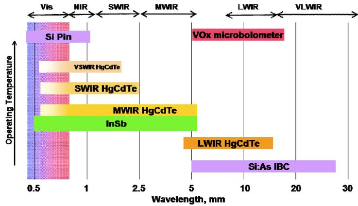
Figure 1. High-performance detector materials available at Raytheon. Operating temperatures for low-background systems is shown qualitatively for each material along with the spectral band of greatest sensitivity. Spectral response of HgCdTe into the visible band has been demonstrated by removing the detector substrate.
