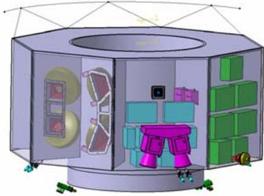
Structure – octagonal shape with outer diameter of 2.2 m → side to side ≈ 2.07m
