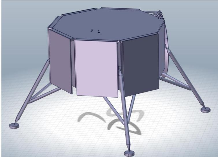
Figure 11-5: LM main structural elements and legs
