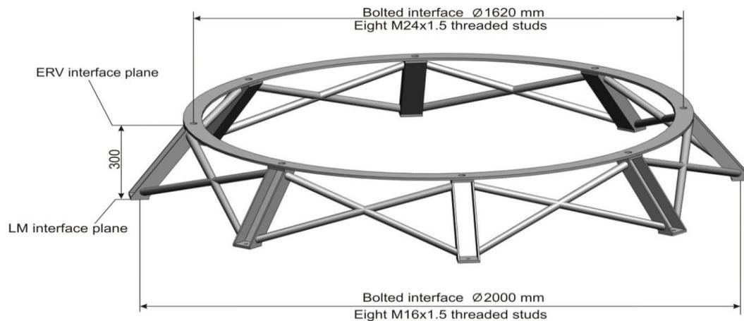
**Figure 7-6: Proposal for LM/ERV adapter**
