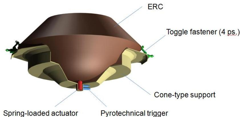
**Figure 7-1: Principle scheme of the ERV/ERC separation system**
