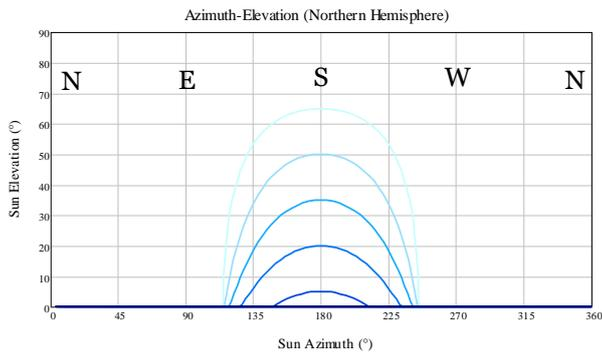
**Figure 16-9: Sun Elevation versus Azimuth, for different landing site latitudes (0° to +90° in steps of 15° - May 2024)**
