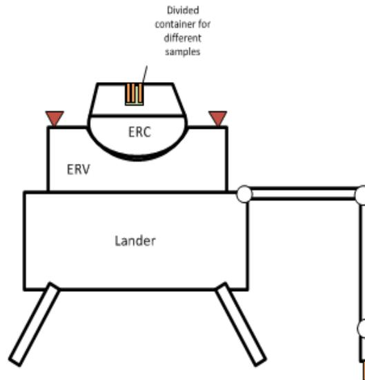
**Figure 24-2: Schematic of the sample container in ERC**
