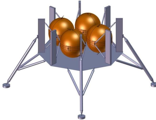
**Figure 10-4: LM Propulsion tanks accommodation**
