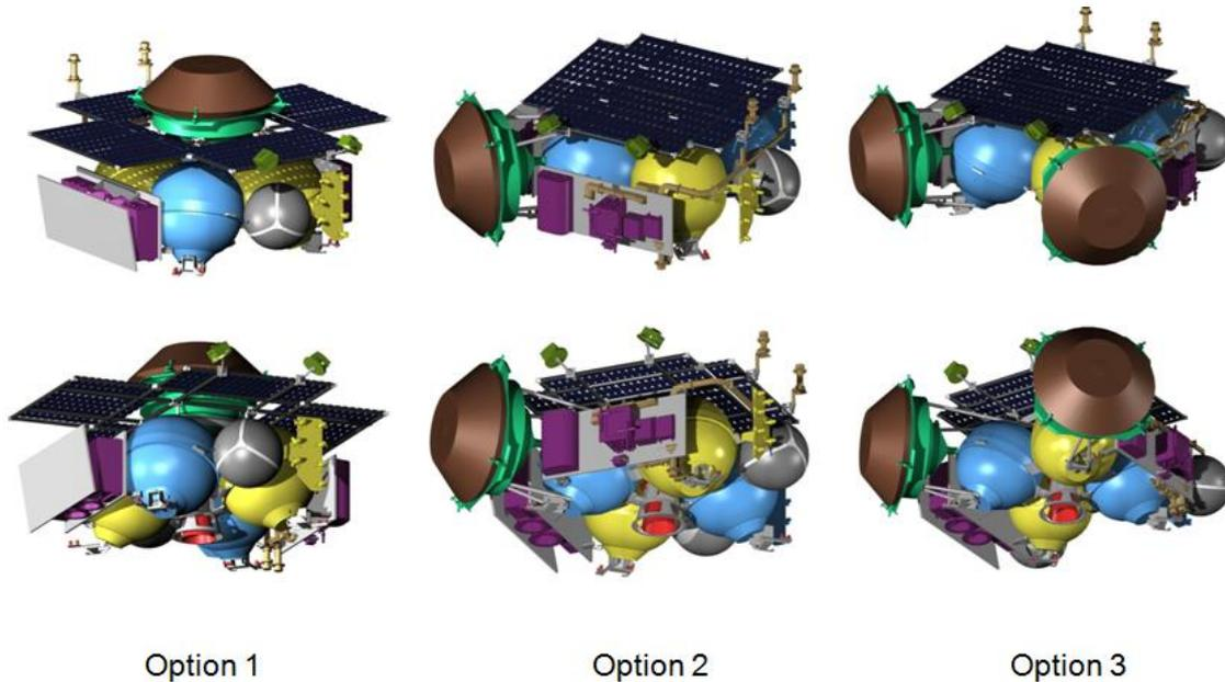
**Figure 7-2: ERV design options with separation system placed in ERC TPS area**
