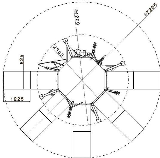
**Figure 10-11: Phobos-SR – LM – dimension in deployed configuration - top view**
