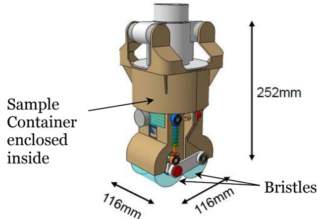
**Figure 24-10: Example of a conceptual design of the Sampling Tool (Airbus DS)**
