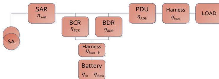
**Figure 16-19: Simple model used for energy balance analysis**
