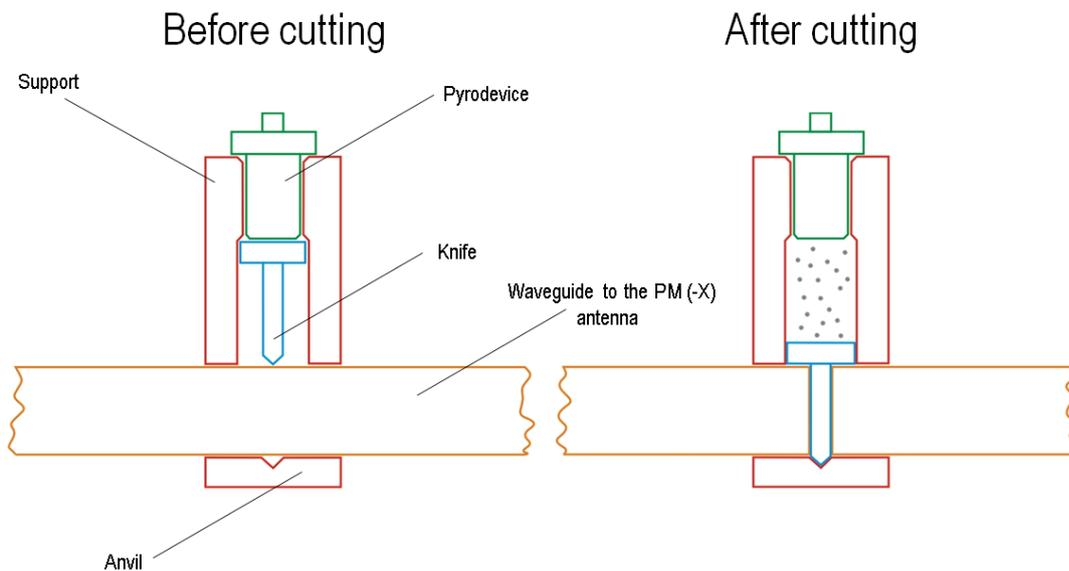
**Figure 6-2: Pyrotechnical knife cutting process scheme**
