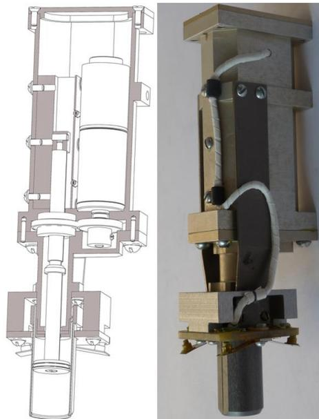
**Figure 25-2: SD of Phobos Soil mission (proposed for PhSM)**
