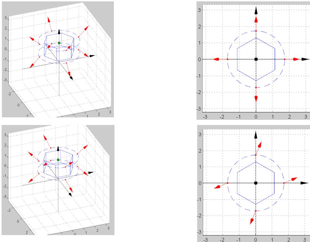
**Figure 15-6: Configurations with 8 RCS tilted 45 deg wrt vertical. Azimuth angle equal to 0 deg (top) and 22.5 deg (bottom)**
