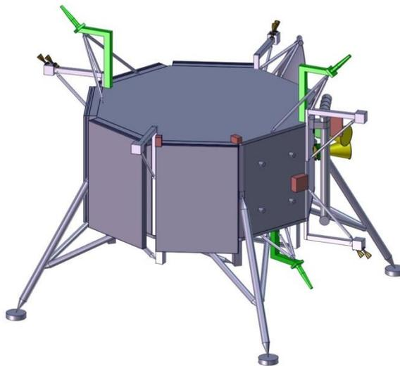
**Figure 10-3: Phobos-SR – LM stowed configuration**
