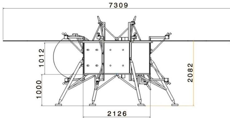
**Figure 10-12: Phobos-SR – LM – dimension in deployed configuration - side view**
