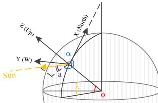
**Figure 16-8: Definitions of Longitude ( $\lambda$ ), Latitude ( $\phi$ ), Elevation ( $a$ ) and Azimuth ( $\alpha$ ) used in this chapter**
