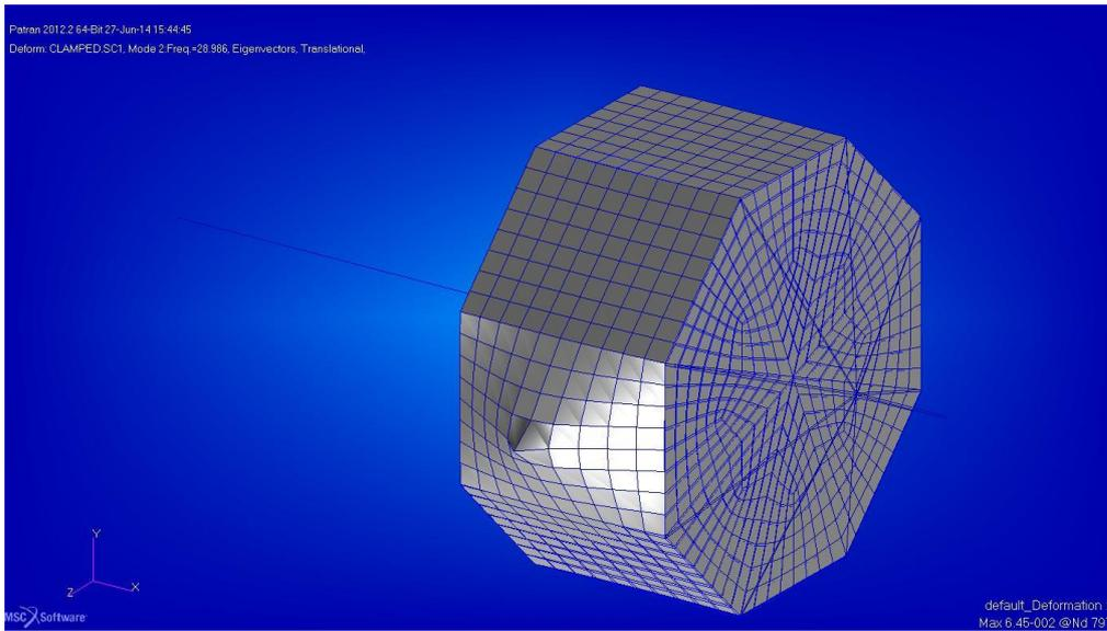
**Figure 11-12: LM lateral CFRP panel mode**
