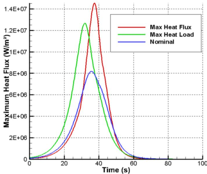
**Figure 19-1: Tot heat fluxes for nominal, max heat flux, max heat load trajectories**
