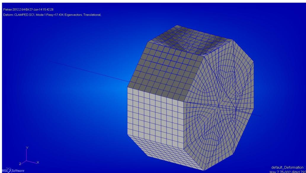
**Figure 11-11: LM lateral aluminium sandwich panel mode**
