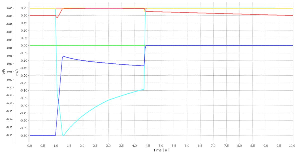
**Figure 13-4: S/C velocities at CoG:  $v_{xo}$  (red),  $v_{yo}$  (blue), and angular speed  $\omega_r$  (light blue). The steep variations during the two crashes are visible**
