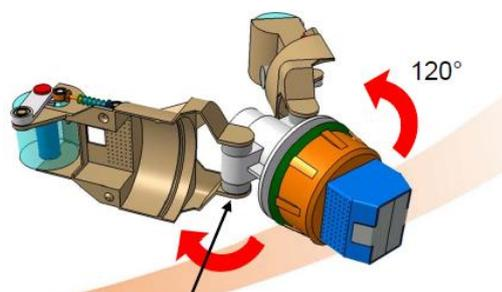
**Figure 13-6: Conceptual representation of the sample container while attached to the sampling device (Airbus DS concept from the Phootprint study). In this example, the bristles open to allow the container to be inserted into the ERC**
