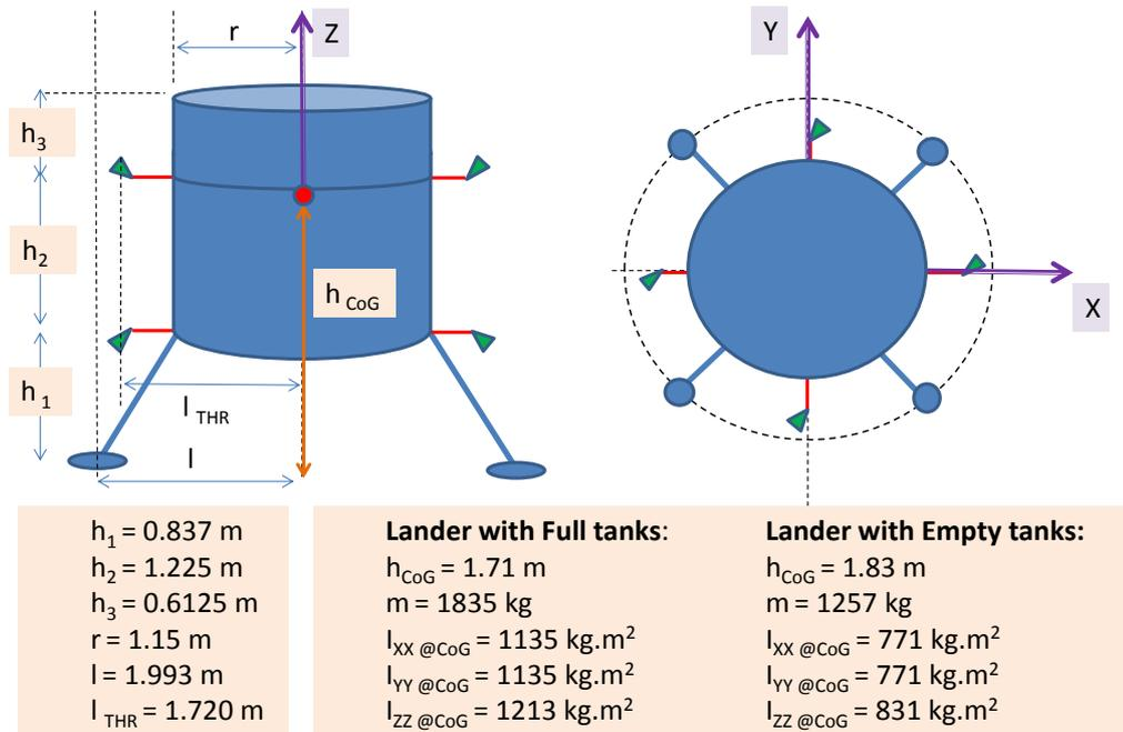
**Figure 15-5: GNC simplified dimensions and MCI of Lander+ERV**
