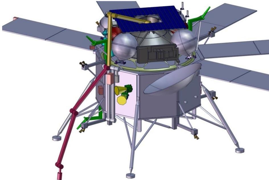
**Figure 10-5: Phobos-SR – LM – 3 configurations of the Robotic arm**
