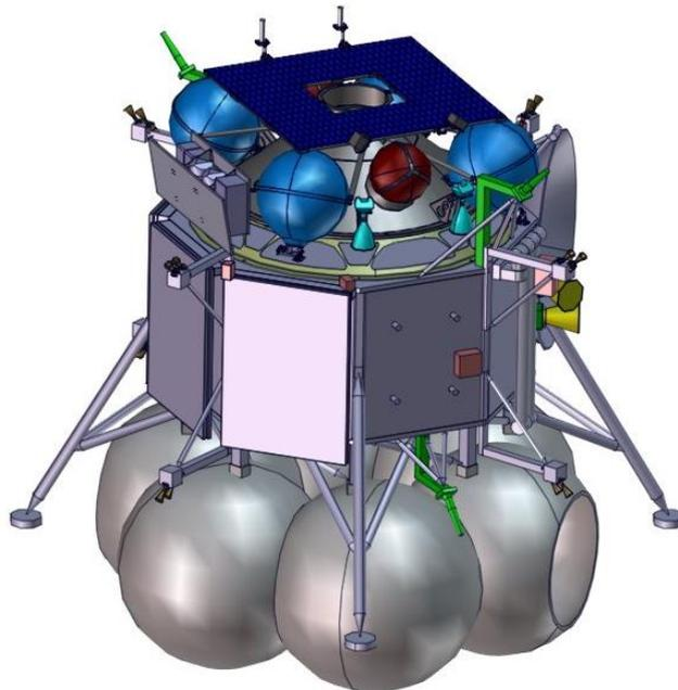
**Figure 8-5 : Phobos Sample Return spacecraft composite**
