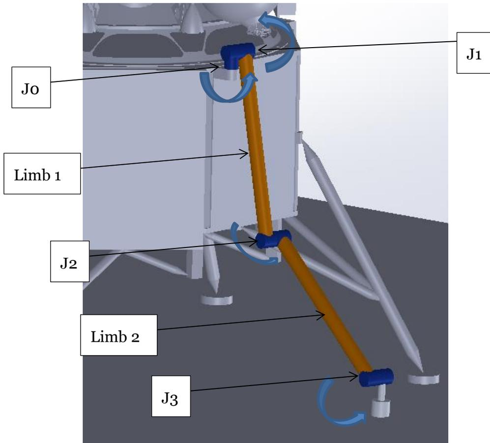
**Figure 12-2: Robotic Arm components**
