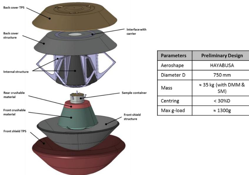
Figure 9-9: ERC preliminary design (ref: Airbus DS Phootprint design)
