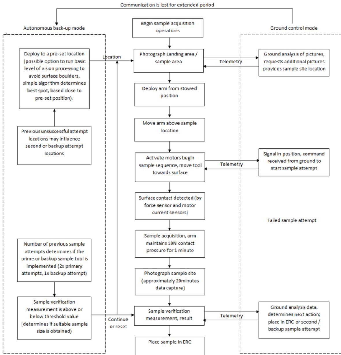
**Figure 12-8: Operations diagram**
