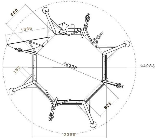
**Figure 10-10: Phobos-SR – LM dimension in stowed configuration – top view**
