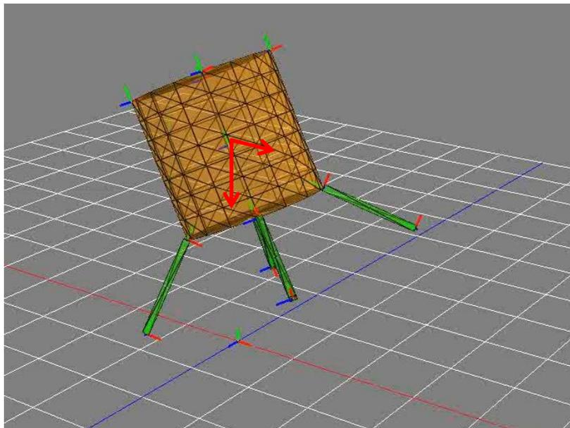
**Figure 13-3: S/C approaching landing in DCAP Multi-body model. Vectors of initial speeds are shown in red**
