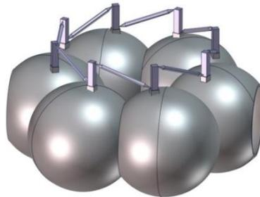
**Figure 10-2: Adapter PM-LM integrated on Fregat upper stage**
