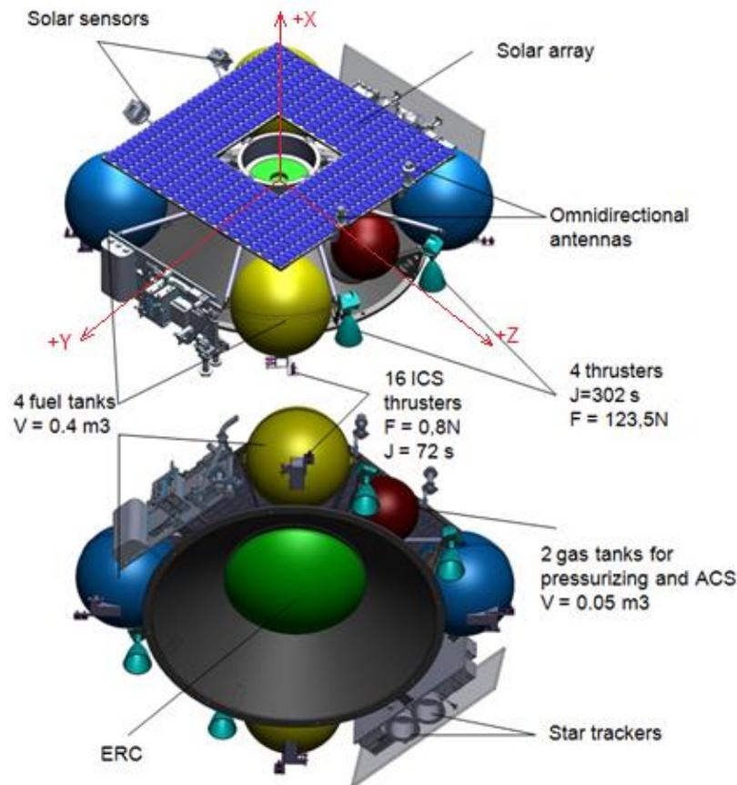
**Figure 7-4: General view of the final ERV design**
