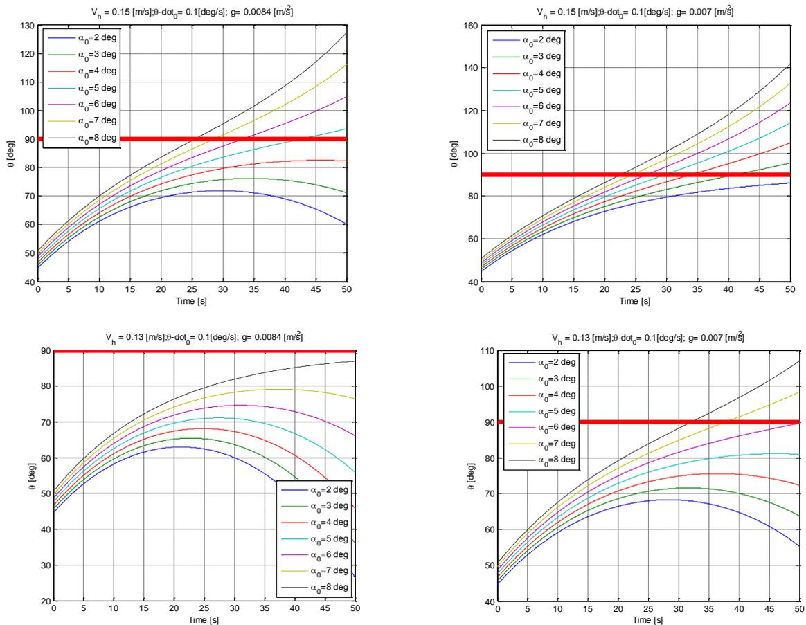
**Figure 15-2: Rotation angle  $\theta$  after touchdown. High surface gravitational level (left) and low surface gravitational level (right). Touchdown lateral speed 15 cm/s (top) and 13 cm/s (bottom)**
