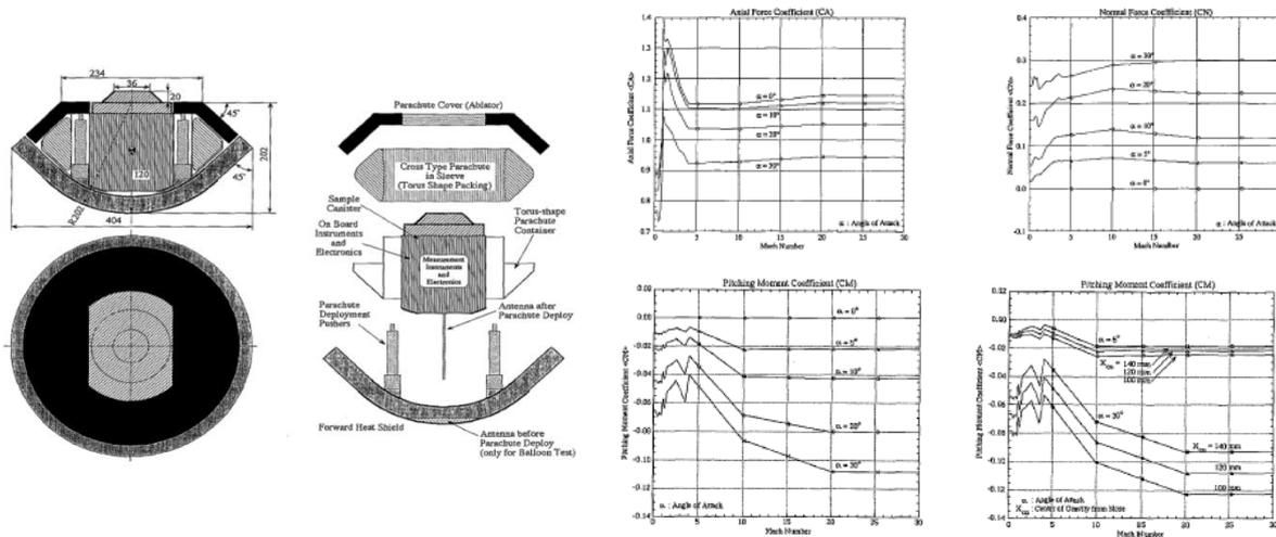
Figure 9-2: Hayabusa geometry and adopted aerodynamic database as in RD[5]
