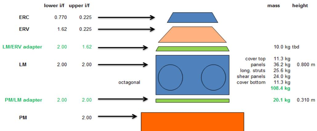
**Figure 11-3: Option B, configuration sketch and mass estimates**
