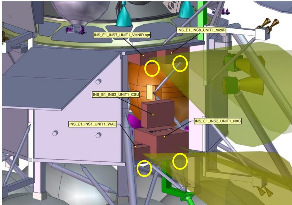
**Figure 10-6: Phobos-SR – LM – PL Field of view**
