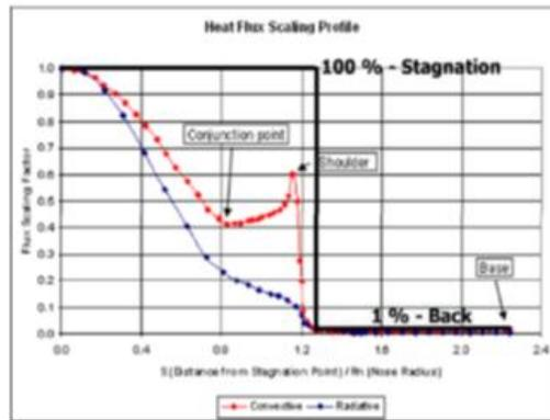
**Figure 19-2: Heat flux evolution between front shield and back cover**
