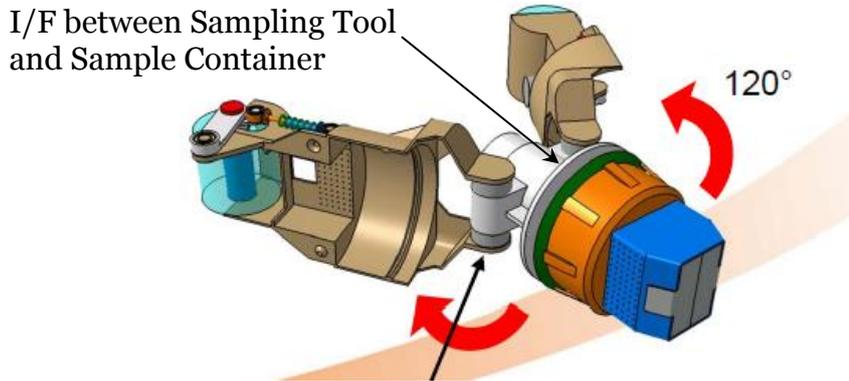
**Figure 24-11: Conceptual design of the Sampling Tool (Airbus DS): opening of the halves to release the Sample Container (in blue)**
