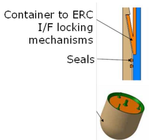
**Figure 13-7: Conceptual representation of the holding interface for the sample container (Airbus DS concept from the Phootprint study). A bayonet-type mechanism is shown in this example**
