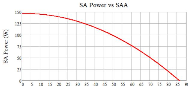
**Figure 16-15: SAR output power vs SAA, for 1 m<sup>2</sup>, June 2024 (1.4 AU)**
