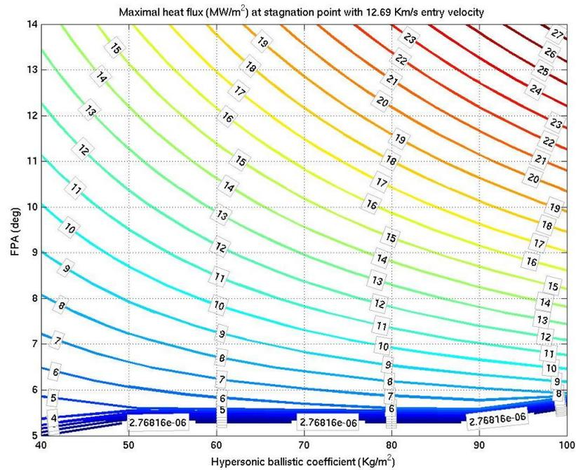
**Figure 9-4: Heat (convective and radiative) flux at stagnation point**
