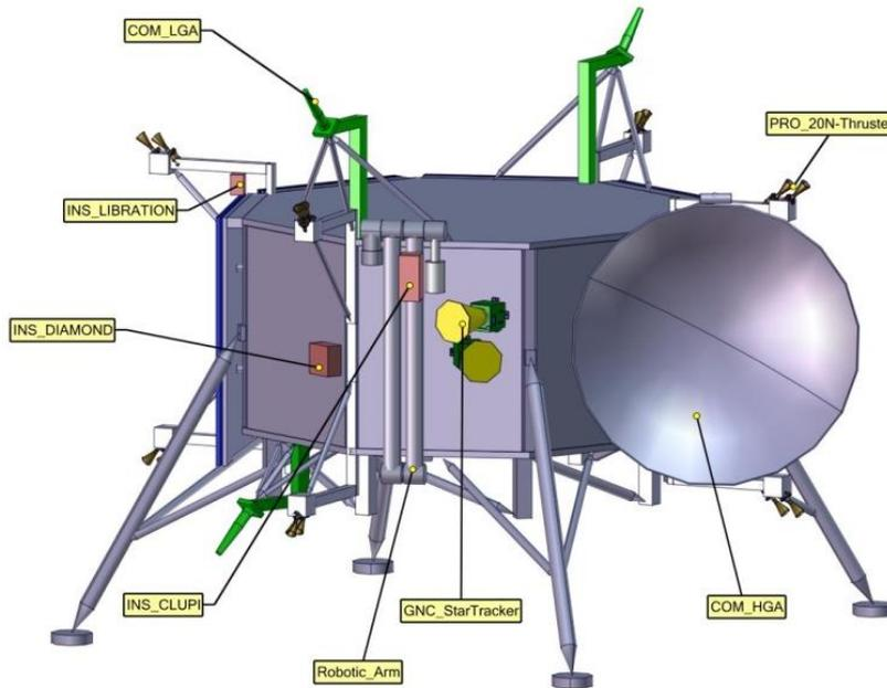
**Figure 10-8: Phobos-SR – LM external accommodation**
