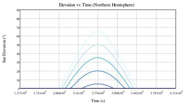
**Figure 16-11: Sun Elevation versus time, for different latitude landing sites (0° to +90° in steps of 15° - May 2024)**
