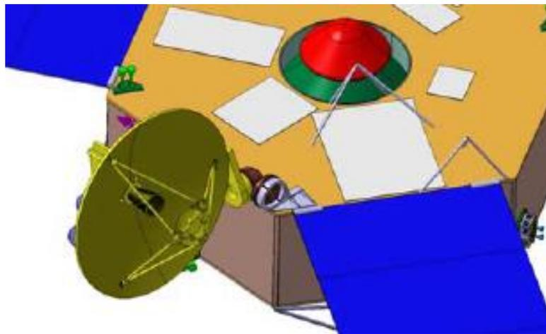
**Figure 13-8: Bepi Colombo high gain antenna pointing mechanism and HDRM**
