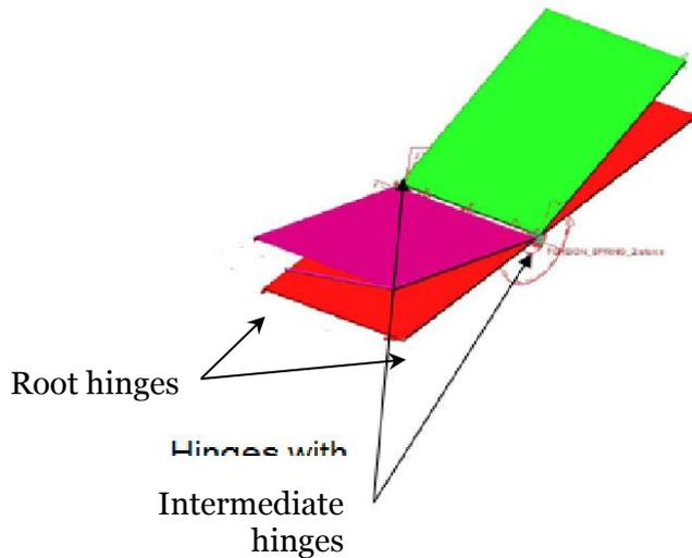
**Figure 13-9: Schematic view of 2 foldable solar panels in one wing and hinges locations**
