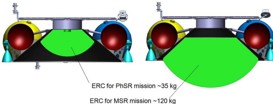
**Figure 7-5: Unified cone-type support for heavy-weight ERC placement**
