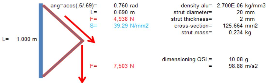
Figure 11-6: LM strut design for tank bipods
