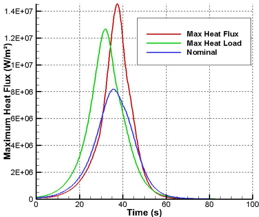
Figure 9-10: nominal, max heat flux and max heat load trajectories (incl. margins)
