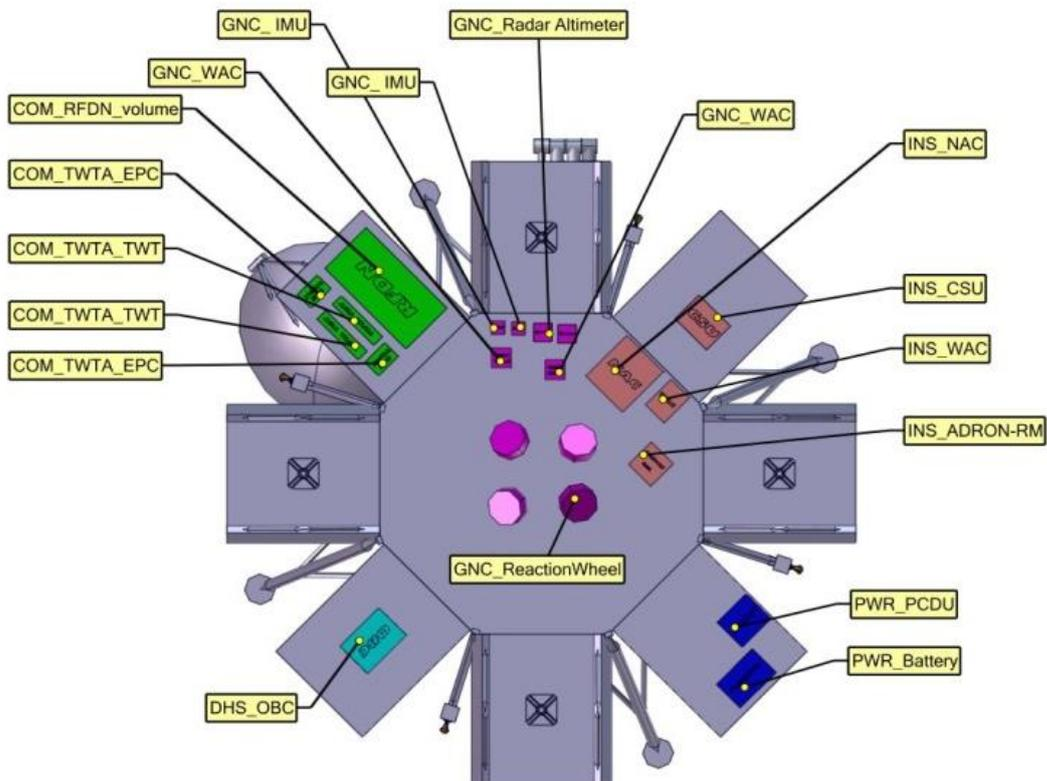
**Figure 10-7: Phobos-SR – LM internal accommodation**
