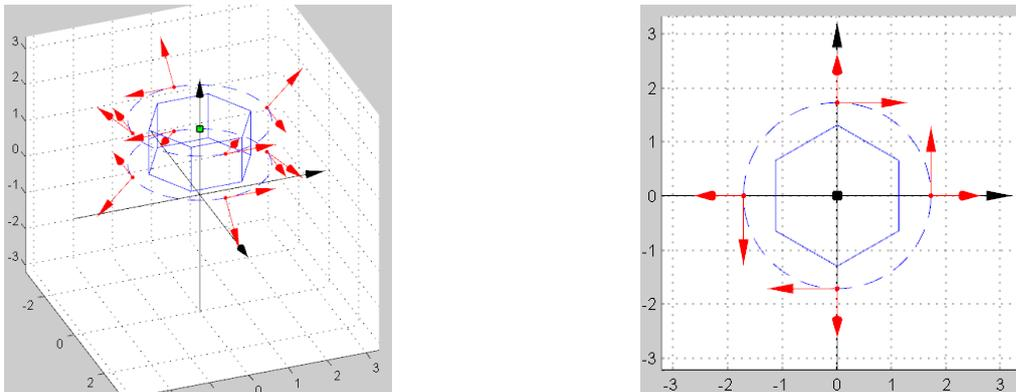
**Figure 15-7: Configurations with 24 RCS: 8x2 ( tilted 45 deg, azimuth 0 deg) + 8 roll thrusters.**
