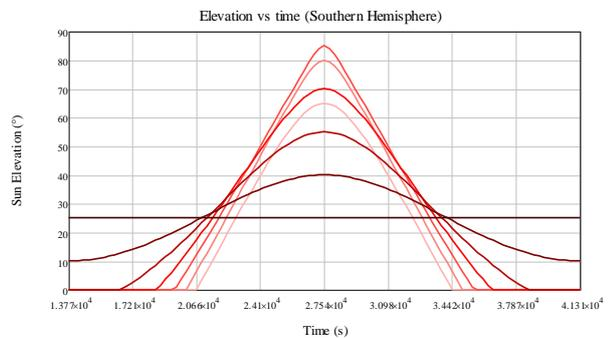
**Figure 16-12: Sun Elevation versus time, for different latitude landing sites (0° to -90° in steps of 15° - May 2024)**
