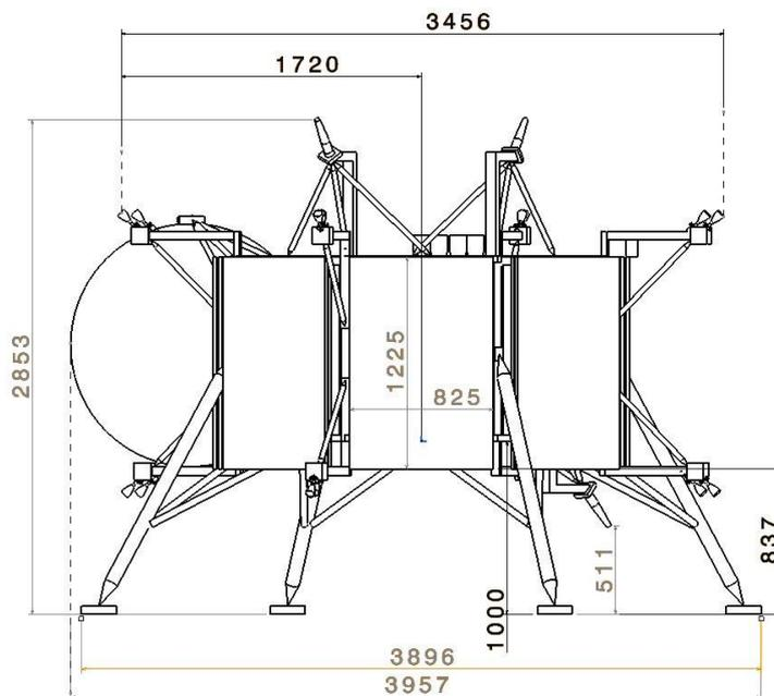
**Figure 10-9: Phobos-SR – LM dimension in stowed configuration – side view**
