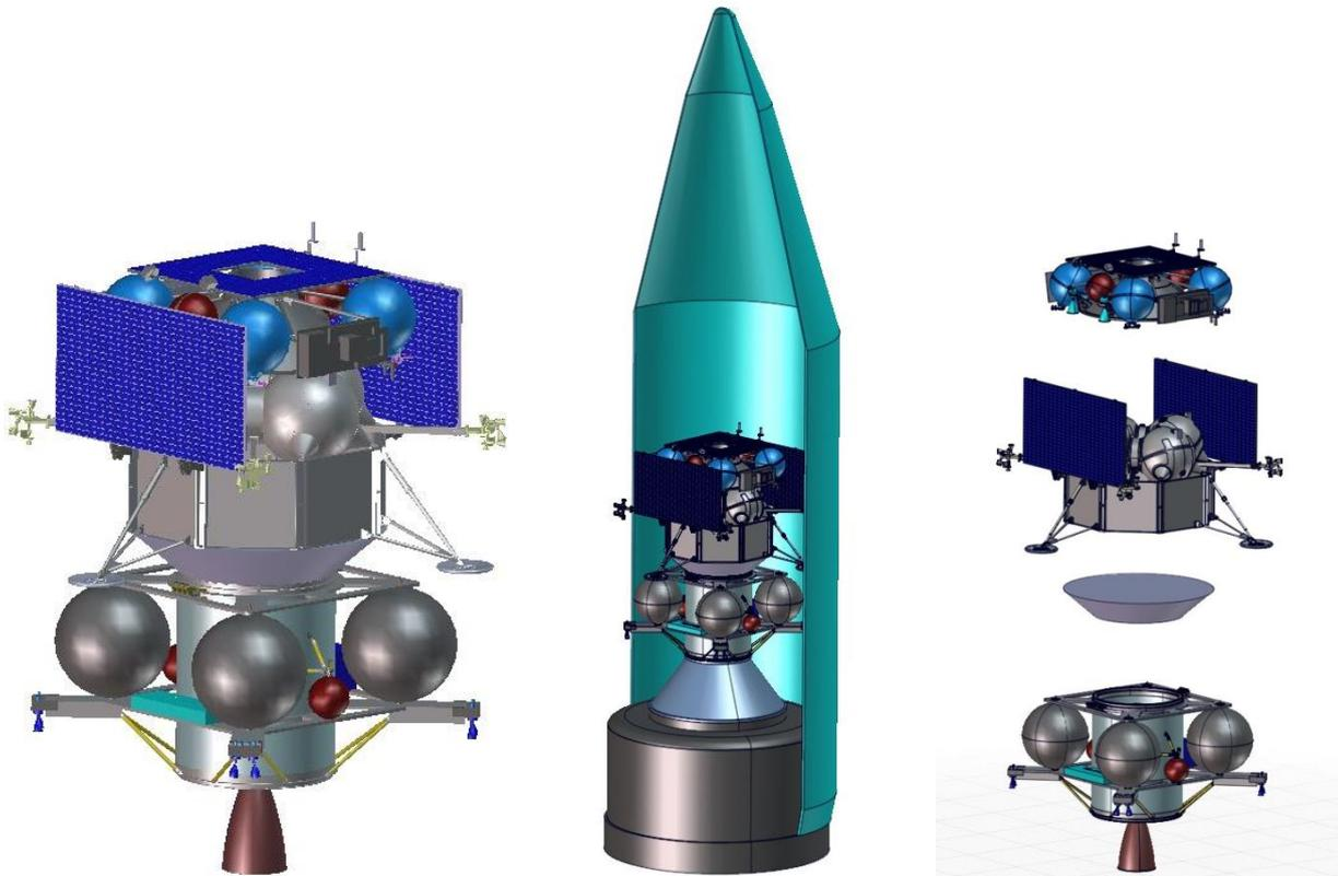
**Figure 8-7 – View of the Phootprint backup cooperation scenario composite standalone (Left), under Proton fairing (Centre) and exploded (Right)**
