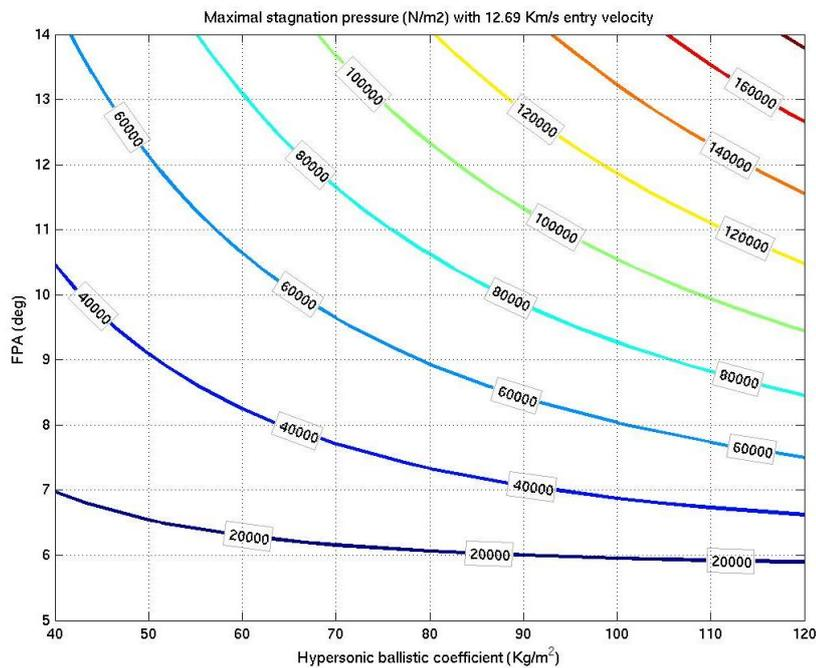
**Figure 9-6: Stagnation pressure (at maximum heat flux)**
