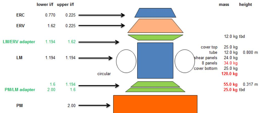
**Figure 11-2: Option A, configuration sketch and mass estimates**
