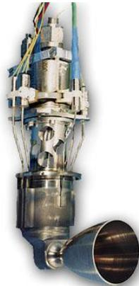
**Figure 14-1: 20 N thrusters with canted nozzle**
