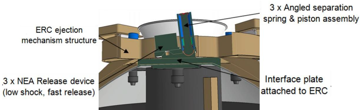
**Figure 13-5: Conceptual solution for the ERC SED. The structure of the ERV which holds the ERC is located on the top, and the ERC hung under it**
