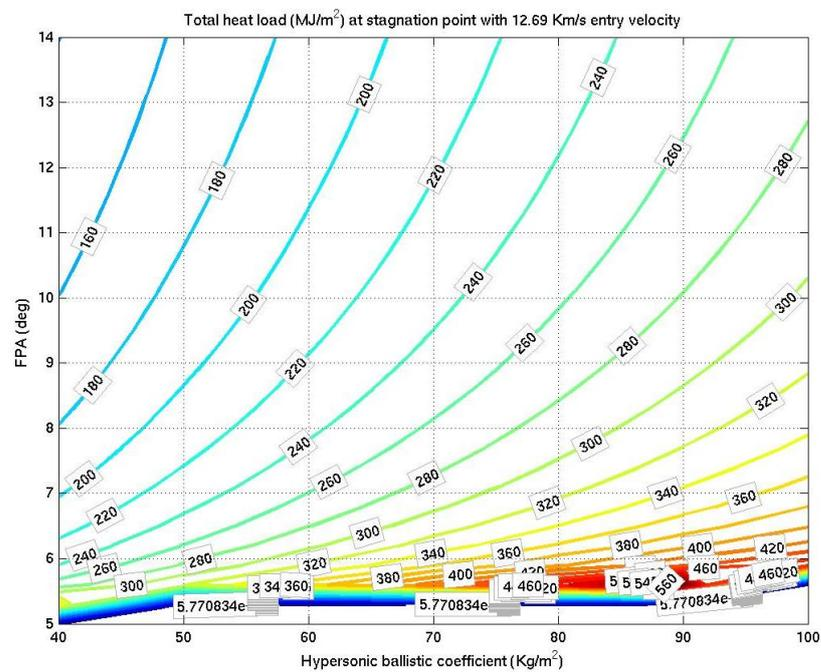
**Figure 9-5: Integrated heat load (at stagnation point)**
