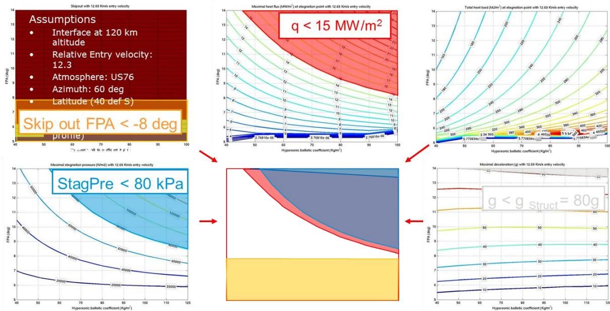
**Figure 9-8: Feasible domain definition (bottom centre picture indicated by the white area)**
