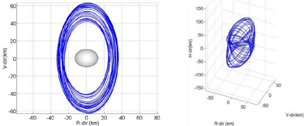
**Figure 15-3: QSO width 28x44 km, 60 deg inclination (from RD[18])**
