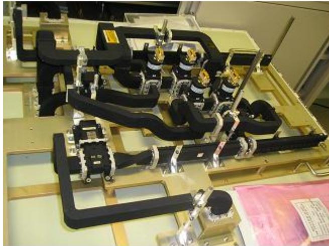
**Figure 15-11: Example Radio Frequency Distribution Unit**
