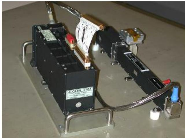
**Figure 15-5: Travelling Wave Tube Amplifier**
