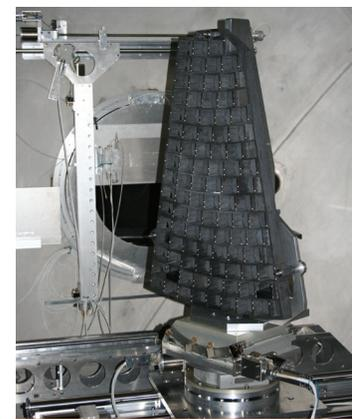
Silicon Pore Optics mirror structure (breadboard)
