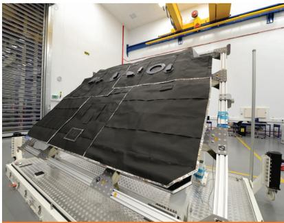
Structural and thermal model of heat shield for Solar Orbiter
