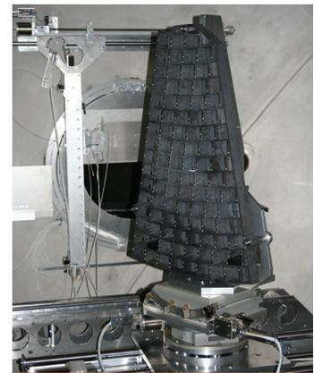
Silicon Pore Optics mirror structure (breadboard)
