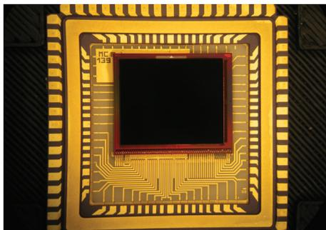
Near-infrared detector (breadboard)
