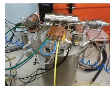
15K pulse tube cooler (breadboard)
