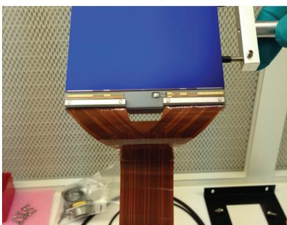
CCD 270 developed by e2v for PLATO
