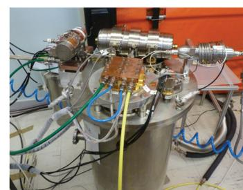
15K pulse tube cooler (breadboard)
