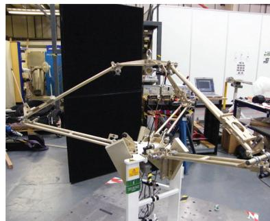
Deployable mast (breadboard)
