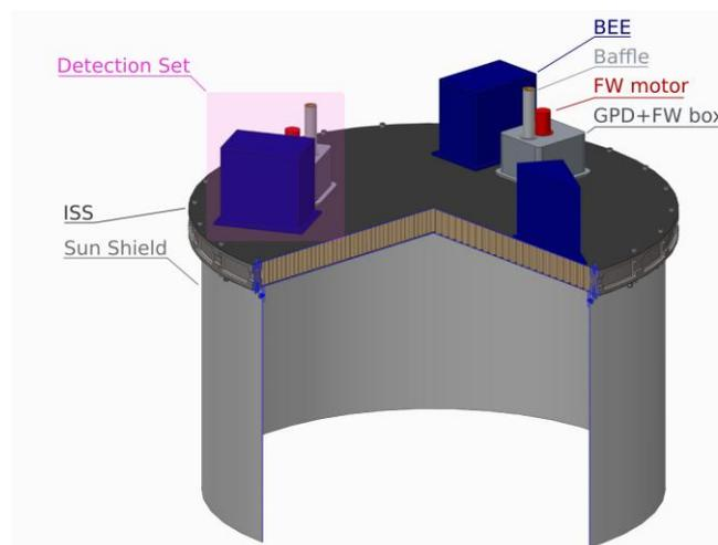
Figure 32 Accommodation of the DSs on the FPA.
