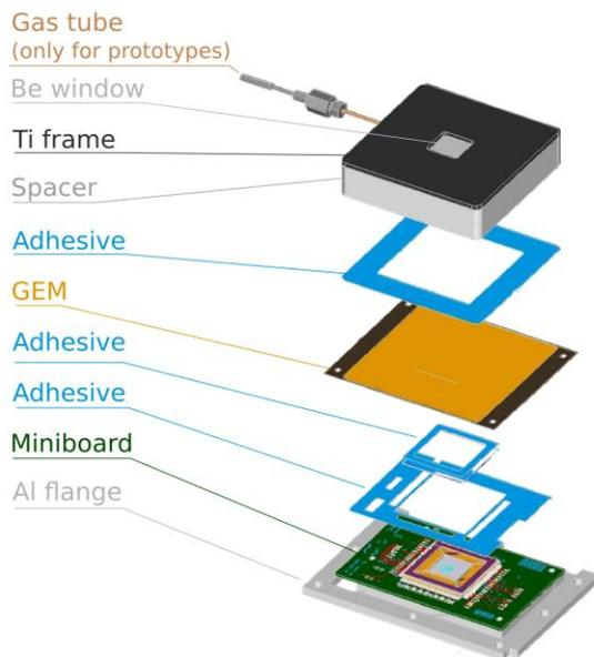
Figure 26 Exploded view of the GPD.
