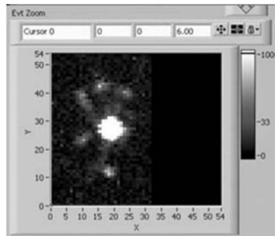
Figure 30 Track generated by a Fe ion with an energy of 500 MeV/nucleon shown by the online monitor during the irradiation test. The dimension of each pixel is  $50 \mu\text{m}$ . The event saturates the electronics in a 5 pixels radius. Several delta rays are also visible (Bellazzini et al. 2010).
