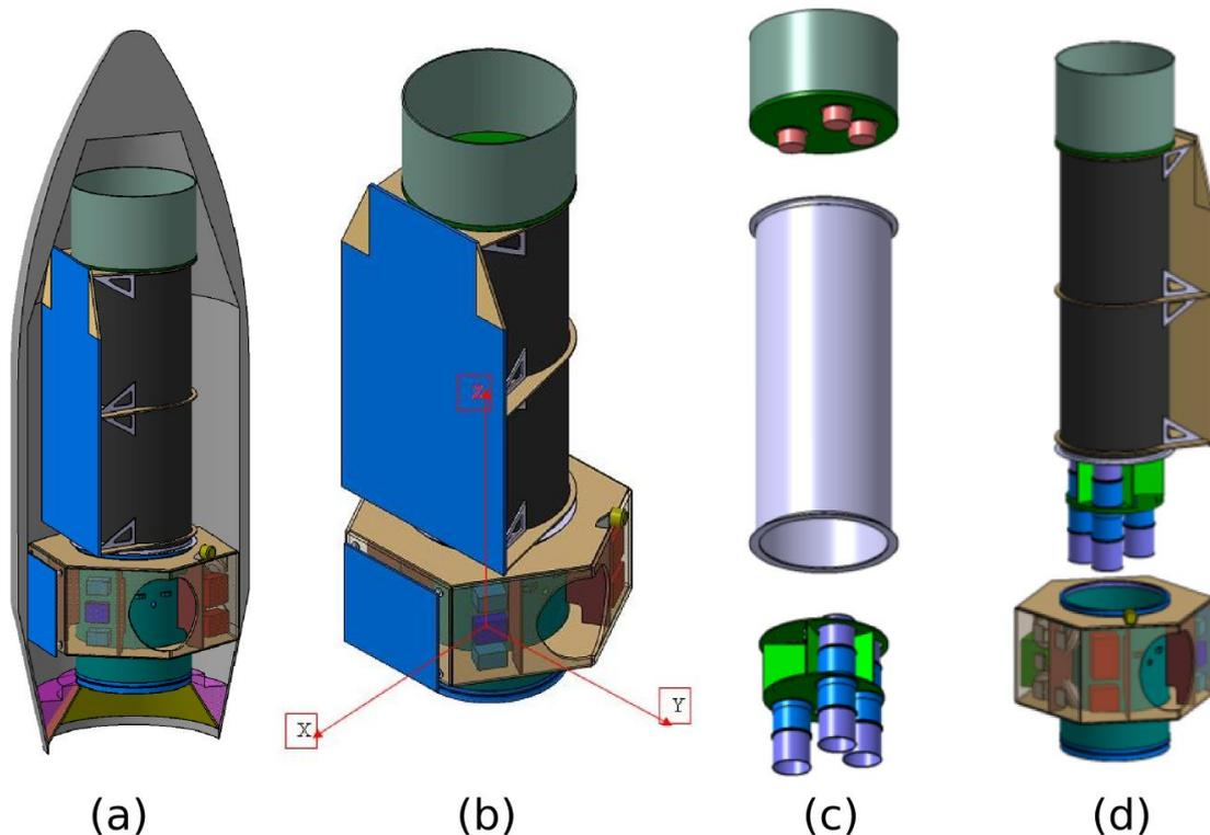
Figure 39 (a) XIPE in the Vega fairing. (b) The complete spacecraft with fixed solar panels. (c) The three main elements of XIPE (Focal plane assembly, the telescope supporting structure and the mirror assembly (the control electronics are hidden from view). (d) The plug&play approach with SVM (below) and P/L and telescope supporting structure (above).
