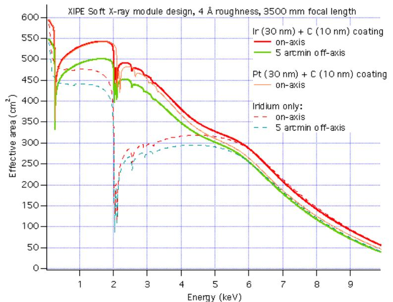
**Figure 16 Effective area of a single XIPE mirror module, on-axis (red lines) and 5 arcmin off-axis (green lines). The computations without the Carbon over-coating are shown as dashed lines, and return a much lower effective area. The computed effective area assuming a Pt +C coating (yellow line) differs only a little from the Ir+C coating.**
