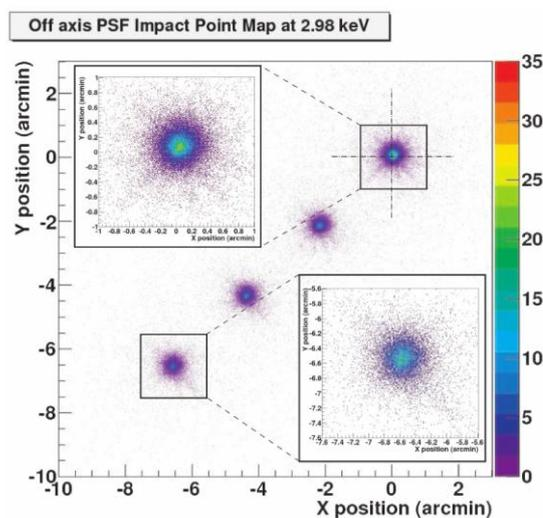
Figure 20 (Left) Image of three 4.5 keV pencil beams (spot size of a few tens of microns) shifted by 300 μm in the X and Y directions. The measured HEW is 92 μm (from Soffitta et al. 2013, Fabiani et al. 2014). (Right) Point Spread Function of the GPD in the focus of a JET-X mirror module at 2.98 keV (Fabiani et al. 2014).
