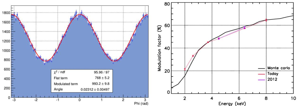
Figure 22 (Left) Modulation curve at 3.7 keV. The measured modulation factor is 41% even without any data selection. (Right) Modulation factor measured for the GPD as a function of the energy, assuming a cut of 20% of data selected on the basis of the elongation of the track. The measurements carried out in 2012 are consistent with those performed two years later. The measurements are also compared with the result of a Monte Carlo.
