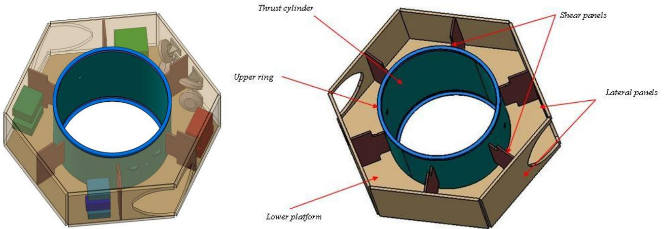
Figure 40 (Left) Overview of the SVM internal configuration. (Right) the SVM structure assembly without top panel.
