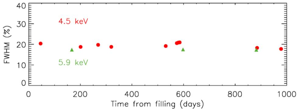
Figure 27 Energy resolution of the GPD FOR nearly 3 years at different energies (Soffitta et al., submitted).
