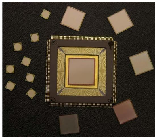
Figure 18 The three ASIC generations, with increasing pixel number and decreasing pixel size, at the basis of the Gas Pixel Detector (Bellazzini et al. 2006).
