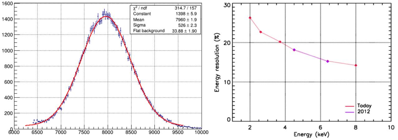
Figure 23 (Left) Spectrum of 6.4 keV photons. The measured energy resolution is 15.5%. (Right) Energy resolution as a function of the energy measured for the GPD in 2012 and today.
