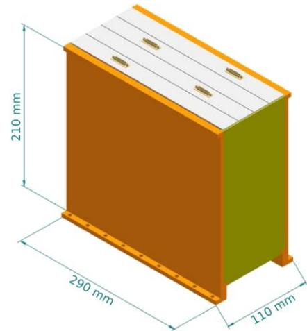
Figure 34 Sketch of the CE with its dimensions.
