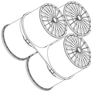
**Figure 14 Mirror Modules assembled in the Mirror Support Structure.**
