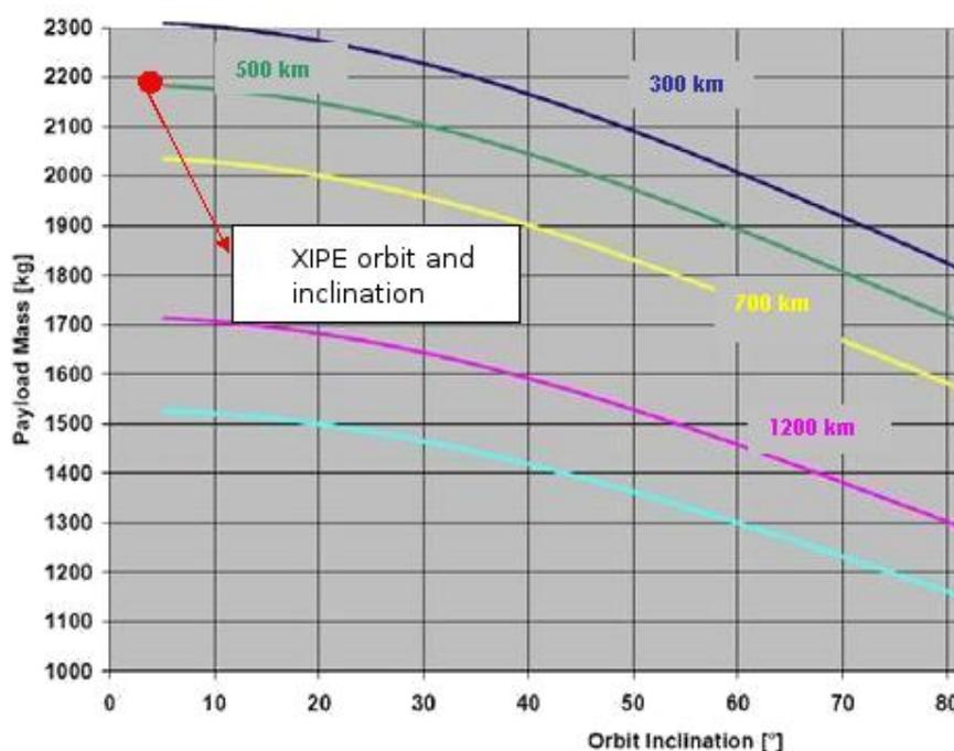
Figure 36 LV (Launch Vehicle) performance for the nearly circular orbits of XIPE. The XIPE dry mass (including margins) is 877 kg (see Section 5.22.2).
