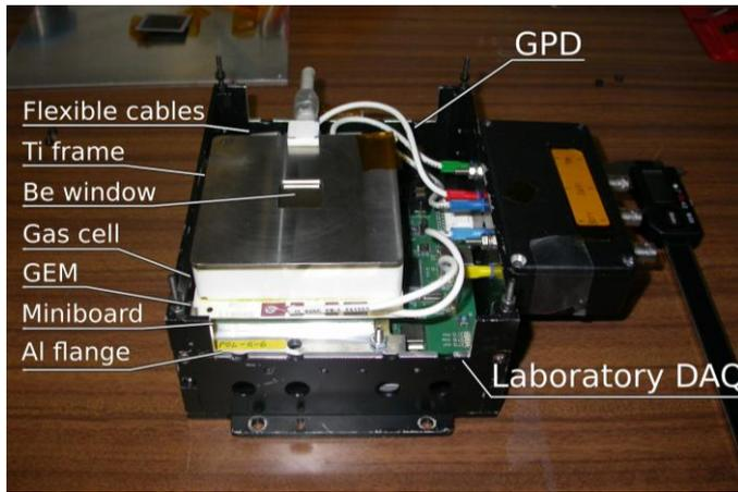
Figure 25 The current version of the GPD, together with the BEE (Laboratory DAQ) used in the laboratory.
