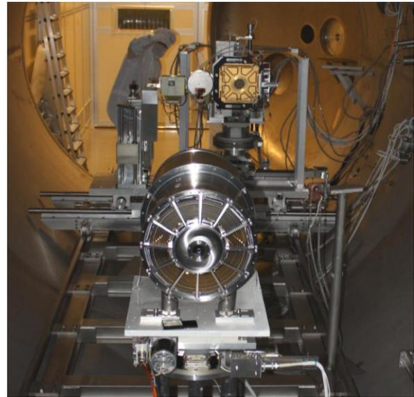
Figure 29 The GPD inside the vacuum chamber (on the left in the background) at the PANTER X-ray testing facility with the flight spare model of the JET-X telescope.
