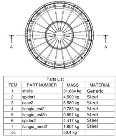
**Figure 15 Technical drawing of the XIPE MM. The weight is 50.4 kg (without margins).**
