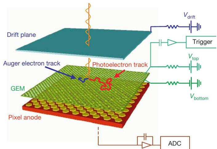
Figure 17 Principle of operation of the GPD (Costa et al. 2001).
