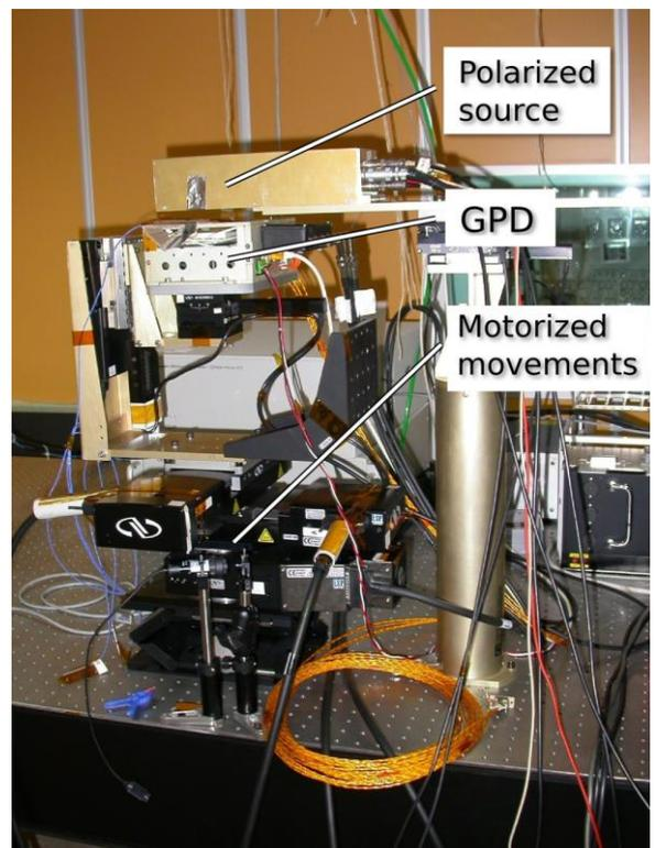
Figure 35 The GPD in the test facility at INAF-IAPS.
