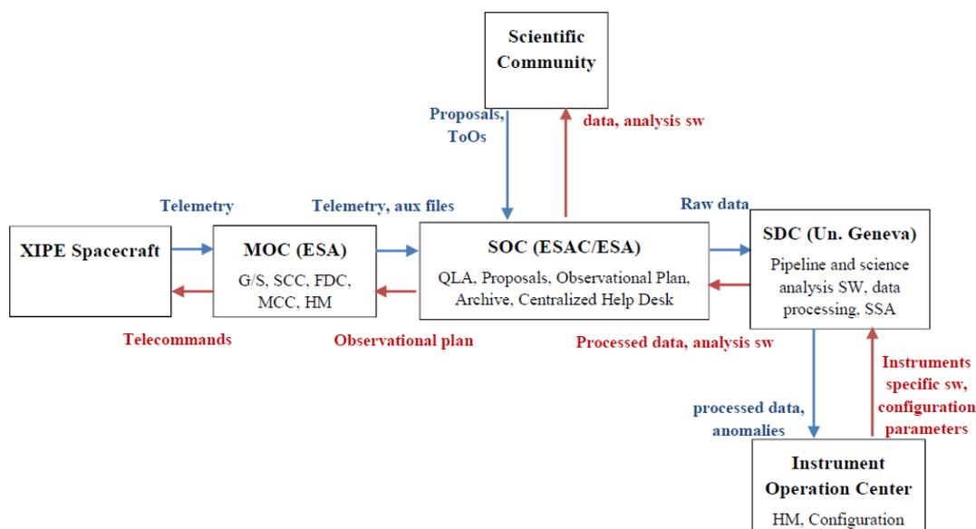
**Figure 45 Block diagram of the Ground Segment and User Segment.**
