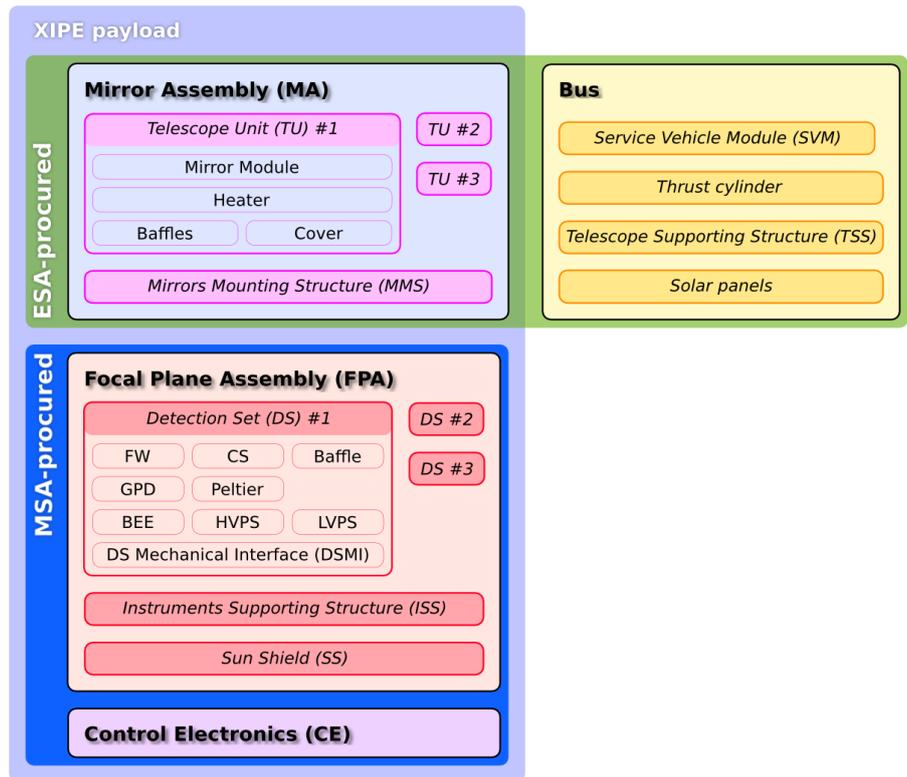
Figure 12 Block diagram of the XIPE scientific payload.
