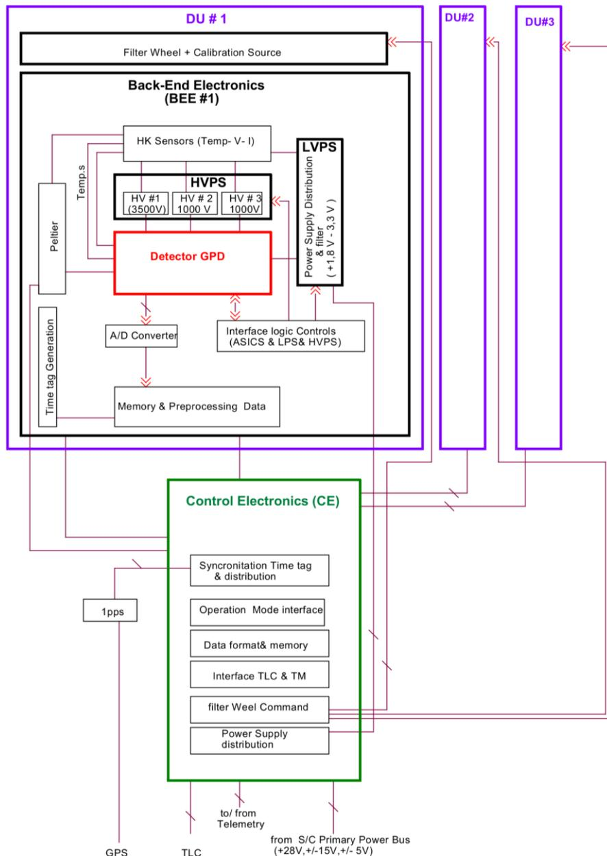
Figure 33 Functional diagram of the FPA and of the CE.
