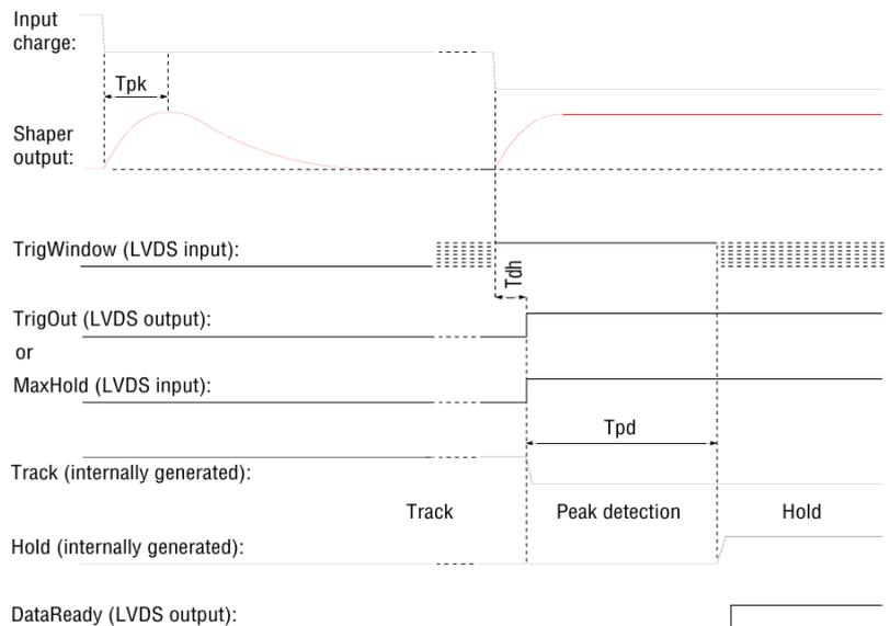
Figure 24 ASIC internal sequence for the capture of an event.
