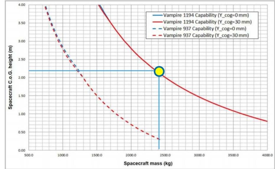
Figure 4.2.3.1.1.a – Limits of spacecraft C.o.G. position vs. spacecraft mass for single launch configuration in case of "VAMPIRE 937" or "VAMPIRE 1194"
