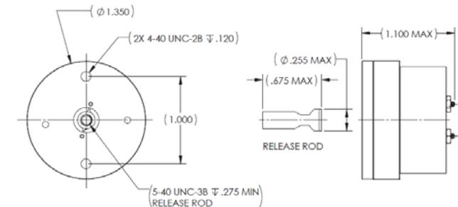
Note: Model 9100 Release Mechanism shown. Different configurations available with alternate release rods, mounting features, and connectors. Metric configurations are also available.
