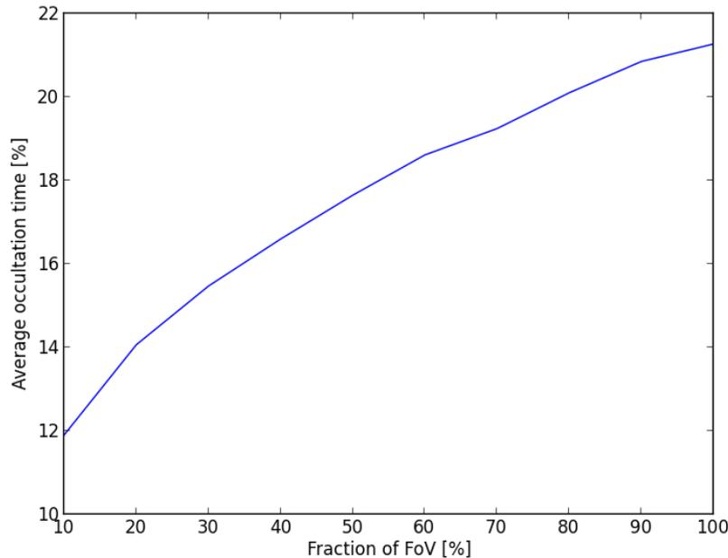
The trend is obtained reducing the FoV area of XGIS while keeping fixed its shape (rectangular).
