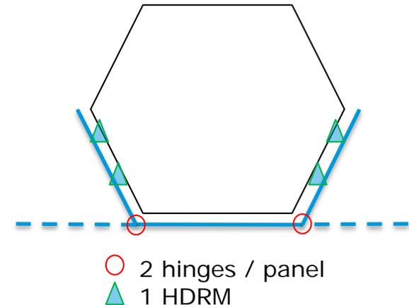
These hinges need to be customized as the solar panel open with an angle of 60deg.
