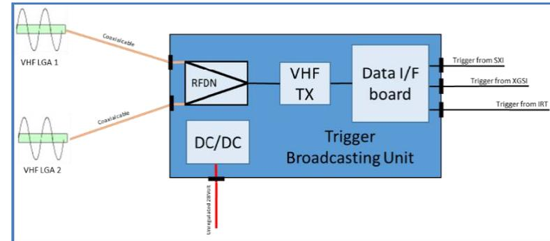
Figure 20: general block diagram of the Trigger Broadcast Unit
