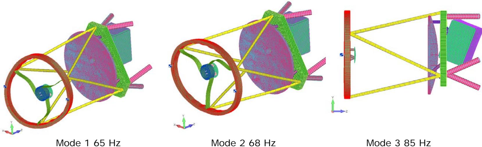
Eigenmodes 1 and 2 dominated by bending and torsional response of Upper Cage and M2 Spider.
