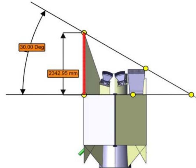
Requested solar area (fixed) = 10m<sup>2</sup> with reduced factor of 50% for angled side panel
