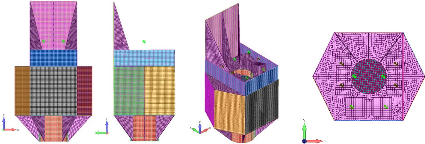
Instruments (XGIS,SXI), Propellant Tanks, cryocoolers added as lumped masses = 530 Kg
