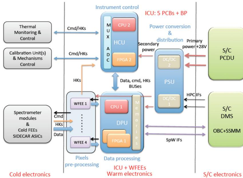
Figure 4-13: EChO payload electrical architecture block diagram (baseline solution).
