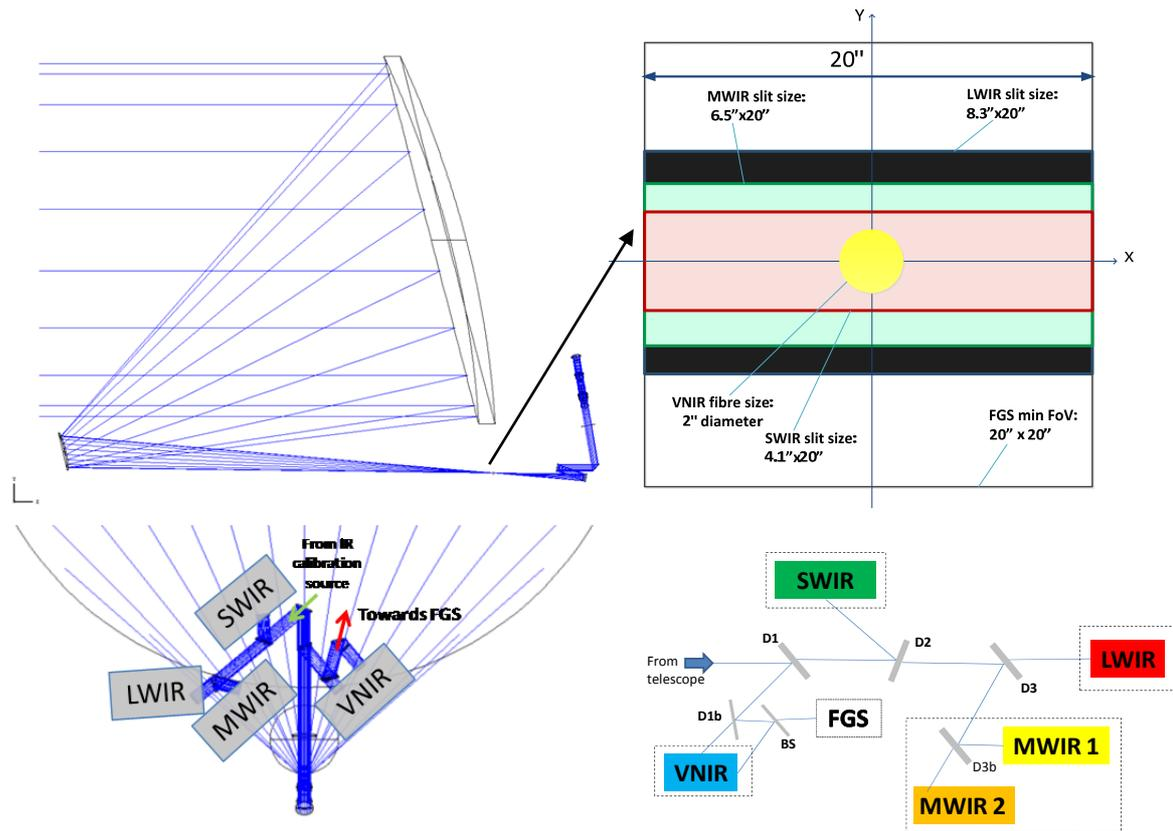
Figure 4-6: Both upper and lower left: optical layout of the EChO front and common optics concept. Upper right: the relative size, nominal position and orientation of the different spectral modules' fields-of-view at the telescope intermediate focus are indicated. Lower right: schematic of channel division by dichroics
