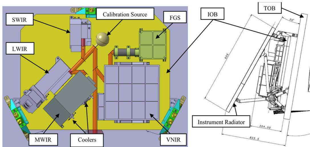
Figure 4-9: Left: chosen layout of the optical modules. Right: MICD extract showing dimensions and location of instrument dedicated radiator
