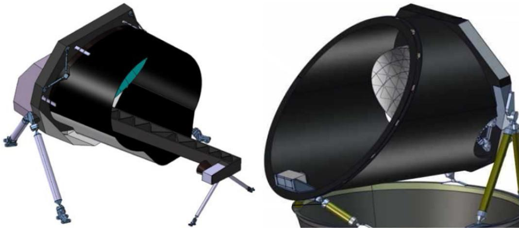
Figure 4-4: Telescope Optical Bench and baffle. Left: Industry A. Right: Industry B.
