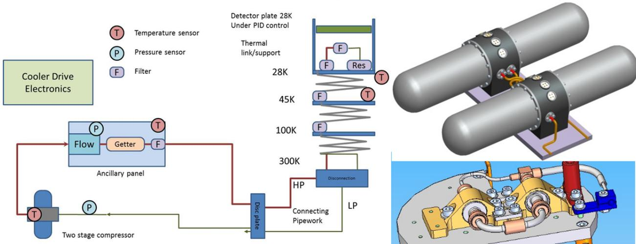
Figure 4-12: Active Cooler System. (left) system schematic, (right top) Four-stage compressor designed for ESA 2K cooler contract as evolution from Planck design - EChO would use half use of this; (right bottom): Final stage filter, J-T expansion valve and heat exchanger CAD model.
