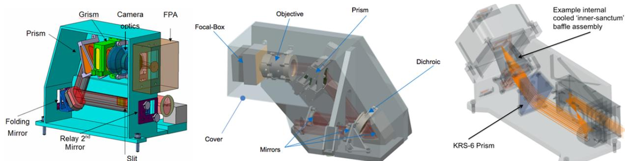
Figure 4-15: (left) SWIR Channel Optical Module design; (centre) MWIR Channel Optical Module Design; (right) LWIR Channel Optical Module design
