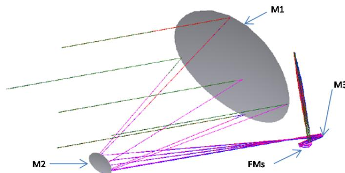
Figure 4-3: Telescope design, showing M1, M2, M3 and the Fold Mirrors (FMs) – Industry B
