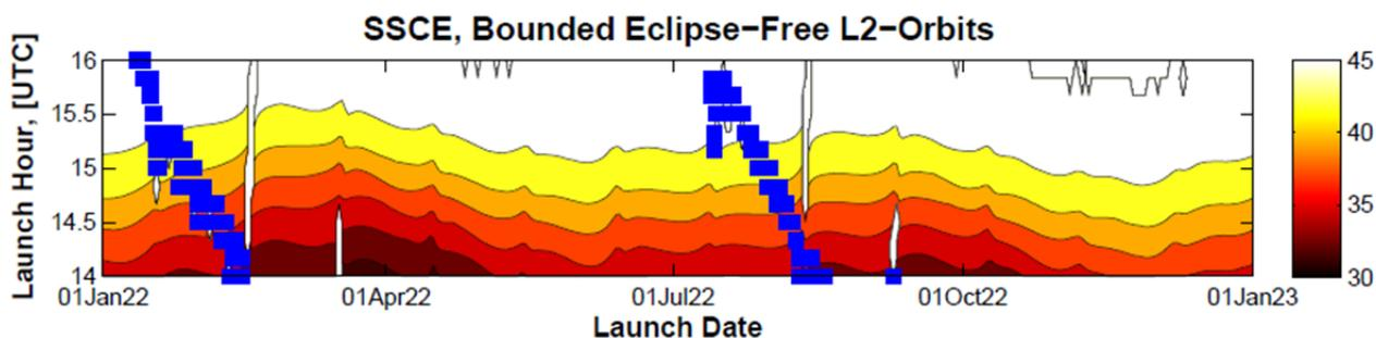
Figure 6-5: EChO launch window, showing daily launch windows between 14:00 and 15:30 UTC apart for 2x 1 month outages around both equinoxes (blue area). The later the launch time, the larger the amplitude of the orbit around L2 (dark red to yellow for Sun-S/C-Earth angle from 30 degrees to 45 degrees respectively).
