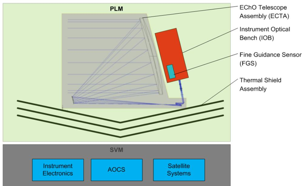
Figure 4-1: Simplified block diagram of the EChO spacecraft system
