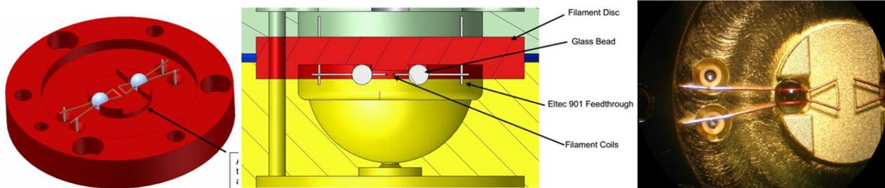
Figure 4-7: Common Calibration Unit: The two redundant filaments are shown at the centre of the assembly. The glass beads which achieve mechanical bonding of the filaments are also visible.
