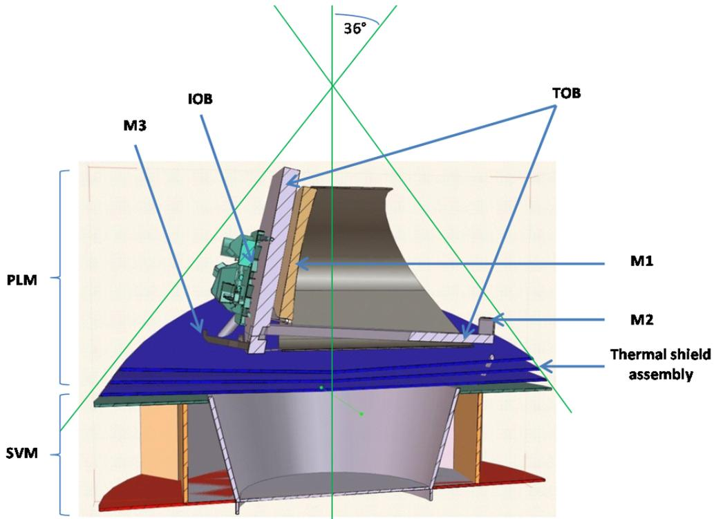
Figure 6-2: Cross-section of EChO showing the main structural elements within the PLM and the angular constraints imposed by the observable sky requirement
