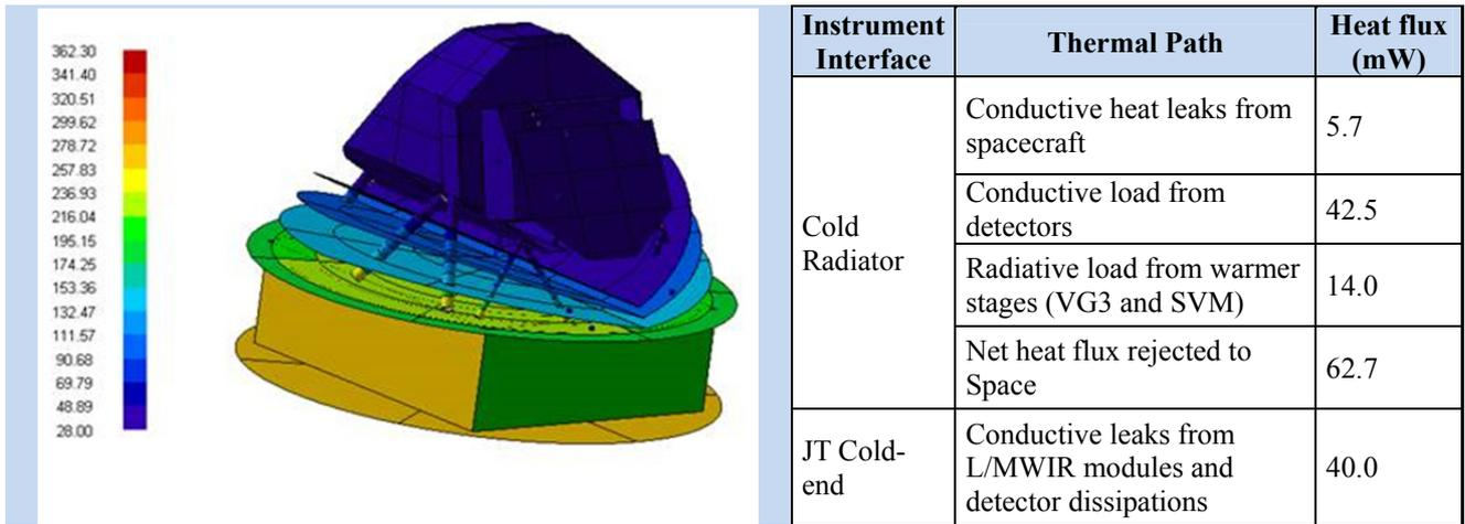
Figure 4-11: Results of coupled S/C, PLM and Instrument thermal models – (left) temperature map, (right) predicted heat fluxes at instrument main thermal interfaces
