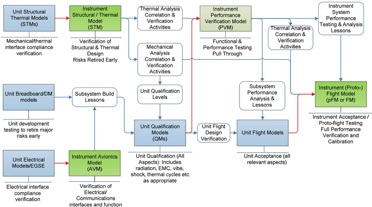
Figure 4-16: General verification flow for the EChO Instrument programme. Blue boxes represent subsystem level hardware activities, Green boxes are instrument level hardware models (only the bright green are delivered onwards to ESA / Spacecraft), Red lines represent hardware deliveries, Blue lines are information or specification flow.
