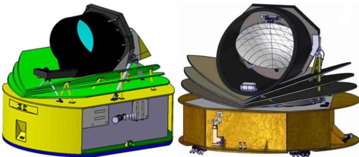
Figure 6-6: EChO S/C, with SVM on the bottom and PLM on the top. Left: Industry A. Right: Industry B.
