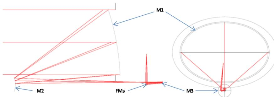
Figure 4-2: Telescope design, showing M1, M2, M3 and the Fold Mirrors (FMs) – Industry A
