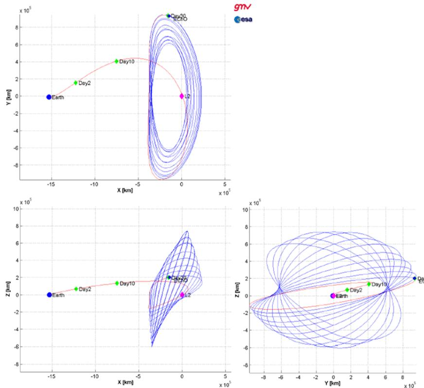
Figure 6-3: Example of EChO orbit around L2
