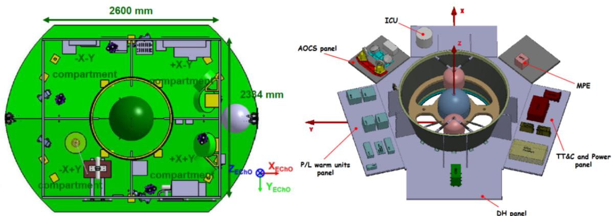
Figure 6-7: Inside view of the EChO SVM. Left: Industry A. Right: Industry B.
