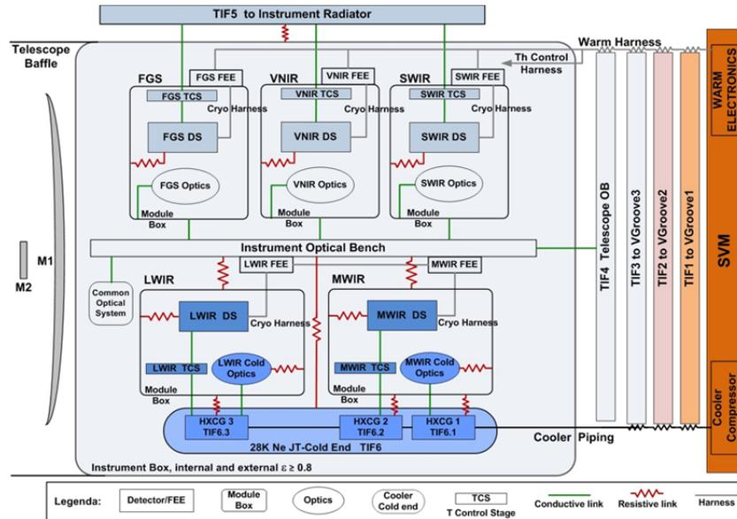
Figure 4-10: EChO thermal scheme with main thermal interfaces to S/C
