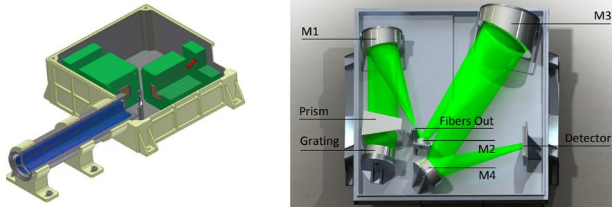
Figure 4-14: (left) FGS Optical Module design including Gregorian telescope, beamsplitter and two redundant detector modules; (right) VNIR Optical Module spectrometer design.
