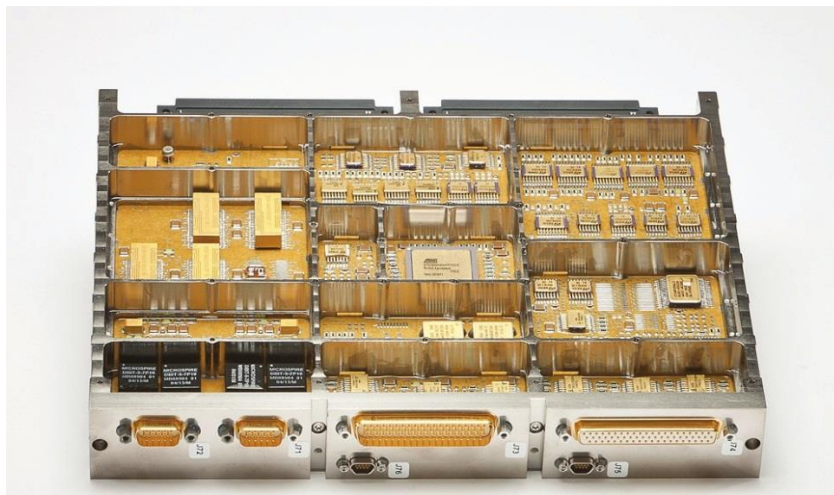
Figure 5: RUAG processing board unit. The “Panther” board provides a LEON core with FPU, cache and additional amenities.
