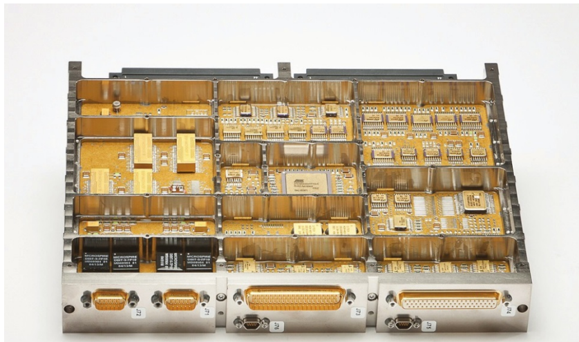
Figure 14-10: RUAG processing board unit. The “Panther” board provides a LEON core with FPU, cache and additional amenities.
