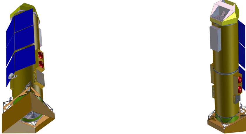
Figure 5.10. Preliminary Athena design by the first industry contractor. The fixed metering structure has a cylindrical section, while the solar arrays are body-mounted. The telescope sun shield is supported by a dedicated frame at the bottom of the central cylinder.
