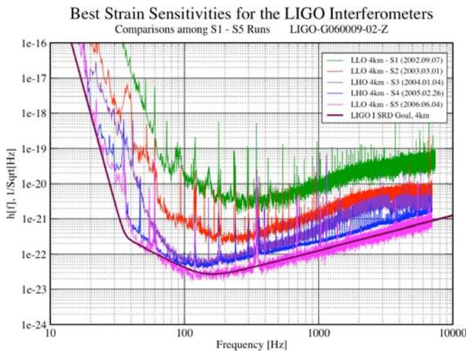
made to bounce several times along cavities in each arm, enhancing the phase-accumulation effect). The free fall of interferometer components is approximated, along the “sensitive” axes, by suspending them from pendulums that are carefully isolated from the environment.
