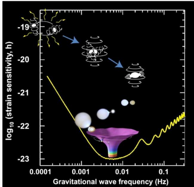
**The LISA strain sensitivity curve showing approximate frequency range and strain amplitude of three categories of sources: massive black hole inspiral, ringdown, and merger (uppermost source); ultra-compact Galactic binaries (middle source); capture of stellar mass compact object by massive black holes (lower source).**
