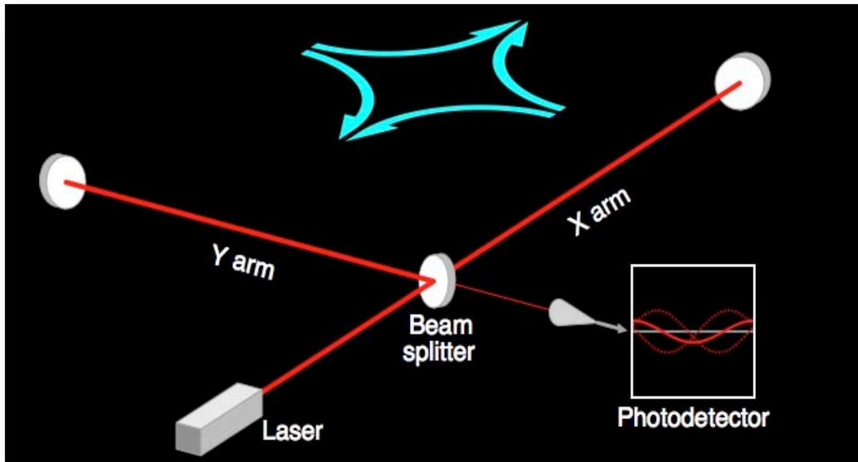
**Figure 1-3:** Idealized Michelson interferometer with laser, beam splitter, end mirrors, and photodetector at the exit port. the blue arrows represent a perpendicularly propagating, linearly polarized gravitational wave.
