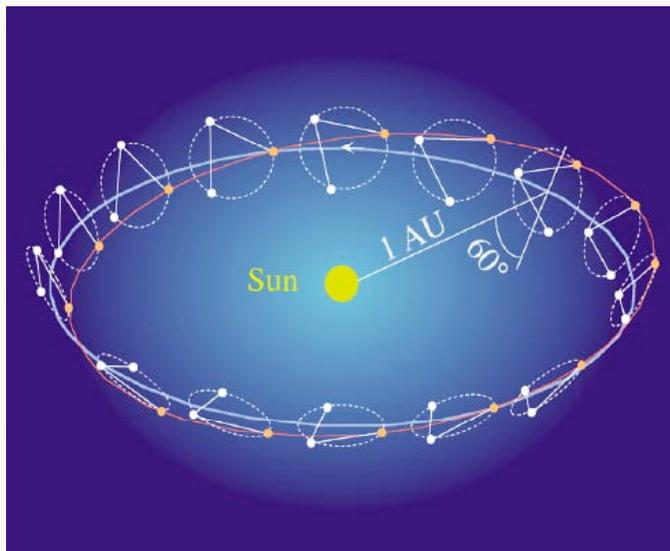
**Figure 2-2: The LISA constellation's heliocentric 1-AU-radius orbit, with the plane of the triangle inclined at 60° to the ecliptic. The triangle appears to rotate once around its center in the course of a year's revolution around the Sun.**
