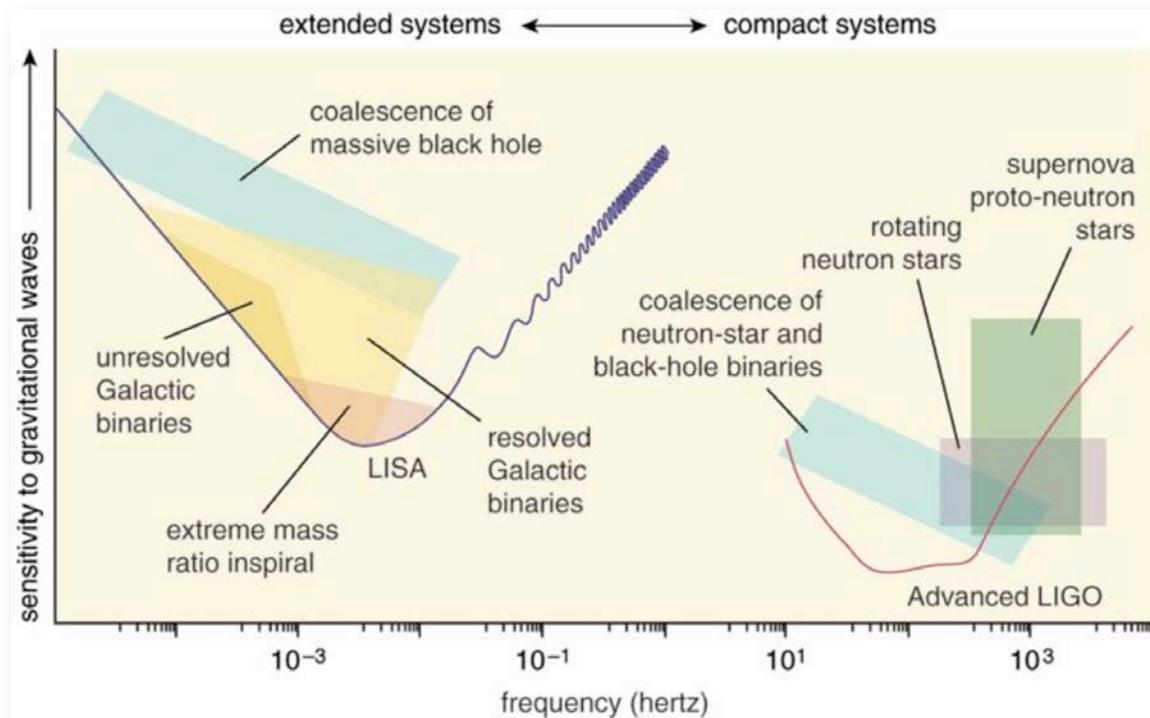
**Figure 2-5: Strain sensitivities predicted for LISA and Advanced LIGO.** The curve is plotted in units of  $(\sqrt{fS_h(f)})$ , where  $S_h(f)$  is the LISA noise power spectrum with  $\sqrt{S_h(f)}$  representing the 1- $\sigma$  noise level. The units of  $(\sqrt{fS_h(f)})$  are the natural units for plotting sensitivity per logarithmic frequency interval.
