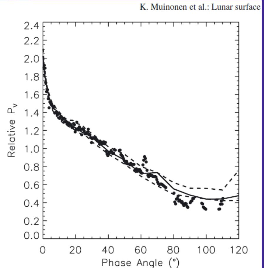
**Fig. 7.** The binned lunar mare volume-element phase function with the corresponding coherent-backscattering modeling including a variation envelope. Double H-G single-scattering phase functions for the fundamental scatterers give rise to coherent-backscattering peaks capable of matching the observations. For the largest phase angles, there is a deviation between the model and the observations potentially due to simplified modeling.
