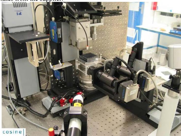
Figure 5 The laboratory robotic system used for demonstrating the stacking techniques for ribbed Si plates. Image courtesy Cosine Research.
