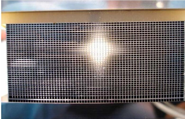
*Figure 7 Assembled stack located in measurement jigs prior to scanning tests at the PTB laboratory int BESSY. This particular stack comprises 35 plates*
