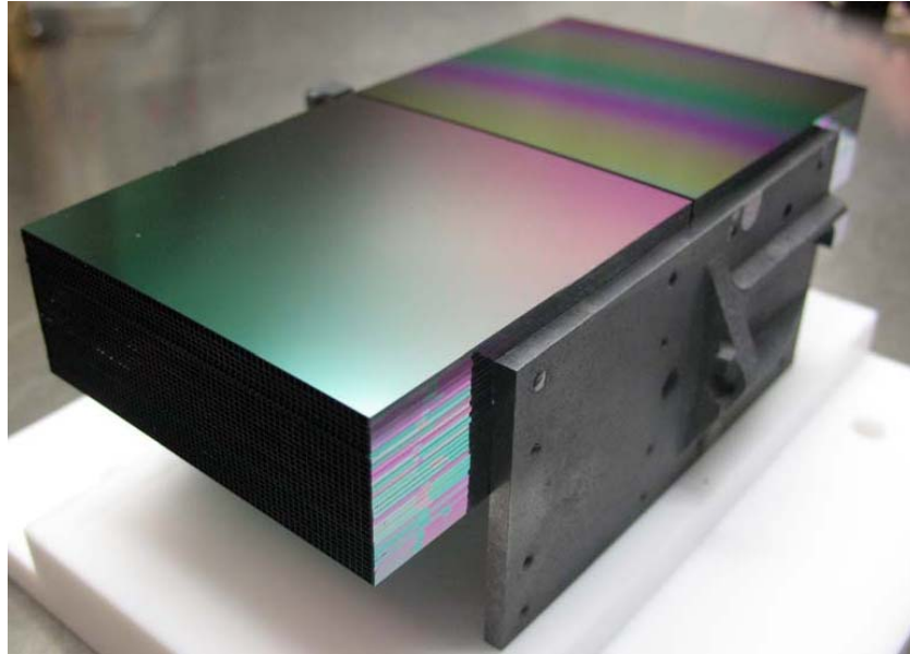
Figure 8 – Photograph of a recent Silicon Pore Optics mirror module. The two stacks (approximating the parabola and hyperbola mirror segments) are connected by the mounting bracket (courtesy of Cosine BV).
