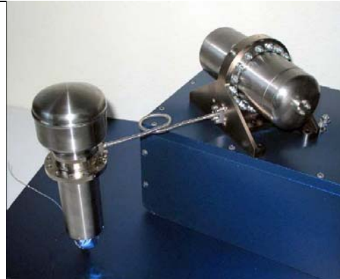
Large pulse tube cooler developed under ESA GSTP contract
