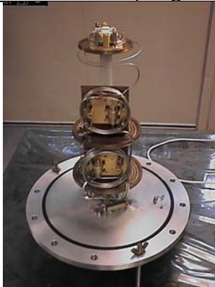
4He Joule Thompson sorption cooler developed for Planck program
