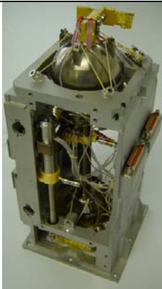
3He Sorption cooler developed for Herschel program
