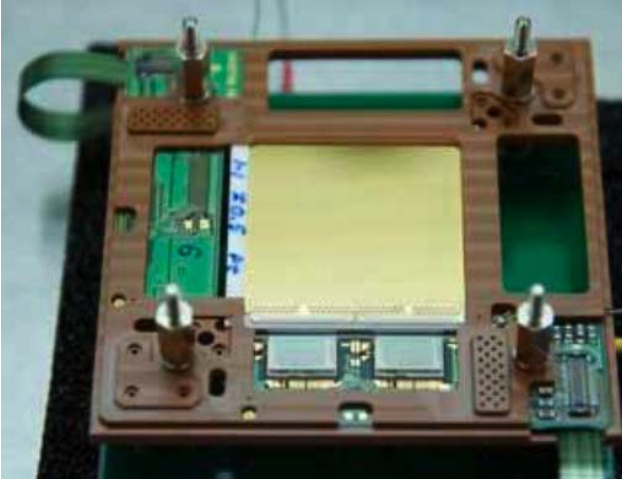
Figure 11: CdTe Strip detector, ASTRO-H heritage
