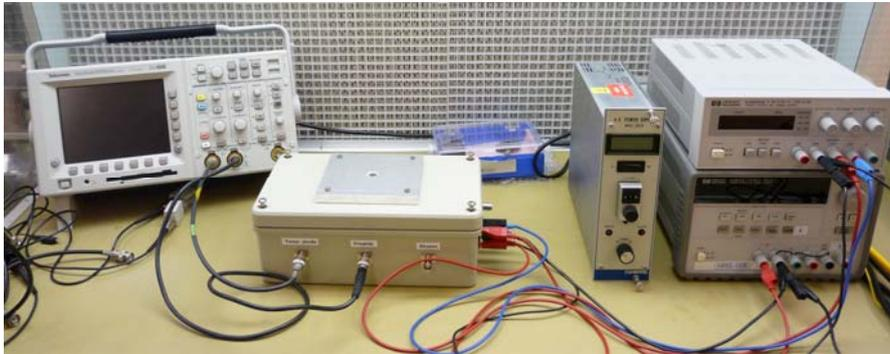
**Figure 5-5: SDD test bench set-up at CESR. It enables analog and digital readout of the SDD.**
