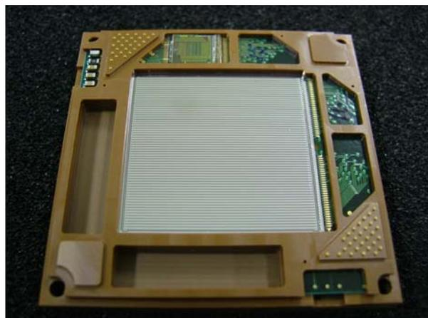
Figure 4-4. Photo of a DSSD prototype layer. The DSSD size is  $2.5 \times 2.5 \text{ cm}^2$ . The IXO-HXI will use DSSDs with a similar design, but with a larger area of  $3.5 \times 3.5 \text{ cm}^2$  (4 chips per layer) or larger.
