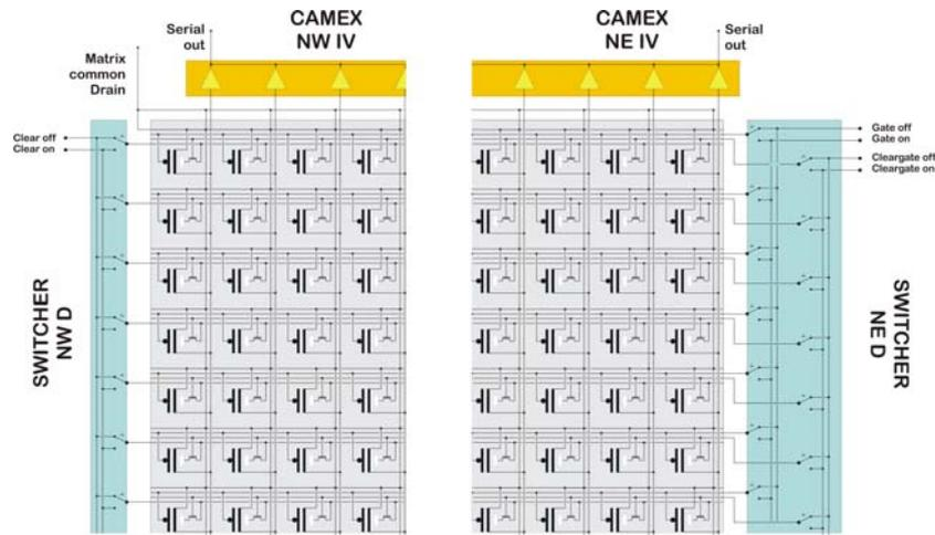
**Figure 2-9: Front end connection to the sensor. Each row of pixels requires 3 Switcher ports, and each column one CAMEX channel. The row connections are made to the respective SWITCHER devices at the left (Clear) and the right (Gate, Cleargate) respectively. A total number of 8 SWITCHER ICs is needed to operate one sensor hemisphere. The CAMEX IC has 128 channels, and every 64 channels are multiplexed to one serial readout node. This means 1 CAMEX and two readout nodes per sector.**
