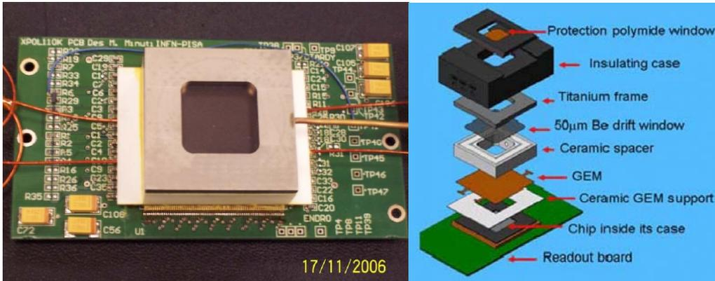
**Figure 6-3:** (Left) The sealed gas pixel detector currently working in laboratory. (Right) an exploded view. The window is 1.5 cm x 1.5 cm.
