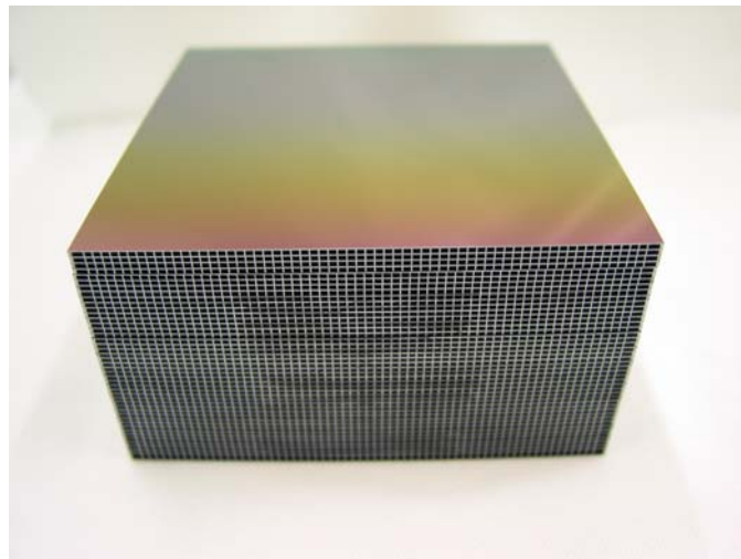
Figure 3: SPO mirror plate stack, consisting of 45 bonded mirror plates, as required for the IXO telescope baseline design.
