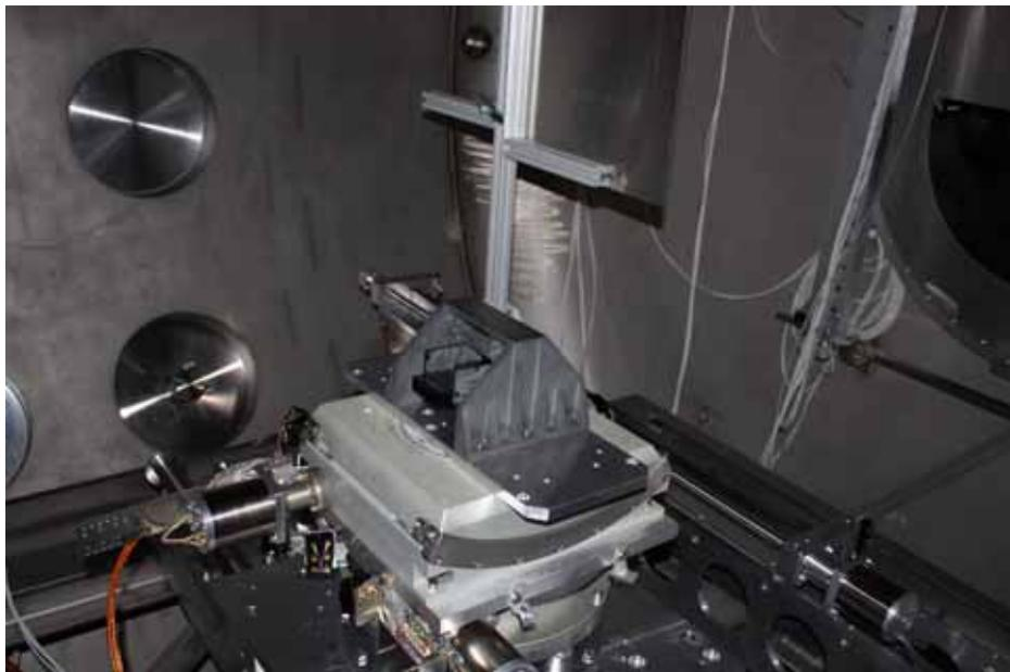
*Figure 25 A mirror module mounted inside the PANTER tank in flight representative configuration in the CEC.*
