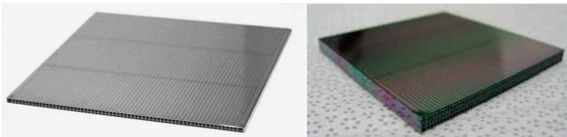
Figure 15 The first coated unwedged (left) and wedged (right) stacked Si pore optics. The contrast in the left picture has been manipulated to make it easier to distinguish the coated and the uncoated area (the dark lines).
