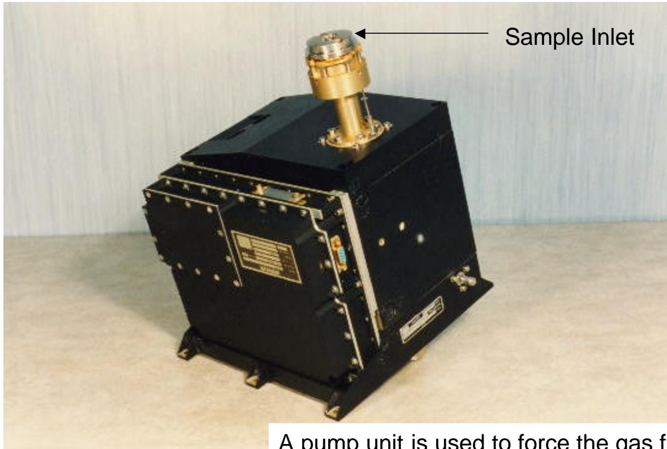
A pump unit is used to force the gas flow through a filter which has a thimble-like shape. In its sampling position, the filter front face extends a few mm beyond the probe fore dome, thus being at a temperature very close to the ambient Titan atmosphere
