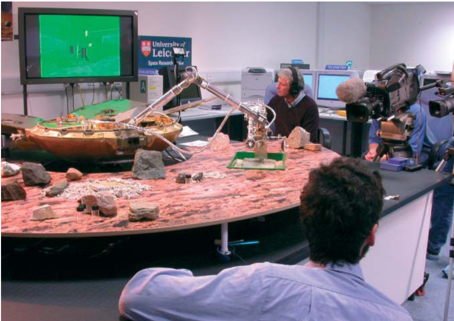
Fig. 16. Sampling operations at the Lander Operations Control Centre, Univ. Leicester (UK) during early December 2003. The lander Ground Test Model, equipped with the DM ARM, is deploying the QM PAW and performing a sampling operation with the Rock Corer Grinder. The sample itself, in this case a fissile shale, is seated in a bed of coarse sand and within the working zone of the PAW/ARM defined by the raised area. All Rights Reserved, Beagle 2
