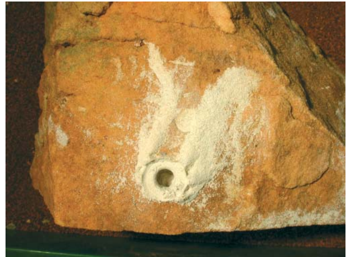
Fig 11. Upper left: the Rock Corer Grinder FM. Note the dual functionality and shape of the sampling tip. Right: results of coring into a field sample of quartzose sandstone with a case-hardened thin (~1 mm) weathering rind (Planetary Science Sample Library 146/274). Lower left: the RCG QM equipped with the Translation Table (TT) for transcribing the tool-head during grinding. The TT was not fitted to the FM following an engineering and scientific assessment on the effectiveness of the device. All Rights Reserved, Beagle 2
