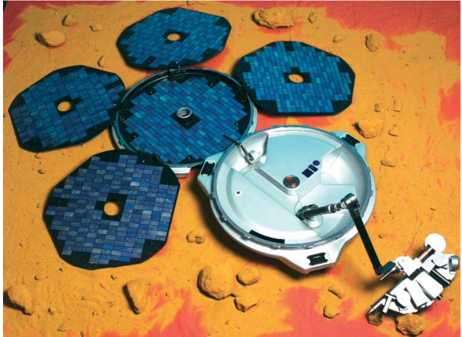
Fig. 1. A fully deployed model of the Beagle 2 lander showing the arrangement of solar arrays (four petals plus the lid). The base unit (diameter ~66 cm) accommodates GAP and the lander systems, including batteries and transceiver. The PAW is shown deployed and making contact with a sample under investigation. All Rights Reserved, Beagle 2
